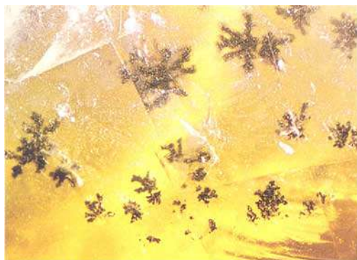
Fig. 18. A yellow opal from Tanzania is charmingly enlivened by numerous dendrites of manganese oxide , varying in size. Transmitted illumination. 25x.
