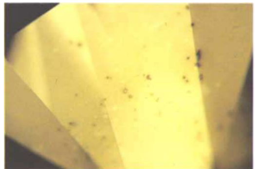
Fig. 15. The blotchy coloration on the pavilion facets of the radioactive diamond in Figure 11. Note also the intense green spots.
