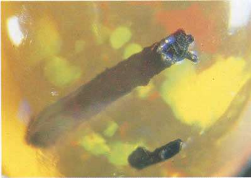
Fig. 14. A green-black hornblende crystal is covered with a crust of limonite . Note the thickness of the limonite layer at the top, near the fracture. Darkfield illumination. 34x.
