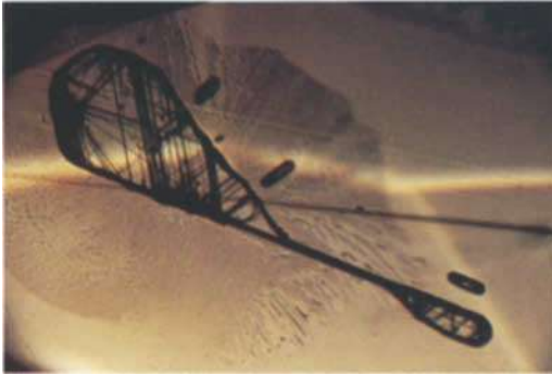
Fig. 4. This picture shows the moving of a vapour bubble nearer the trapping. Direct illumination, polarized light. 40x.
