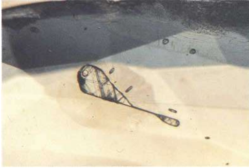
Fig. 2. The 'necked-down' three-phase inclusion. Within the cavity are seen the thin radiating needles, the gaseous phase and the small nuclei of crystallization. A fingerprint surrounds the three-phase inclusion. Direct illumination. 18x.
