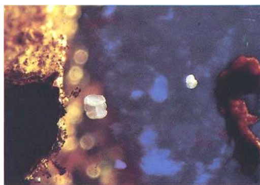
Fig. 9. Translucent white cristobalite inclusions in a Mexican opal, are suspended against a background of a deep blue/orange/red play of colour. Oblique illumination. 20x.
