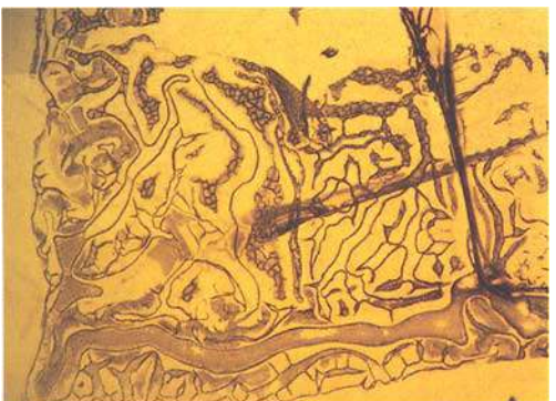
Fig. 22. An epigenetic pattern was produced when iron-rich fluids invaded the fracture in this Mexican opal and dried out. Transmitted light. 40x.
