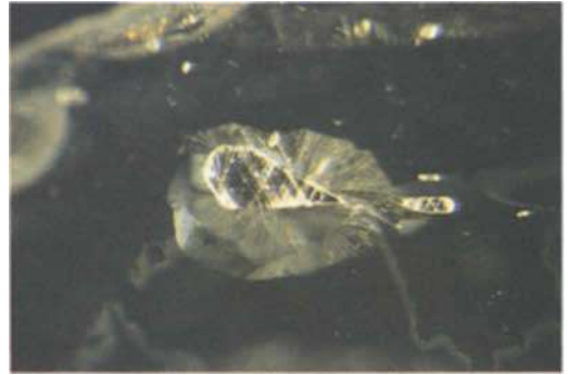
Fig. 3. The external fingerprint inclusion and the triangular or tetrahedral nuclei of crystallization show better. Reflected illumination. 20x.
