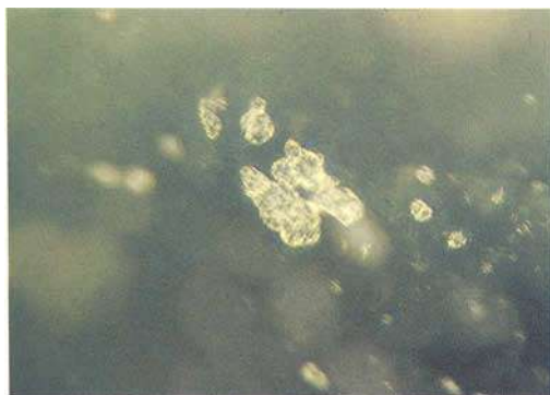
Fig. 8. Looking like glass, small aggregates of tiny plate-like cristobalite crystallites hover in a water opal from Querétaro, Mexico. Darkfield illumination. 150x.
