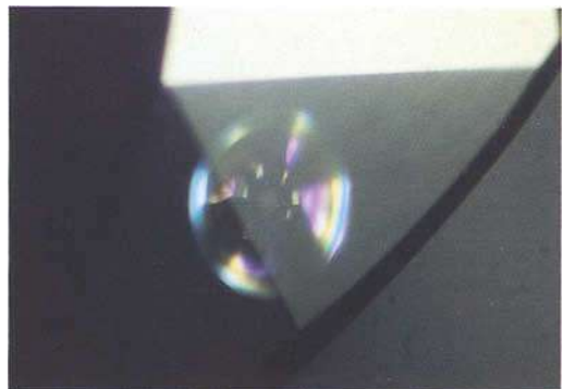
Fig. 13. Altered inclusion and tension halo in a heat treated sapphire, reflected light.
