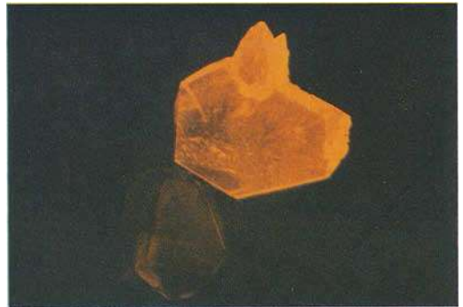
Fig. 7. A Knischka synthetic ruby (above) and a less intensely luminescing Ramaura synthetic ruby during the impact of electrons; for details see text.
