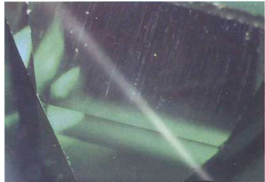
Fig. 22. Needle-like inclusions in the Kyocera synthetic emerald.
