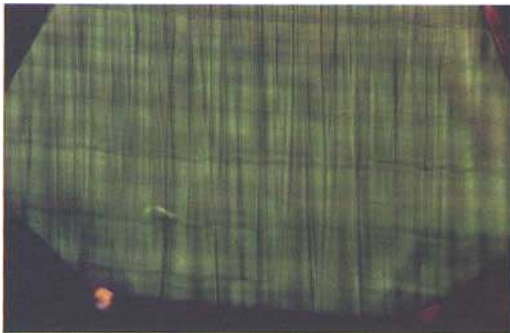
Fig. 10. Russian hydrothermally-grown synthetic emerald; faceted sample without residue of the seed, step-like growth lines and colour zoning, irregularly changing subgrain boundaries almost perpendicular to the colour zoning. Crossed polarizers. 40x.
