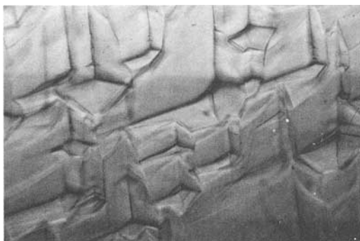
Fig. 13. Russian hydrothermally-grown synthetic emerald; block structure of subparallel orientated sub-individuals with curved surfaces. 30x.
