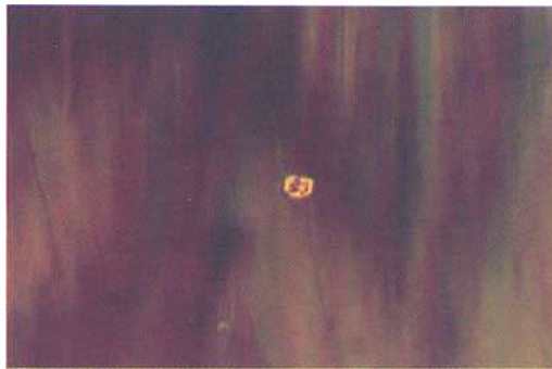
Fig. 20. Russian hydrothermally-grown synthetic emerald; inclusion of a double refractive crystal. Crossed polarizers. 100x.
