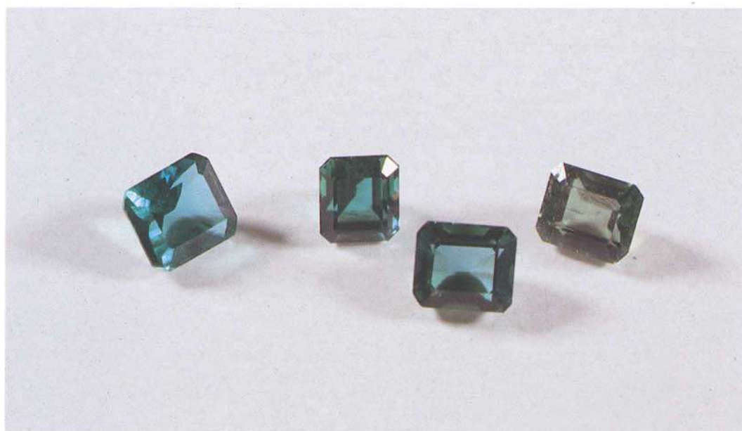
Fig. 1. Faceted Russian hydrothermally-grown synthetic emeralds. Size of samples approx. 4 \times 5 mm (Photo by O. Medenbach, Bochum, West Germany).
