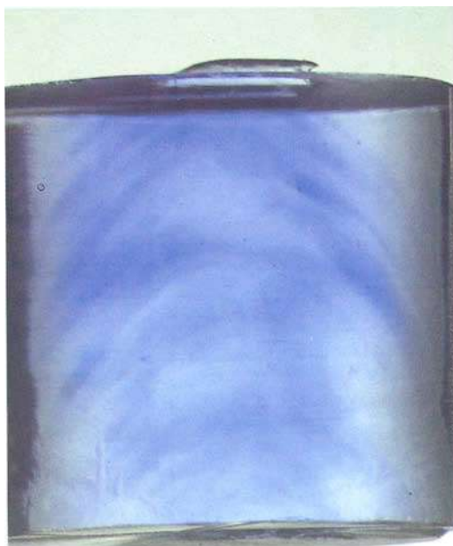
Fig. 29. Colour distribution in a Kyocera synthetic blue sapphire crystal.
