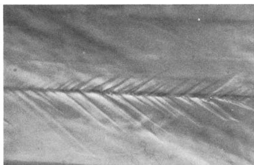
Fig. 16. Russian hydrothermally-grown synthetic emerald; angular growth pattern with the edge of a sub-individual as bisector of the angles. 50x.
