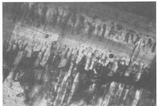
Fig. 7. 'Two phase' and other needle-like inclusions in the Lennix synthetic emerald.
