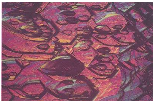
Fig. 3. Shield-shaped etch figures on a second order bypyramid of a Brazilian goshenite. Nomarski Differential Interference Contrast. 80x.
