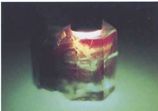
Fig. 23. Kyocera synthetic emerald glowing red in the light produced from an optical fibre light unit.
