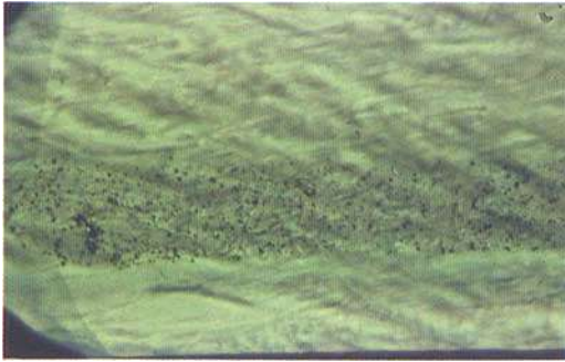
Fig. 18. Russian hydrothermally-grown synthetic emerald; opaque particles confined to the boundary colourless seed/synthetic emerald. View in a direction perpendicular to the boundary. 40x.
