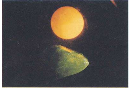
Fig. 10. The upper two cabochons of Figure 9 under the impact of electrons (10.5 kV at 1.0 mA); note orange-yellow CL-colour of the grossular against canary-green CL-colour of jadeite; dyed agate is non-luminescing.
