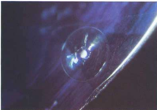
Fig. 12. Altered inclusion and tension halo in a heat treated sapphire, transmitted light.
