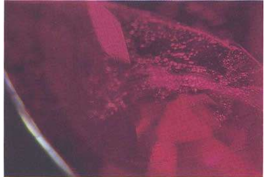
Fig. 10. Partially glass-filled feather in a natural ruby.
