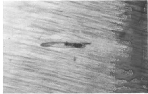
Fig. 22. Russian hydrothermally-grown synthetic emerald; three-phase inclusion, probably consisting of two immiscible liquids and one gaseous phase. 100x.
