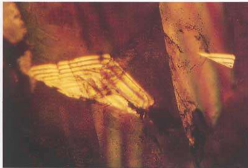
Fig. 3. Natural sapphire from Sri Lanka; inserted bodies of corundum revealing plane boundaries between dominant and subordinate individuals. Crossed polarizers. 30x.
