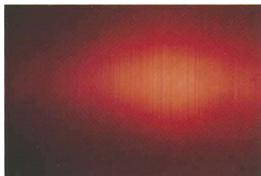
Fig. 3. The very slightly undulating growth-colour zones, shown here in shadowed transmitted light, are the single most important diagnostic feature of Kyocera's new product 30x.
