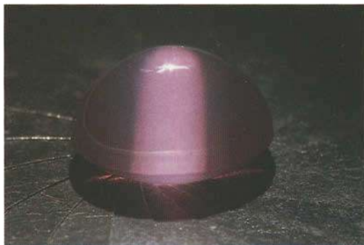
Fig. 2. The typical conical-shaped milky light transmission effect shown by the Inamori alexandrite cat's-eyes.
