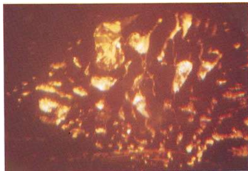
Fig. 2. Bizarre-shaped cavities, partly filled with solid substance. Reflected light. 20x.
