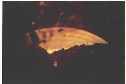
Fig. 4. Natural sapphire from Sri Lanka; inserted body of corundum [below] confined to an intercalated lamella on the positive rhombohedron r(10\bar{1}1) [above] as boundary between dominant and subordinate individuals. View almost perpendicular to the intercalated lamella, crossed polarizers. 20x.
