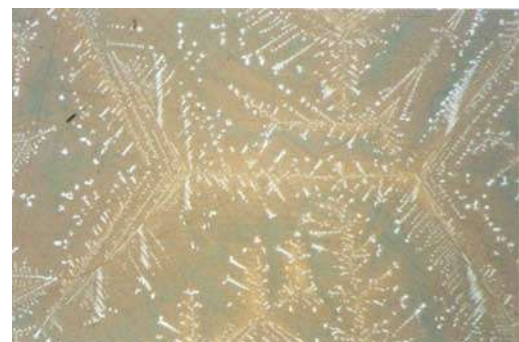
Fig. 5. Polished section of glass shown in Figure 2; shows skeletal crystals of cuprous oxide; field of view 0.6mm across.
