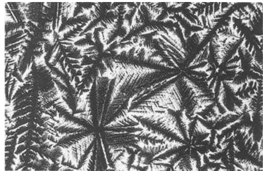
Fig. 4. Thin section (30 μm) of glass shown in Figure 2; shows skeletal crystals of cuprous oxide in plane polarized light; field of view 4mm across.
