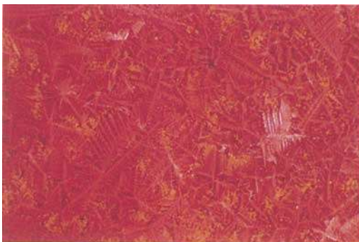
Fig. 3. Crystals in red glass showing skeletal structure. Photo by E.A. Jobbins.
