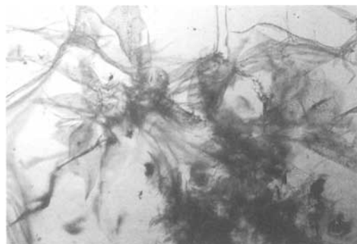
Fig. 2. Wispy or veil-like patterns of residual flux in yellowish-green Gilson synthetic emerald. 25\times
