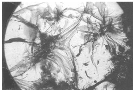
Fig. 1. Wispy or veil-like patterns of residual flux in yellowish-green Gilson synthetic emerald. 32\times
