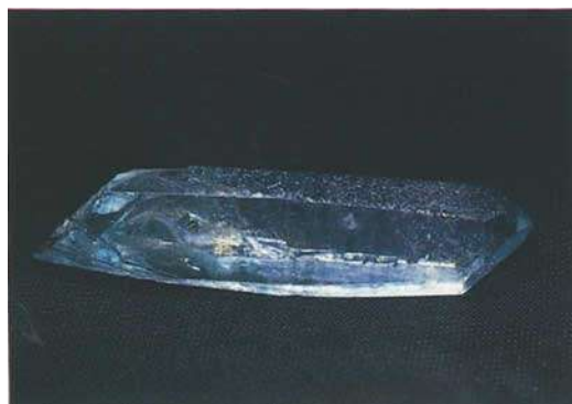
Figs. 1a & b. 'Aqua Aura' coated quartz crystal (GIA Collection No.16667) showing (left) the blue colour (right) the iridescent colours provided by the coating. Oblique fibre optic illumination. Photos by William Videto.
