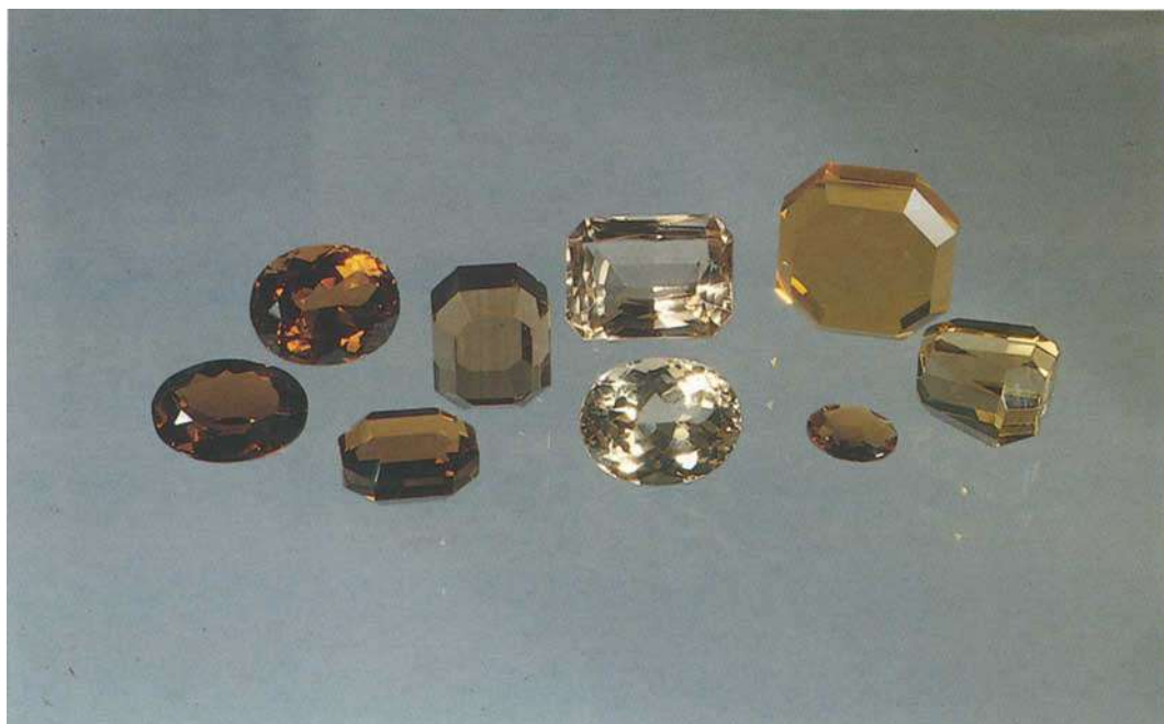
Fig. 24. Colour sequence of synthetic citrines: sample 1: type 1, produced in USSR; sample 2: type 4, produced in Japan; sample 3: type 4, produced in Japan; sample 4: type 3, produced in USSR; sample 5: type 3, produced in USSR; sample 6: type 4, produced in Japan (heat-treated); sample 7: type 6, produced in USA; sample 8: type 3, produced in Japan; sample 9: type 6, produced in USSR. Size of sample 2 approx. 11 \times 14 mm. Photo by O. Medenbach, Bochum, FRG.
