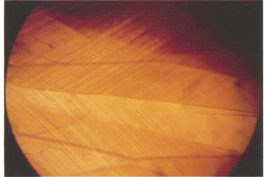
Fig. 15. Natural citrine (heat-treated natural amethyst) from Brazil; families of straight parallel growth planes parallel to the major rhombohedron r \{1011\} and parallel to the minor rhombohedron z \{0111\} forming an angle of 76^\circ , different colour intensities are observable in the growth sector confined to r (dark orange-brown) and the growth sector confined to z (light orange-brown). 26x.
