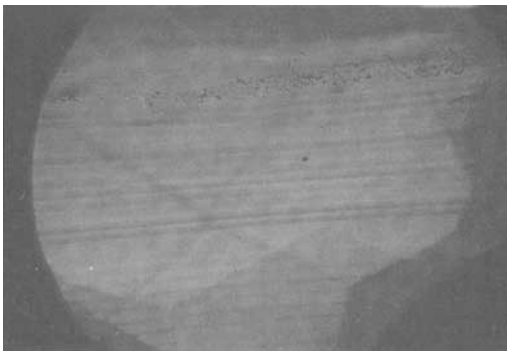
Fig. 34. Synthetic citrine of type 3 produced in USSR; growth planes parallel to the basal pinacoid. 22x.
