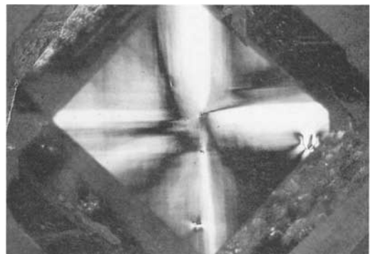
Fig. 8. The De Beers synthetic diamond of Figure 6 between crossed polarized light.
