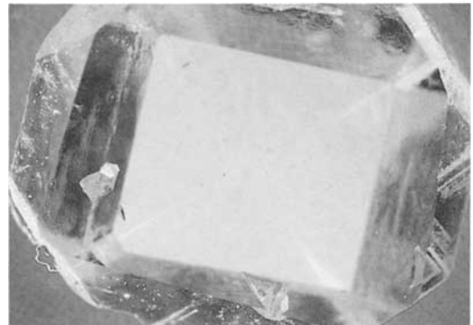
Fig. 6. A colourless cross formation in an uncut De Beers synthetic diamond.
