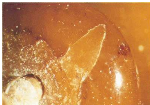
Fig. 13. A coated amber bead showing an area where the coating has come away.
