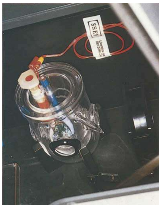
Fig. 5. The Dresden Green mounted in the \text{N}_2 vapour atmosphere of the highly transparent cooling cell and adjusted in the sample beam of the Pye Unicam SP8-100 UV/VIS spectrophotometer prior to the first absorption measurement in refrigeration.
