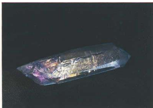
Figs. 1a & b. 'Aqua Aura' coated quartz crystal (GIA Collection No.16667) showing (left) the blue colour (right) the iridescent colours provided by the coating. Oblique fibre optic illumination. Photos by William Videto.
