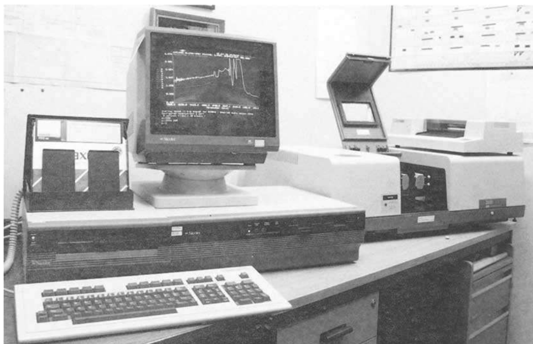
Fig. 1. Nicolet model 510 FT-IR spectrometer with 620 work station, plotter and added 8" floppy drive in use at the Gem Testing Laboratory of Great Britain.
