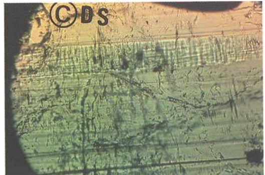
Fig. 19. Typical growth striae (growth layers) with internal structure. 50x
