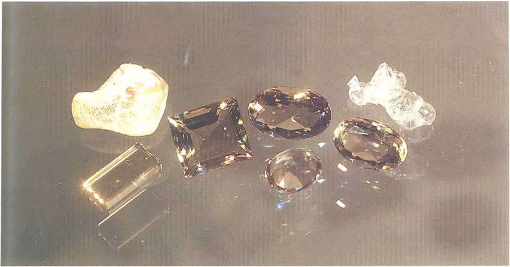
Fig. 1. A number of specimens of natural iridescent glass from Mexico. Rear left: natural untreated material; rear right: a frothy specimen of the glass after heating to 1200°C. The largest of the faceted stones weighs 3.2ct.
