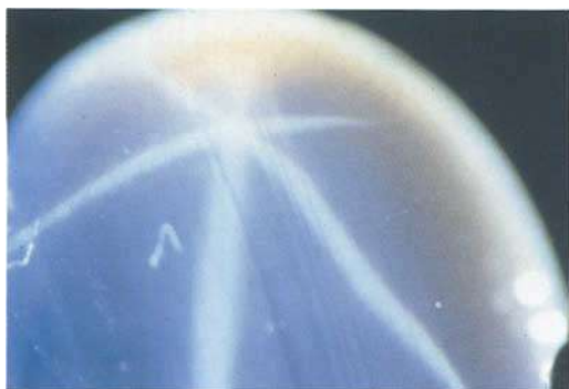
Fig. 3. Dark brownish-blue cabochon-cut star sapphire from Kenya. The hue is related to the presence of hematite needles; the parallel striae are ascribed to a lamellar twinning structure. 8x.
