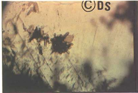
Fig. 11. Protogenetic mica crystals showing irregular outlines. 35x
