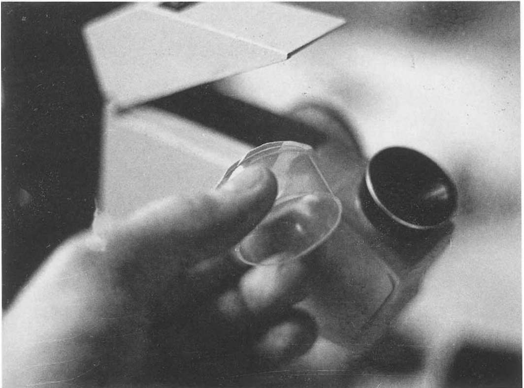
Fig. 3. Pill-box 'cover' for Dialdex eyepiece; open side in view, lenses on the other side away from view.
