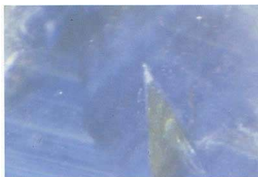
Fig. 4. The straight-edged blue colour bands show the hexagonal sapphire symmetry and are referred to both multiple growth episodes and contemporary changes in the chemical environment. Fluid 'feather' and haloes of iron compounds create a characteristic microscopic appearance of these star-sapphires. 20x.
