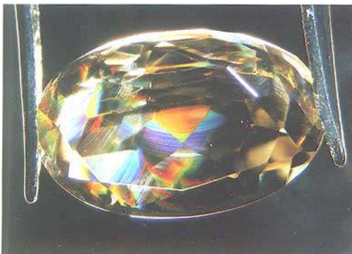
Fig. 2. Iridescent glass with botryoidal form, exhibiting spectral colours due to interference on thin layers.
