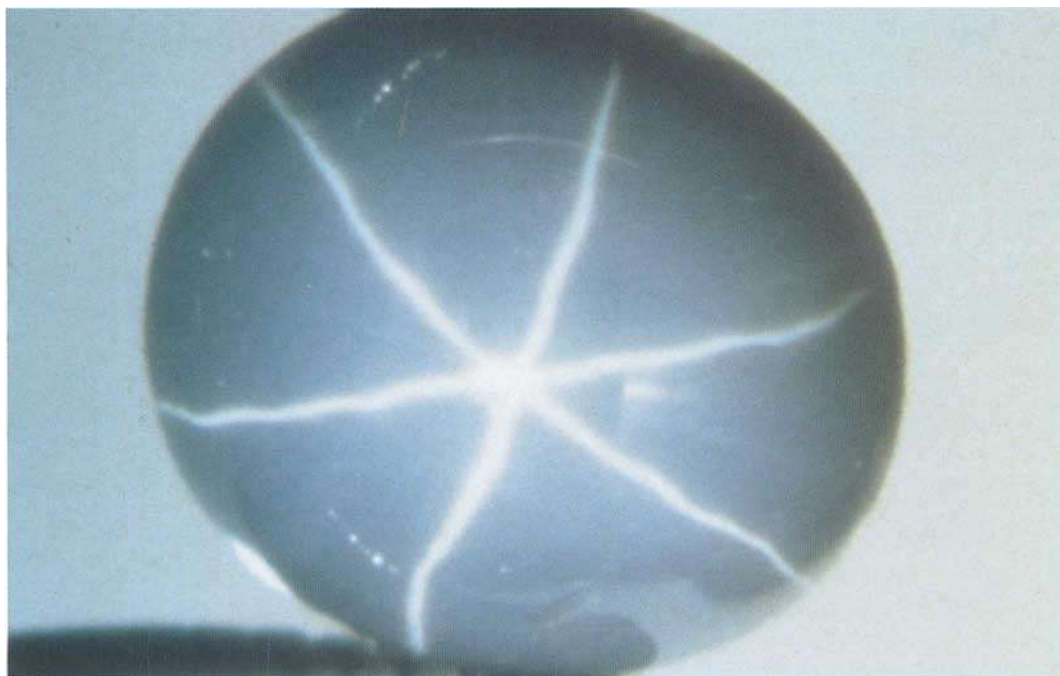
Fig. 2. A blue cabochon-cut star sapphire from Kenya displays a six equally rayed asterism. The hexagonally orientated acicular inclusions engender the six equally spaced narrow rays of same length and brightness, very sharp edged. The star effect in these gems is identical to that seen in the synthetic Linde sapphires. 10x.
