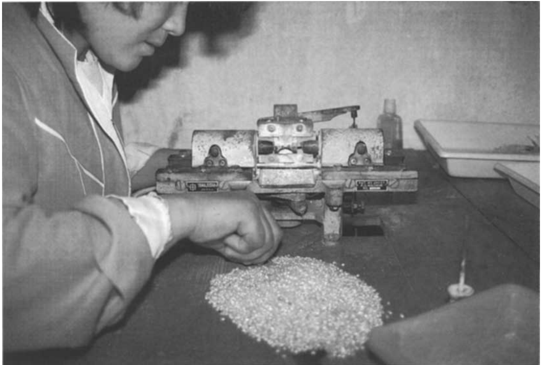
Fig. 13. Drilling small non-nucleated baroque cultured pearls with a double-ended drilling machine, Yangxin, China.
