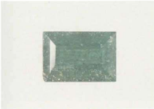
Fig. 1. Faceted hydrothermally-grown Lechleitner fully synthetic emerald (sample 2). Size of the stone approx. 6.4 \times 4.3 mm. (Photo by O. Medenbach, Bochum, West Germany)
