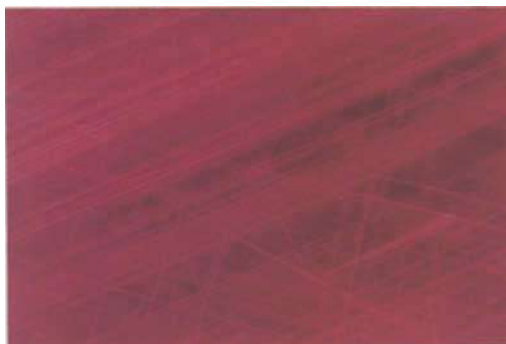
Fig. 3. Very fine acicular crystals of rutile pictured here are the cause of the asterism in this Tanzanian star rhodolite. 40x.
