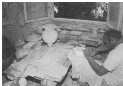
Fig. 1. Carving translucent alabaster (gypsum) in a small workshop in Volterra, Italy.
