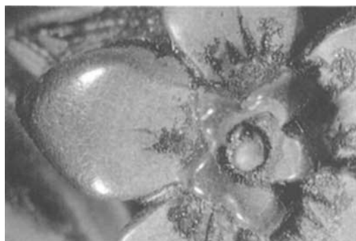
Fig. 5. Uncoated, crazed surface of the gutta-percha brooch shown in Figure 1.
