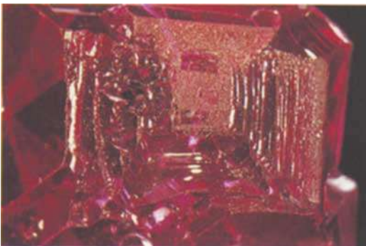
Fig. 3. The truncated surface that appears to be the point of attachment or growth-nucleation of the synthetic spinel. Magnified 5 \times . Photomicrograph by John I. Koivula.
