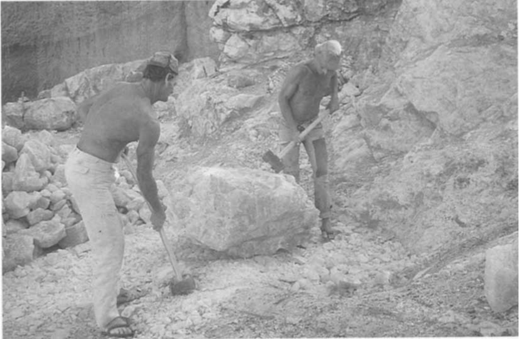
Fig. 8. Lavra do Bianor (Minas Gerais). Sorting massive rose quartz using a sledge-hammer.
