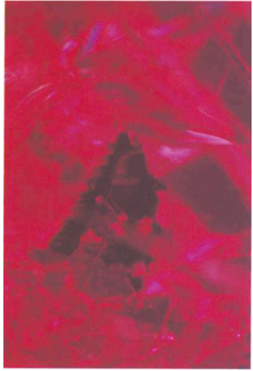
Fig. 2. Primary flux inclusions in the synthetic spinel crystal. Magnified 20 \times . Photomicrograph by John I. Koivula.
