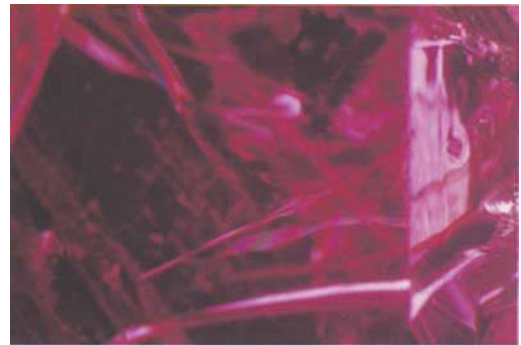
Fig. 4. Brightly reflective and iridescent air-filled fractures resulting from strain as observed in the synthetic spinel. Magnified 10 \times . Photomicrograph by John I. Koivula.
