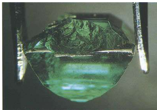
Fig. 25 Extensive irregular breakage caused by the strong unilateral pressure of a diamond bagueette on this emerald, formerly a centre stone in a ring. Development of breakage from the point of contact (the asymmetric indentation below the girdle) over the entire left crown side of this Colombian emerald, free from cracks and poor in inclusions. Length of the notch approximately 2.65 mm.
