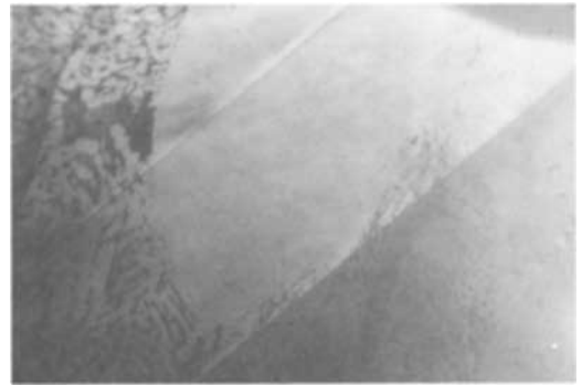
Fig. 60. Twinning in flux-grown Chatham synthetic sapphire; intercalated lamellae of corundum in twin position on r(10\bar{1}1) . View 32.4^\circ inclined to the c -axis. 40x.
