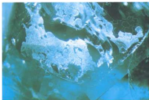
Fig. 23 Covering of oil, fat or Canada balsam on an extended tension crack in a Colombian emerald, transformed into a semi-solid, ugly-looking white crust. Width of photomicrograph about 0.40 mm.
