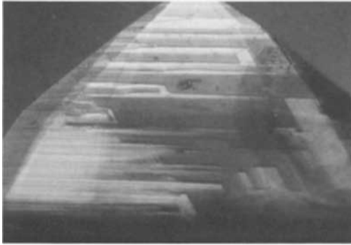
Fig. 50. Growth structures in natural sapphire from Pailin, Cambodia; planes parallel to c (0001) and r (1011). View perpendicular to the c -axis, the c -axis runs vertically. 25x.
