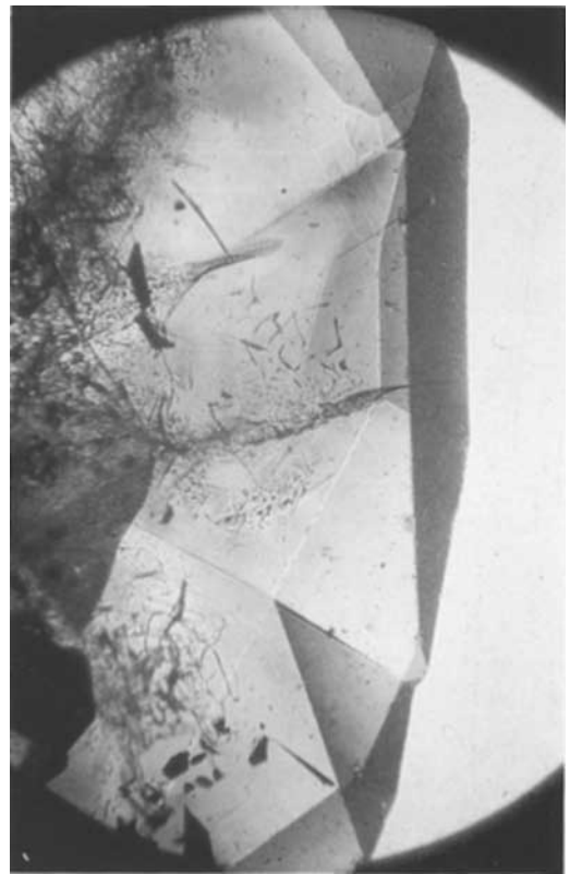
Fig. 59. Growth structures and twinning in flux-grown Chatham synthetic sapphire; repeated twinning across \{10\bar{1}0\} with two composition planes a and a' \{11\bar{2}0\} observable. View parallel to the c -axis. 24\times .
