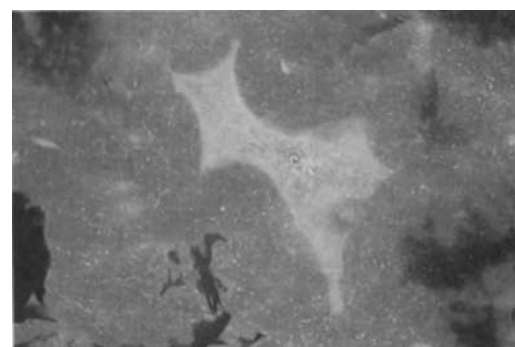
Fig. 7. The typical agate structure was detected in some areas of the agate base. Photomicrograph by John I. Koivula. Magnified 30x.
