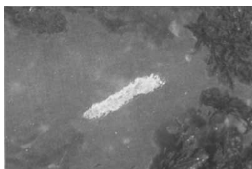
Fig. 5. A scratch can be seen in the colourless coating on the base of the assembled agate. Photomicrograph by John I. Koivula. Magnified 10x.
