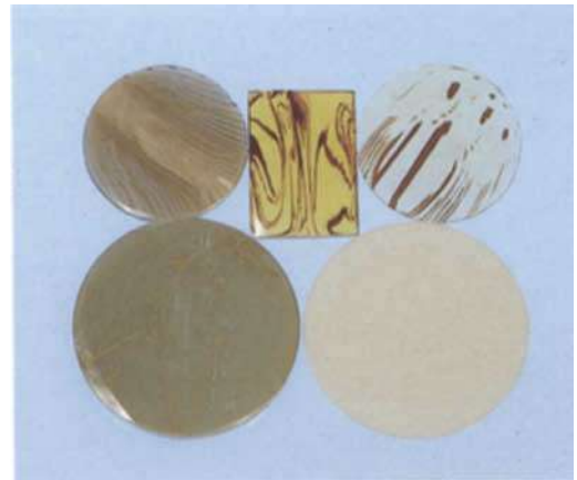
Fig. 14. The structures seen in the cast polyester resin imitations of: top row, left to right – horn and tortoise-shell (2), bottom row – 'onyx marble' and ivory. (Photo E.A. Jobbins)
