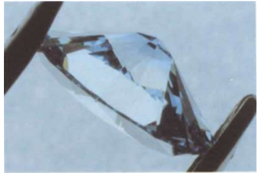
Fig. 7. Side view of the treated blue diamond showing the lack of colour in the body of the stone. (Photo Jobbins/Scarratt)
