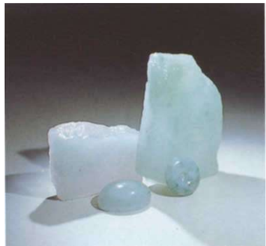
Fig. 10. Resin impregnated jadeite or 'B-Jade'. The disc on the right weighing 1.56ct and the cabochon on the left weighing 5.65ct. (Photo K. Scarratt)
