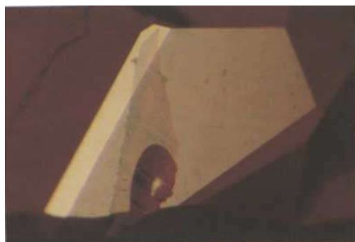
Fig. 6. A facet of a heat and glass treated ruby. A cavity (and all open fractures) have been filled with glass, identifiable by its lower lustre compared with corundum. Within the glass part an air bubble is cut by the surface. Magnification 20x.
