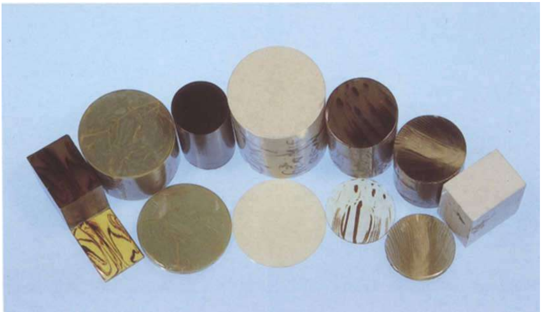
Fig. 13. The 'varieties' produced in cast polyester resin to imitate (rods, from left to right) tortoise-shell, 'onyx marble', jet, ivory, tortoise-shell, horn and bone. (Photo E.A. Jobbins)
