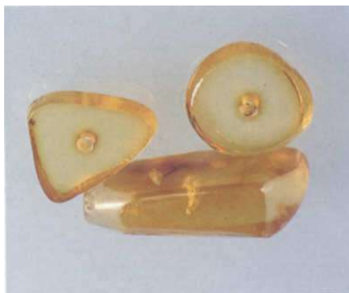
Fig. 28 Examples of surface enhanced amber showing the deep yellow exterior contrasting with the colourless to near-colourless interior. Each specimen has been specially sectioned and polished to display the effect of the treatment. (Photo K. Scarratt)
