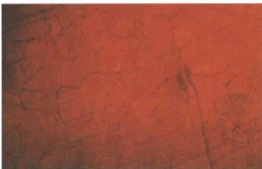
Fig. 4. The cracked or 'dried mud' structure - also referred to as the 'honeycomb' appearance - of the Opalite is seen here when examined in transmitted light down the length of the columnar structure. 20x. Photo by John I. Koivula.
