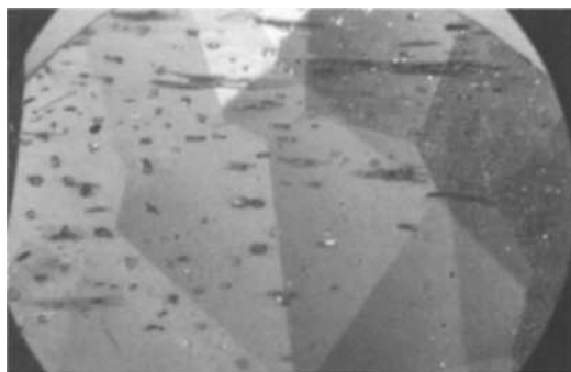
Fig. 2. Inclusions in musgravite, first stone, transmitted polarized light (50x).
