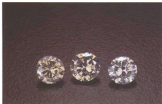
Fig. 3. The vast majority of 'white' or 'opalescent' diamonds, such as these three round brilliant-cuts from the Panna mine in India ranging from 0.30 to 0.33 ct, are also H-rich diamonds. Stones courtesy Malhotra Inc., New York. Photo by R. Weldon
