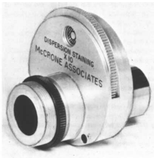
Fig. 3. The McCrone dispersion staining microscope objective.
