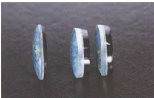
Fig. 11. When examined from the side, the two Opalite mosaic triplets on the right are seen to have thicker colourless caps than does the typical natural opal mosaic triplet, as illustrated by the one assemblage on the left. Photo by Maha DeMaggio.
