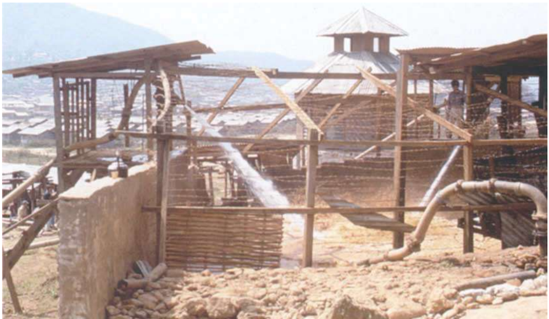
Fig. 18. Central Washing Plant. From platforms on either side of a pen, water cannons are used to wash the gravels brought to the facility for processing. Photo by R.C. Kammerling
