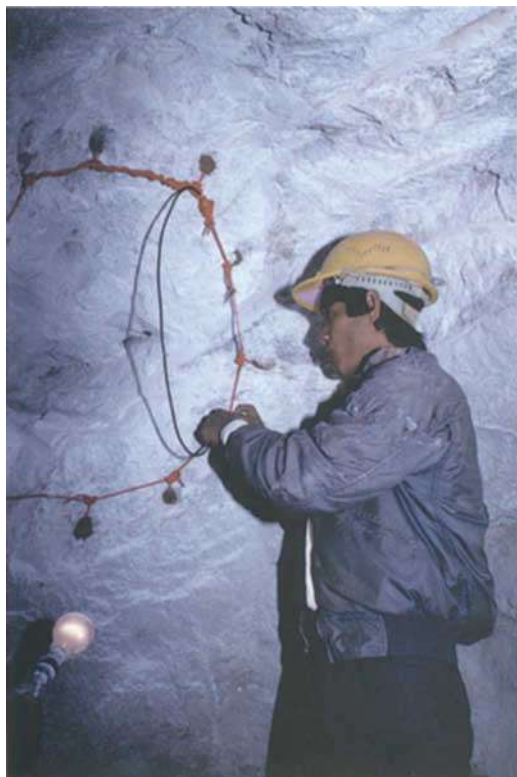
Fig. 12. Miner preparing for blasting in the 'hard-rock' mine at Thurein Taung. Photo by R.E. Kane
