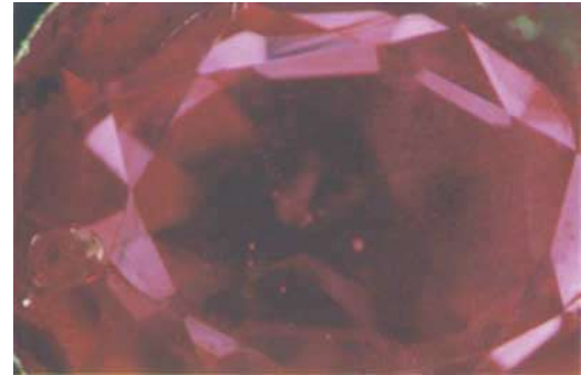
Fig. 32. Fine 'silk' of rutile needles and a corroded yellowish apatite in a Mogok ruby. 20x. Photomicrograph by E.J. Gübelin
