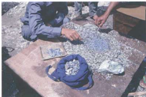
Fig. 13. Sorting sapphire at the primary tunnel mine at Thurein Taung. The blue sapphire is visible in matrix (bottom right) and in the concentrate (centre). Photo by E.A. Jobbins
