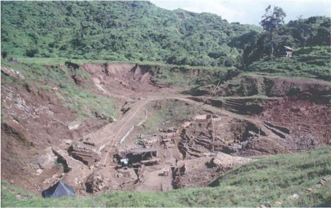
Fig. 8. The large open-pit mine at Yadanar Kaday-kadar in October 1992. The 'byon' (gem gravel) is being washed down by the water jet (upper left); the gravel is concentrated in the sluices or 'hymadwin' (centre); the vertical drainage shaft is capped by the black 'tent' (bottom left); see text. Photo by E.A. Jobbins
