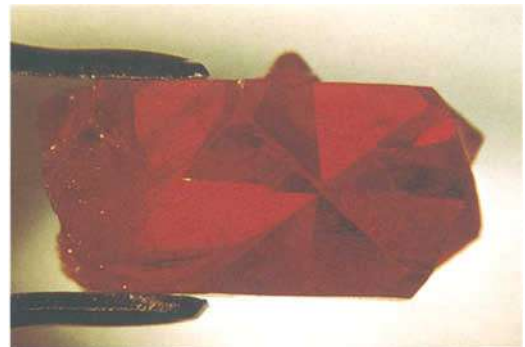
Figs 3, 4. Penetration twin viewed in a direction perpendicular to the c -axis: the two figures are related by a small rotation about the c -axis, 18x.
