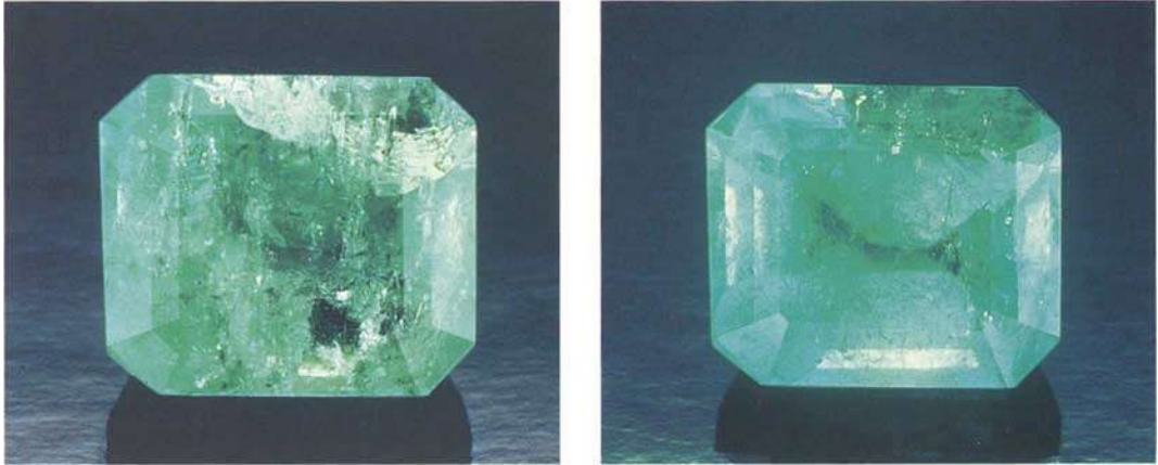
Fig. 1. Opticon filled emerald: 5.71ct. Before treatment. After treatment. Reproduced from the article of Reference 2, with the kind permission of the Editor of Gems and Gemology . © Gemological Institute of America and Tino Hammid.
