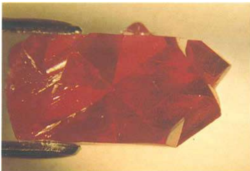
Figs 3, 4. Penetration twin viewed in a direction perpendicular to the c -axis: the two figures are related by a small rotation about the c -axis, 18x.
