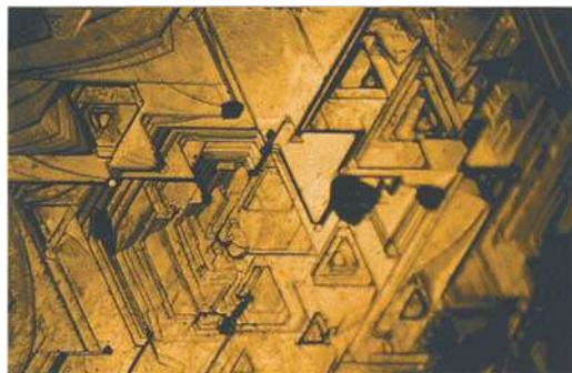
Fig. 9: A twin boundary extends from the lower right to the upper middle of the photograph, 30x.
