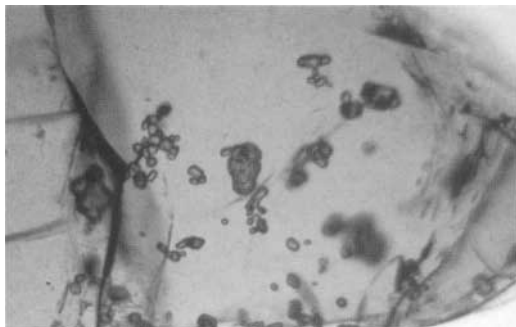
Fig. 6. Mineral inclusions with a strongly corroded surface in Ghatpara hessonite. Immersion, 20x. (Photo M. Redmann)
