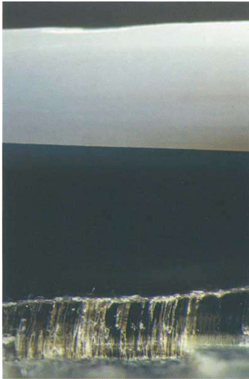
Fig. 2. Cross-section through the shell of the saltwater oyster Pinctada margaritifera (Tahiti). The components from the bottom to the top are: prismatic layer (calcite), mother-of-pearl layer (black-and-white, aragonite). 27x
