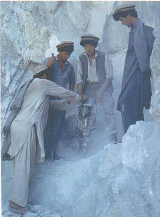
Fig. 3. Afghan miners drilling the limestone for rubies at Jagdalek, Afghanistan. (Photo by Gary Bowersox)
