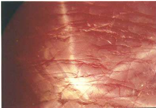
Fig. 3. Growth zoning and concentration of red dye in fissures of treated natural star corundum; the figure represents an area of about 0.4 x 0.6mm.
