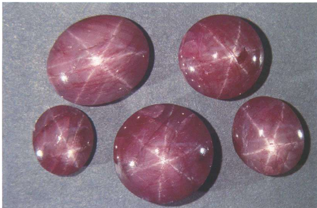
Fig. 1. Dyed natural star corundums; the middle cabochon in the front measures 11.4mm in diameter. (Photo by H.A. Hänni, Basel)
