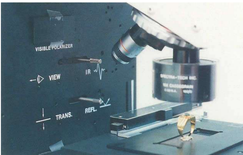
Fig. 2. The sample stage of the infrared microscope and the jewellery stuck to the sample board with plasticine. The visible light objective lens is used to find and focus a sample and the infrared light objective is used to measure the spectrum.
