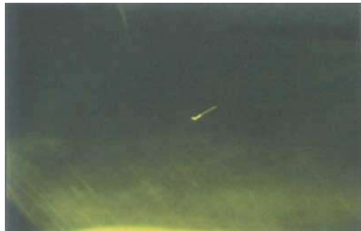
Fig. 5. The minute nail-head inclusion seen in one of the synthetic emeralds.
