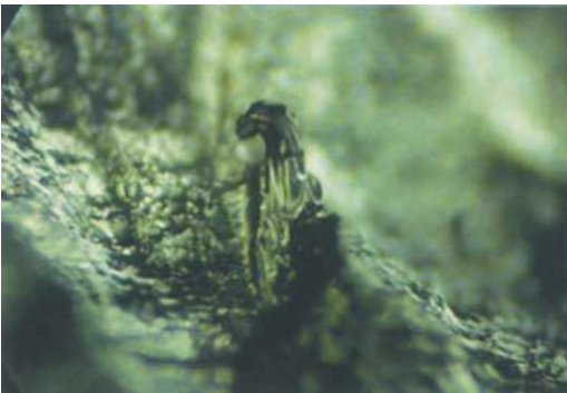
Fig. 8. Hook-shaped lechatelierite occlusion on the surface of a moldavite. Dark field illumination, magnified 30x. Photo: A. de Goutière.
