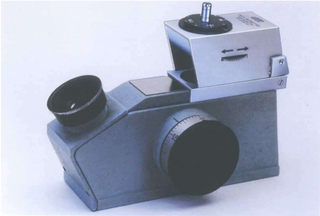
Fig. 2. The declinometer is fitted on a Rayner refractometer by means of an additional base-piece.
