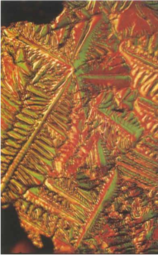
Fig. 1 (a). Differential interference photomicrographs of coralloid dendritic pattern commonly observed on a synthetic diamond face \{111\} (above) and \{100\} (left); the hopper nature of the face, growth steps, and surface dendritic pattern are seen.
