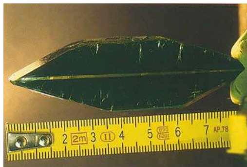
Fig. 1. The 39g rough of Russian hydrothermally-grown synthetic emerald, displaying the colourless beryl seed in the middle.
