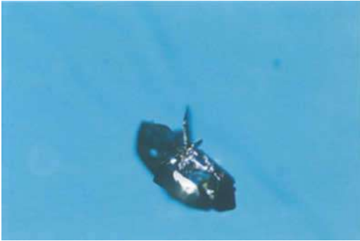
Fig. 7. Inclusion of an aggregate of black, opaque, lamellar metallic crystals. 400x.
