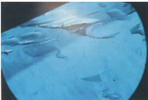
Fig. 16. Flat negative crystals having a shape very similar to that of the growth-figures seen on the surface of the emerald rough. 60x.
