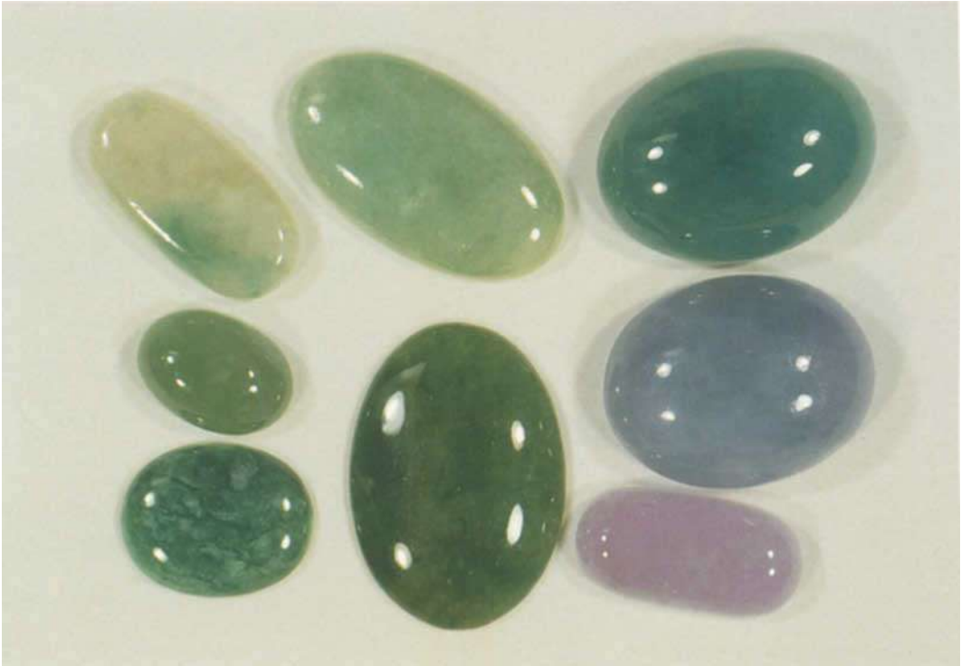
Fig. 1. Multi-coloured jadeites from Burma. The colour of the emerald-green jadeite, caused by chromium, can also be influenced by iron or nickel. The colour of the blue jadeite is probably due to its high content of titanium and iron. In the mauve jadeite cobalt and manganese may be acting as colouring agents.
