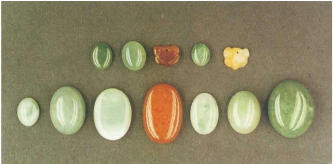
Fig. 2. Five pieces of natural wax polished jadeite, numbered 5 to 9 (upper row, from left to right). Seven pieces of bleached wax- or polymer-impregnated jadeite, numbered 10 to 16 (lower row, from left to right)
