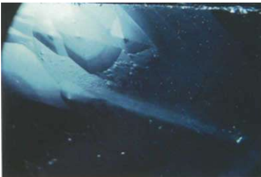
Fig. 3. Shield-shaped growth-figures on a surface of the 39g Russian synthetic emerald rough. 20x.
