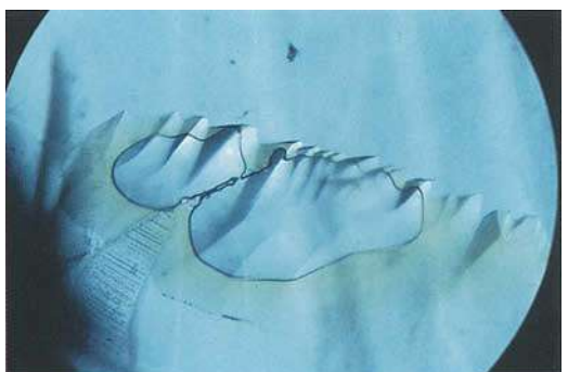
Fig. 17. This negative crystal hosts a two-phase inclusion. 100x.
