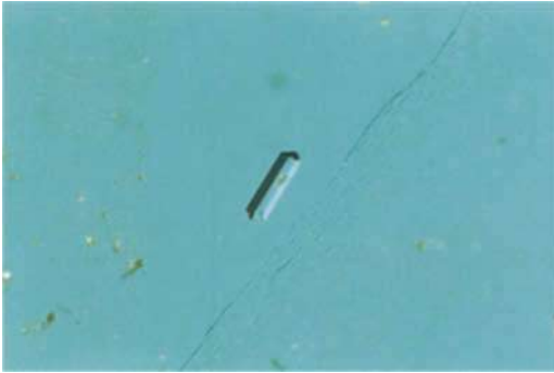
Fig. 14. Isolated phenakite crystal: around it many reflecting metallic inclusions are visible. 400x.
