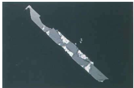
Fig. 10. Secondary electron-image of a polished section of a synthetic emerald: an opaque metallic crystal with strongly reflecting zones is visible.
