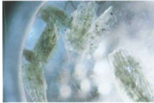
Fig. 9. Fragments of greenish tremolite from the Mong Hsu ruby mine. The green is due to Cr- and V-concentrations in the tremolite (see Table I for these and F content). Transmitted light. Length of crystal is 2 mm (Crystals immersed in epoxy, polished on one side).
