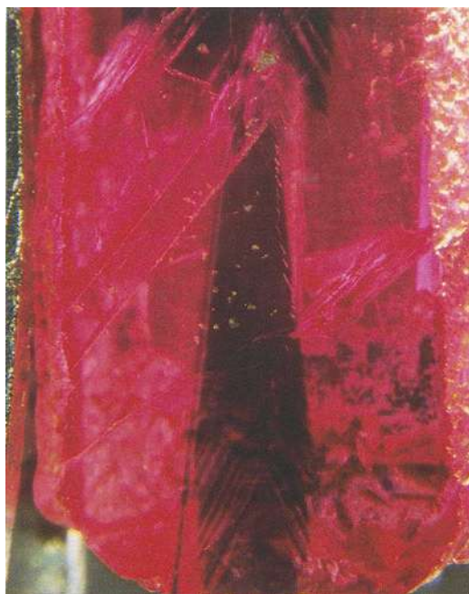
Fig. 4a. Typical colour zoning in a Mong Hsu ruby which has not been subjected to heat-treatment. Central violet to black zones are correlated with high concentrations of titanium and chromium (Peretti et al. , 1995a). Ruby cut parallel to the c -axis. Magnification on slide is 40x. Ruby approx. 2 ct. Photo by Dr E. Gübelin
