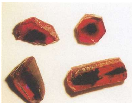
Fig. 3. Non-heat-treated Mong Hsu rubies, partly with polished facets, showing black to violet cores. Rubies between 0.50 and 2.00 ct.
