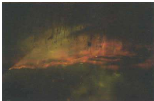
Fig. 4. The distinct orange colour seen in the fractures of a resin-treated emerald.
