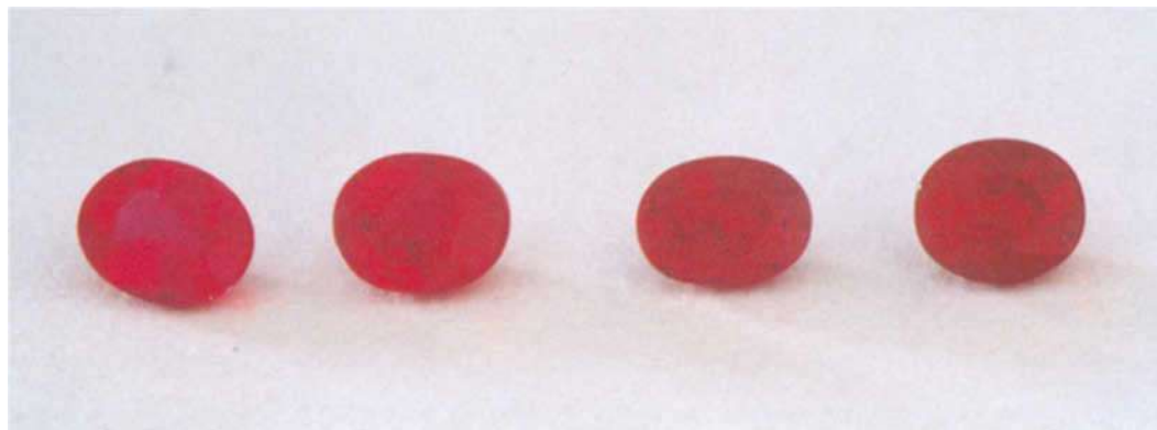
Fig. 6. A set of cut stones showing different colour shades obtainable from Mong Hsu rubies after heat-treatment. Rubies heat-treated and cut by the authors. Sizes of rubies around 1 carat each. Photo by Mouawad, Bangkok (Thailand).
