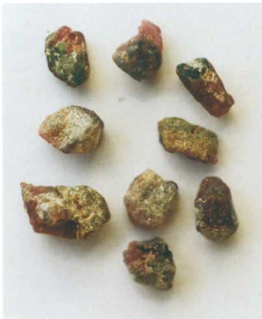
Fig. 13. Mong Hsu rubies intergrown with fuchsite (top three crystals) and light green Mg-chlorite and white mica. Crystal length of lower left ruby is 9 mm (identified by means of XRD and SEM-EDS, see Peretti et al. , 1995a).
