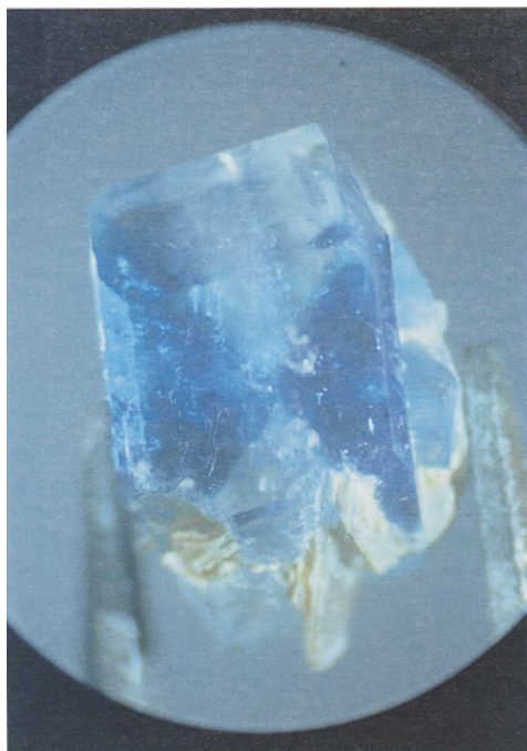
212 Figure 5: Euclase crystal with mica 'booklet' projecting from base and showing 'hour glass' colour distribution. Photo: S.M. Stocklmayer
