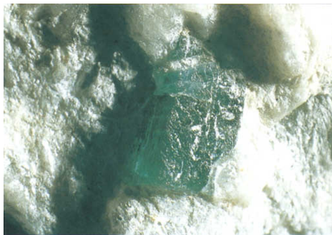
Figure 2: Carbonate vein sample showing an emerald crystal from Campos Verdes. The length of the crystal is about 25 mm.
