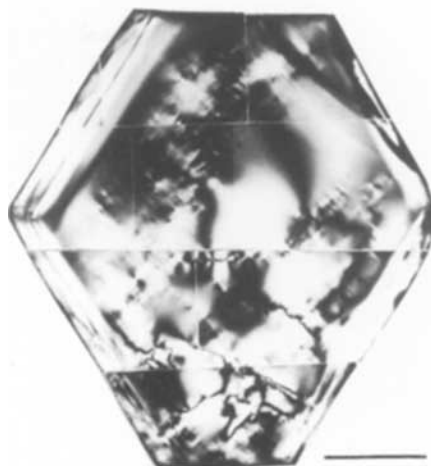
Figure 5: An example of commonly observed optical anomalies, most of which are associated with dislocations. Section perpendicular to c -axis. Crossed polarizers. Sample No. 8, Heffernan's mine, Australia. Bar 1 mm.
