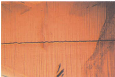
Figure 4: Subgrain boundaries, variably oriented in detail, almost perpendicular to the step-like growth structure. Immersion, magnified 30x.
