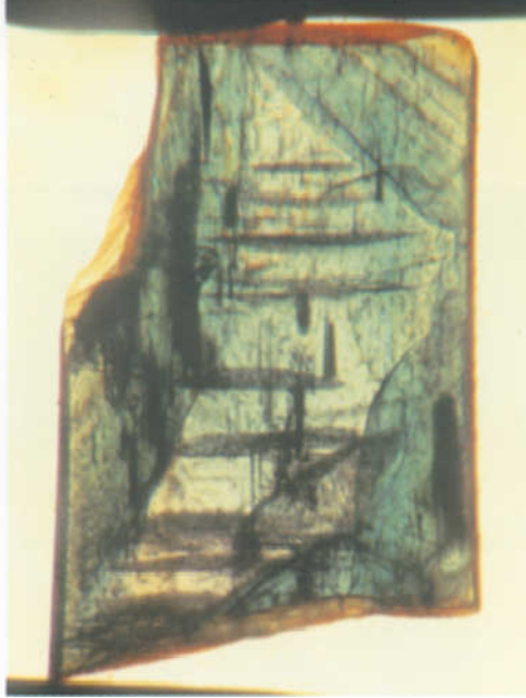
Figure 3: Prismatic crystal of Nacken synthetic emerald which contains a colourless, natural irregularly shaped seed; the c -axis runs vertically, melt filled channels and spicules are oriented parallel to c , flat cavities with primary liquid and two-phase inclusions are oriented perpendicular to c . Immersion, length of crystal. 3.4 mm.
