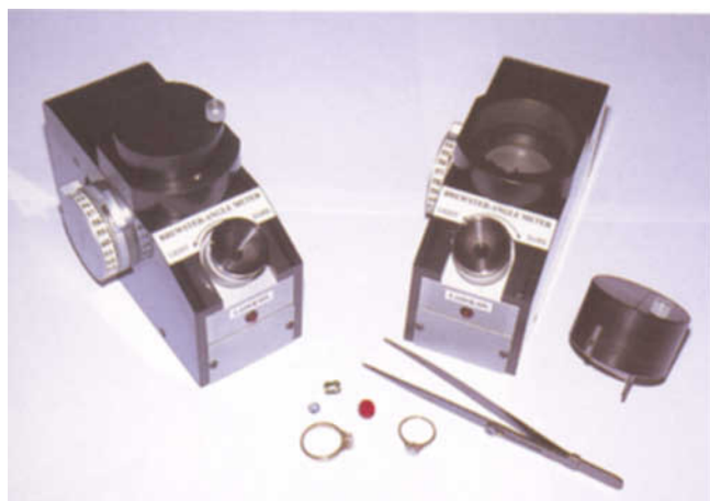
Figure 3: Two views of the GAGTL Brewster-angle meter. The operate button on the test plate cover is used to switch on the laser.
