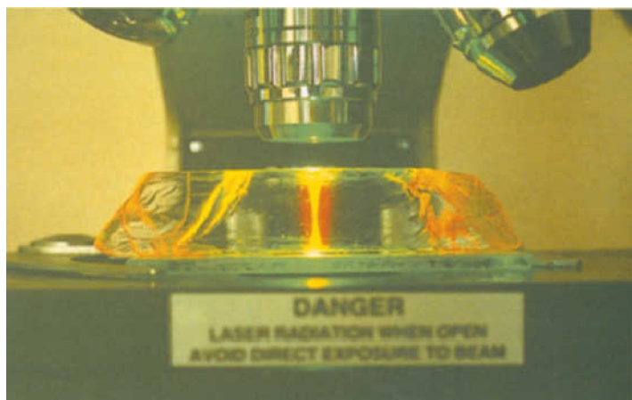
Figure 16: The laser beam of a Raman spectrometer focused in the middle of a transparent crystal. At the focus the excited volume is a few cubic microns. Photo by Thomas Ostertag.
