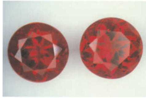
Figure 1: Two faceted synthetic red beryls produced in Russia each weighing approximately 1 ct.
