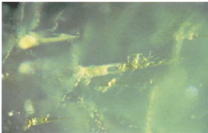
Figure 8: Elongated channel parallel to the c-axis with multicomponent filling and shrinking bubble. Renishaw Raman microscope. 200x.
