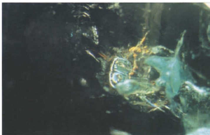
Figure 8: Trapped air bubbles and dendritic pattern in an epoxy resin-treated emerald. © SSEF Swiss Gemmological Institute.
