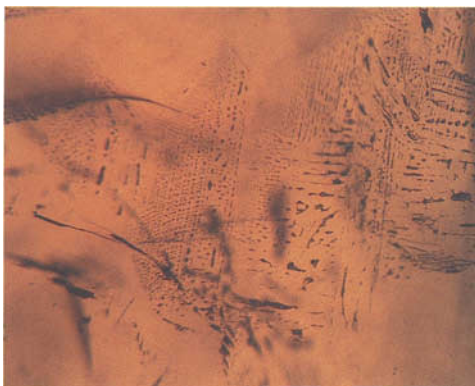
Figure 4: Healed cracks in spessartine from Nigeria.
