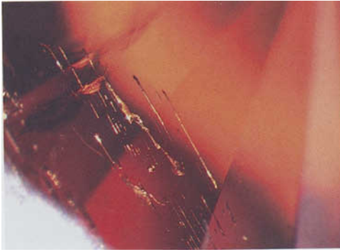
Figure 16: A cluster of parallel tubular, partially liquid-filled inclusions in sample G1.
