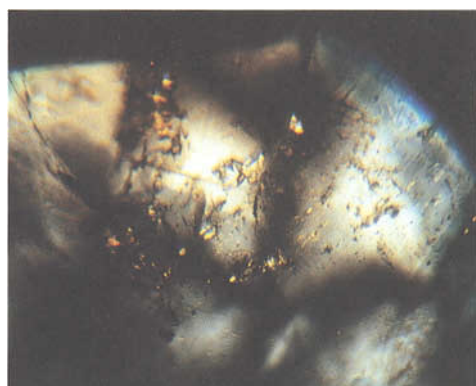
Figure 5: Tabby extinction visible under crossed polarizing filters.
