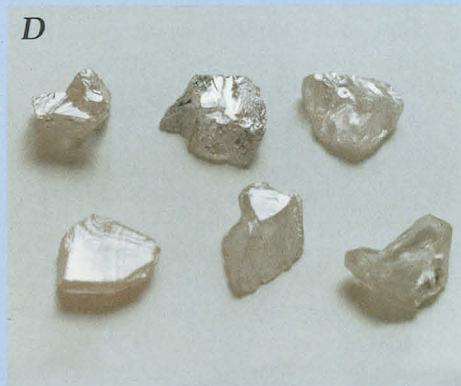
Figure 1: Examples showing irregular shapes of type II natural diamonds. A-C from the DTC Research Centre collection, magnification ca. 5-10x photomicrographs. To secure better views of surface features, combined illumination was used, which resulted in the appearance of brown tinted stones, B, C, being darker than they really are. D and E are from the DTC Sorting Room collection, macrophotographs, ca. 2x.
