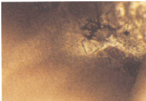
Figure 14: Crystallographically oriented rutile needles in a spinel from the new deposit in south-western Madagascar. Immersion, transmitted light, magnified 20x.
