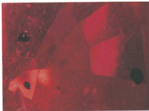
Figure 7: Rounded-elongate, dark brown and black opaque rutile crystals, displaying strong lustre. 50x; photo E. Gübelin.
