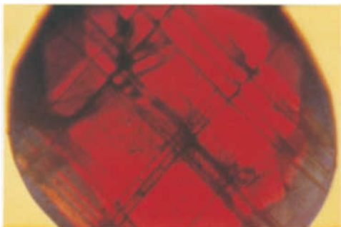
Figure 3: Vatomandry ruby with 'chessboard-like' pattern, caused by twin lamellae forming angles of almost 90°. 40x; photo K. Schmetzer.
