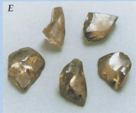
Figure 1: Examples showing irregular shapes of type II natural diamonds. A-C from the DTC Research Centre collection, magnification ca. 5-10x photomicrographs. To secure better views of surface features, combined illumination was used, which resulted in the appearance of brown tinted stones, B, C, being darker than they really are. D and E are from the DTC Sorting Room collection, macrophotographs, ca. 2x.
