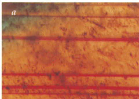
Figures 5 a and b: Pronounced polysynthetic twin lamellae, observed in polarized light, in different orientations of the polarizer. 50x. Photos K. Schmetzer.
