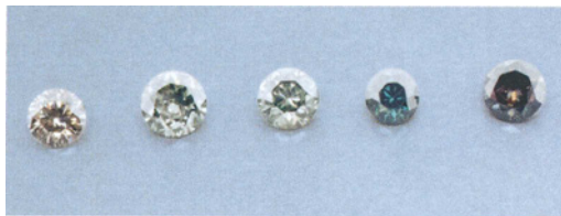
Figure 1: Faceted synthetic moissanites grown in St. Petersburg, Russia, by sublimation from the vapour phase. The samples range from 0.38 to 0.60 ct in weight and measure from 4.60 to 5.70 mm in diameter. Photo: © L.Kiefert, SSEF.
