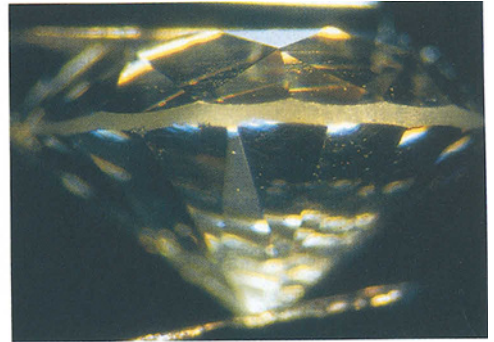
Figures 5 and 6: Pleochroism of bluish-brown synthetic moissanite which was determined as 4H-SiC by Raman spectroscopy. Figure 5 blue direction, Figure 6 brown direction. Sample is 5.40 mm in diameter. Photos: © H.A Hänni, SSEF.
