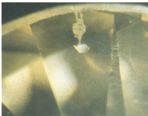
Figure 10: Tiny moissanite crystal or negative crystal with an elongate tube extending from this inclusion in yellow synthetic moissanite from Russia. Magnified 30 x. Photo: © H.A. Hänni, SSEF.
