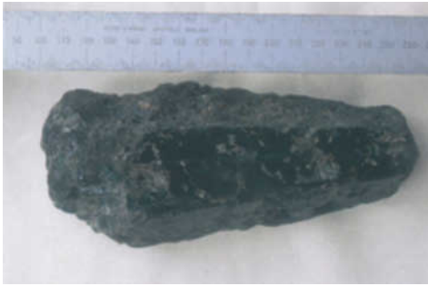
Figure 2: An artificially coloured quartz composite stone, weighing 0.82 kilograms.
