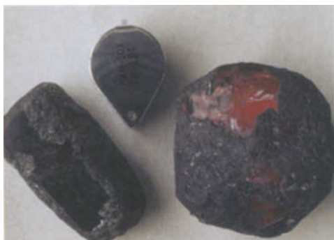
Figure 1: Green artificial glass imitating a piece of emerald rough, which weighs 40 grams, and an artificially coloured quartz composite imitating ruby rough, weighing 96.6 grams.
