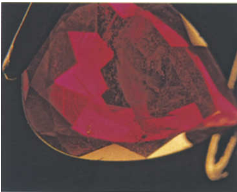
Figure 3: Parallel angular (V-shaped) growth zones observed in the 3.54 ct flux grown pear-shaped ruby. (Dark field illumination 40 \times ).
