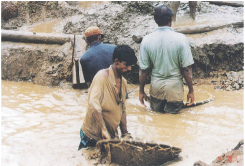
Figure 1: Washing of gem gravel using bamboo baskets.
