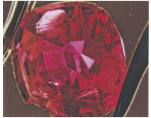
Figure 2: Enlarged view of the 3.28 ct cushion-shaped ruby. Notice the important break visible in the bottom right corner of the stone.
