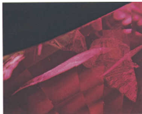
Figure 11: A 'feather' filled with precipitated substances (not analysed), observed in the 3.28 ct cushion-shaped ruby from Mong Hsu. (Dark field illumination 40×).
