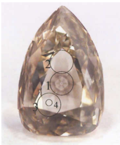
Figure 5: The four locations in sample A analysed using infrared and VIS/UV spectrometers to check the distribution of impurities and defects. Spot 1 has the highest cloud density, and spot 4 has the lowest. The two large parallel facets make this diamond an excellent specimen for spectroscopic measurement. The diameters of spots 1–3 are 2.0 mm and that of spot 4 is approximately 0.6 mm. Photograph by Elizabeth Schrader.
