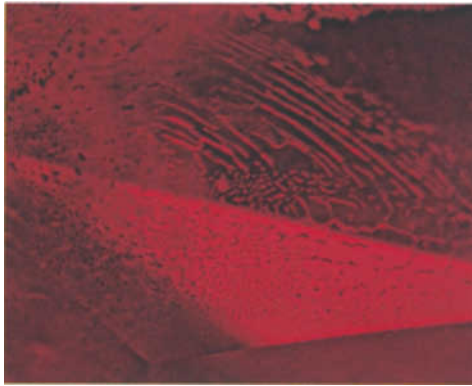
Figure 7: A veil-like 'flux feather' in the 3.54 ct flux grown pear-shaped ruby. (Dark field illumination 60×).
