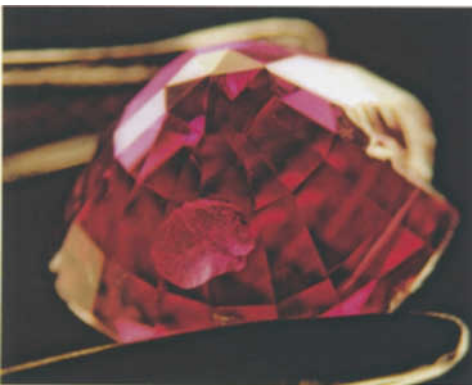
Figure 8: A large oval-shaped open cavity on the pavilion of the 3.28 ct cushion-shaped ruby from Mong Hsu. (Dark field illumination 10×).
