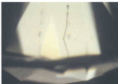
Figure 4: Bent channels were occasionally observed in synthetic moissanite. Magnification 5×, transmitted light. Photo by J. Shigley. © GIA.
