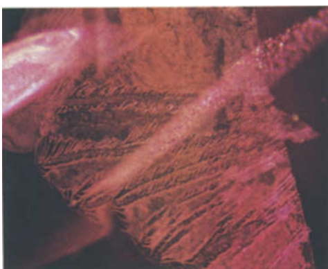
Figure 12: Enlarged view of the 'feather' in Figure 11 with patterns reminiscent of those observed in amethysts and described as 'zebra stripes'. (Dark field illumination, 80×).
