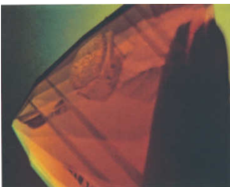
Figure 13: Polysynthetic twinning that penetrates the entire stone, observed in the cushion-shaped Mong Hsu ruby of 3.28 ct. (Immersed in methylene iodide and between crossed polars, 40×).
