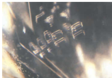
Figure 7: Double images of plate-like inclusions observed in a faceted synthetic moissanite. Magnification 20×, transmitted light dark field. Photo by T. Lu. © GIA.
