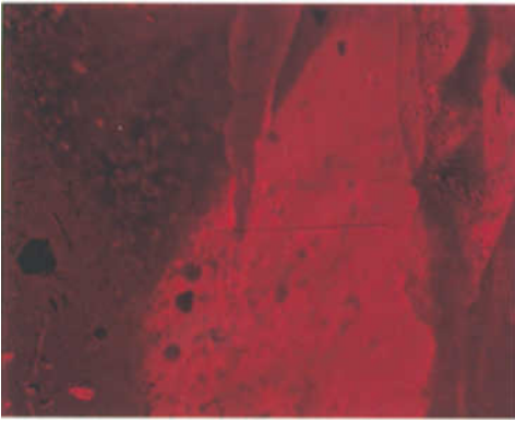
Figure 5: A long and extremely thin phantom-like acicular inclusion (unidentified) in the 3.54 ct flux grown pear-shaped ruby. (Dark field illumination 60×).
