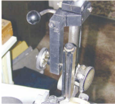
Figure 24: Detail of parallel bar hard stop with micro adjustment in Morgan concave facet machine.
