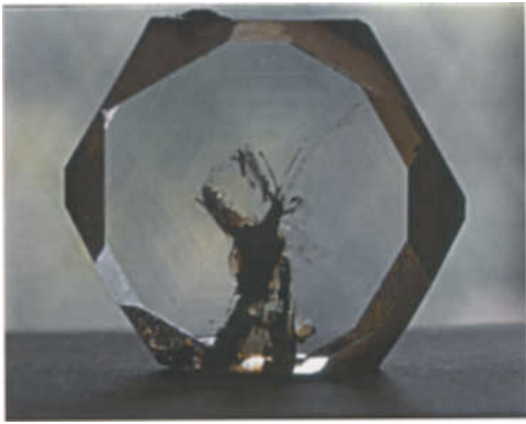
Figure 3: View parallel to the c -axis of a beryl crystal measuring approximately 49.5 mm across, 43 mm high and 13.8 mm thick. The crystal contains numerous inclusions and displays growth zones (seen as 'ripples') parallel to the prism faces.
