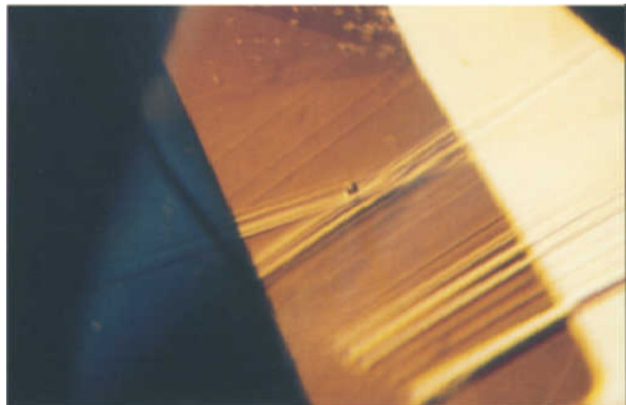
Figure 4: Enlarged view of a gas bubble lying at the junction of intersecting needle-like inclusions, in the sky-blue square cut glass of 2.44 ct (dark field illumination 25×).
