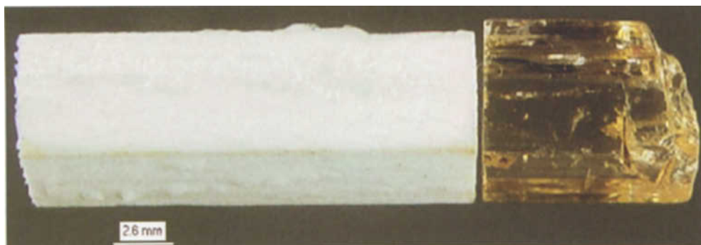
Figure 8: Mullite on the left formed by heating topaz at high temperature. The apparent difference in thickness is due to different orientation of the two crystal samples and is not an effect of the heat treatment.
