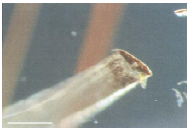
Figure 3b: Relatively thick coiled whisker very near the quartz surface and showing fibres making up the walls of a hollow cylinder. Bar 0.05 mm.
