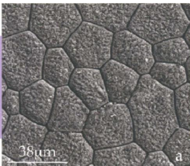
Figure 8a & b: Five- and six-sided calcite prisms and organic matter at boundaries.
