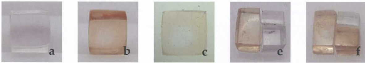
Figure 13: Photos of a 3.85 ct flame-fusion-grown colourless sapphire (PKSCS01) before treatment (a) and pale brown after Be-treatment under unknown conditions (b). The pale brown rim and colourless core are better seen under immersion (c). After the treatment the sample was cut in half and a five-point profile (d) was analysed across the cut surface using LA-ICP-MS (see also Table II, Figures 14 and 15). The other half was then cut into three pieces; one piece was kept as the reference and the other two were heated in a pure nitrogen atmosphere at 1650°C for three hours, which turned the stones colourless (e). One of the colourless pieces was then re-heated in air (i.e. oxidation conditions) at 1650°C for 1 hour, which turned the sample back to pale brown (f). (Photos by Somboon, GIT and Lomthong, KU)
