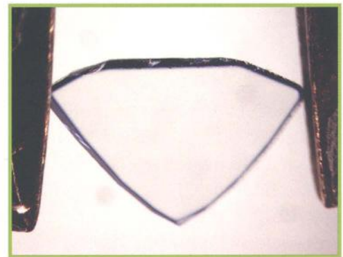
Figure 4: Slice of colourless sapphire with blue rim caused by external diffusion of Ti into the stone; 4 × 7 mm. (Immersion, photo by Häger)
