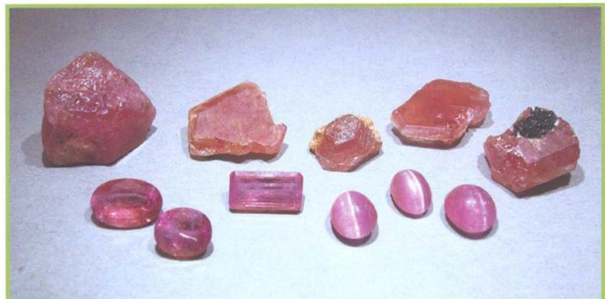
Figure 1: A selection of pezzottaite crystals with characteristic tabular habit. The cut stones are from 1.5 to 3.00 ct, (the step-cut sample in the middle is 12 mm long). Pezzottaites with a dense array of fine tubes (parallel to c) are cut as cabochons and produce cat's-eyes.
