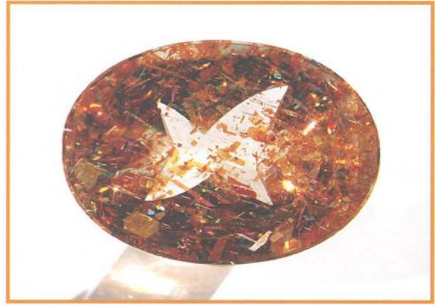
Figure 2: Faceted oligoclase feldspar from Oregon, USA. The pale red colour is due to concentrations of hematite inclusions (30.90 ct, cut by Tom Munsteiner).
