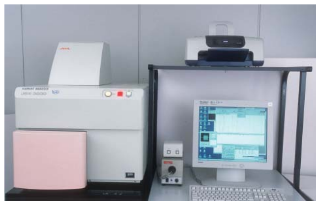
Figure 6: A JEOL energy dispersive X-ray fluorescence (EDXRF) spectrometer JSX-3600 used in this study is shown on the left. On the right is a close-up view of the newly developed goniometric sample stage for attachment to an EDXRF JSX-3600. A rotating stage with rotation angle ( \omega ) is mounted on the X-Y scanning stage, and a tilting stage with tilting angle ( \tau ) is placed on the rotation stage. The tilting stage can be inclined \pm 20^\circ . Each stage is labelled with a graduated scale underneath and is powered by a stepping motor. Photo by Masaaki Kobayashi (left) and A. Abduriyim (right).
