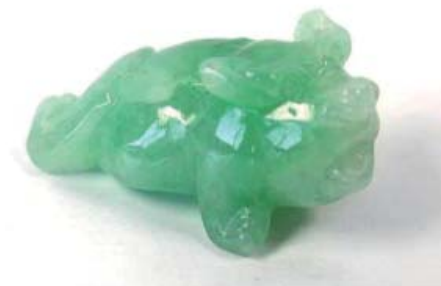
Figure 2: 'Cold' colour sharp reflections on the surface of a green A-jadeite carving.
