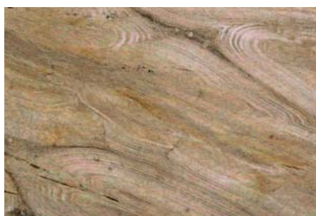
Figure 8b: Thin section of colloform variscite V5; fibres have aggregated to form elongated pods, with concentric growth patterns. Magnification 50x.
