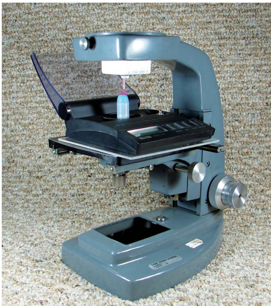
Figure 1: Apparatus used to measure magnetic susceptibility in this study.
