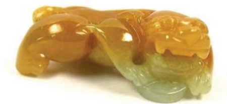
Figure 1: Example of vitreous reflection which is sharply defined and three light belts with sharp boundary on the back leg of the carving, characteristic of A-jadeite.
