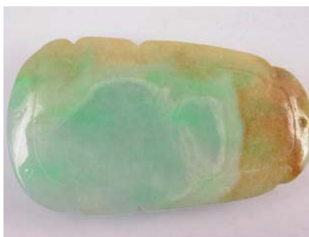
Figure 4: Clear colour boundaries and unaltered green core zones in partially weathered jadeite, characteristic of A-jadeite.
