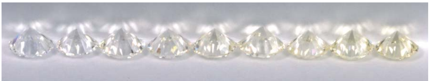
Figure 2: Complete set of GIA-graded diamond master stones from E through L and N.
