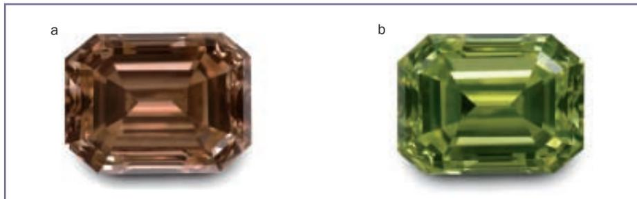
Figure 14 a,b: This type Ia diamond of 2.10 ct (a) was originally brown and treated in a HPHT process and became yellowish green (b). Photograph by courtesy of T. Hainschwang, Gemlab, Gemological Laboratory, Balzers, Liechtenstein.
