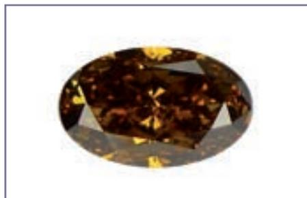
Figure 13: This type Ia diamond of 1.30 ct was originally brown and treated in a HPHT process. Photograph by courtesy of E. Erel, Carat Gem Lab, Gemological Laboratory, Montigny-les-Metz, France.
