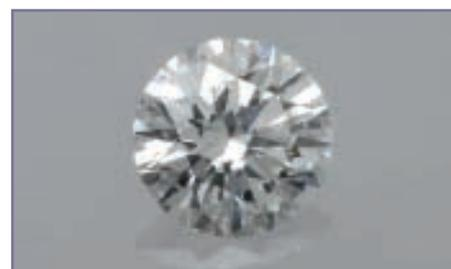
Figure 8: This type IIa diamond of 0.70 ct was originally brown and treated in a HPHT process. Photograph by courtesy of J.-P. Chalain, SSEF Swiss Gemmological Institute, Basel, Switzerland.
