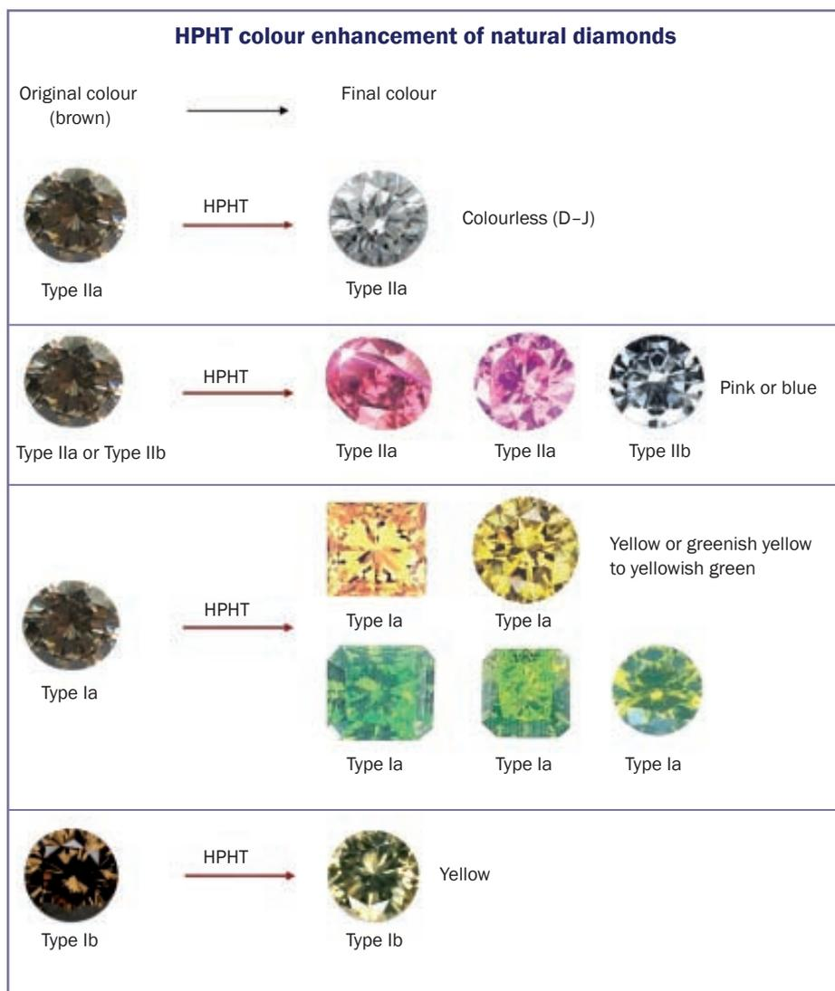
Figure 7: Systematic overview of possible colour alteration by HPHT treatment of natural brown type I and II diamonds. This diagram is based on a somewhat smaller schema by V. Vins, Institute of Single Crystals, Novosibirsk, Russia, which has been extended by the present author.
