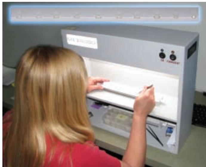
Figure 9: Grading in the DiamondDock at the AGS Laboratory with (inset) a 10-diamond master set. Courtesy of AGSL.
