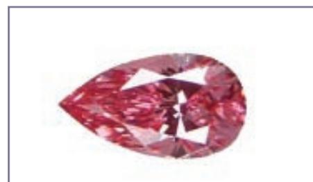
Figure 9: This type IIa diamond of 0.50 ct was originally brown and treated in a HPHT process. Photograph by courtesy of E. Erel, Carat Gem Lab, Gemological Laboratory, Montigny-les-Metz, France.
