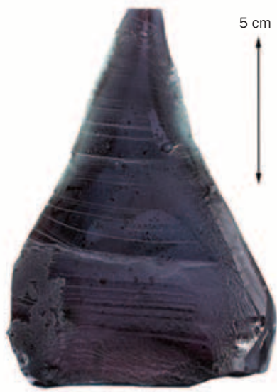
Figure 4: Complete alexandrite crystal grown by the HOC technique in a molybdenum container in Novosibirsk. Weight of the crystal approx. 420 g. Photo courtesy of V.V. Gurov.
