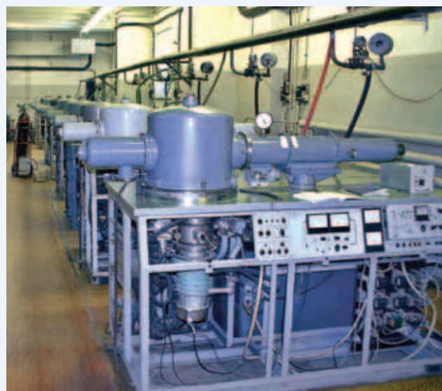
Figure A2: Production hall with numerous HOC facilities for the growth of large single crystals of compounds with high melting temperatures; Institute of Geology and Mineralogy, Siberian Division, Russian Academy of Sciences, Novosibirsk, Russia. Photo courtesy of V.V. Gurov.
