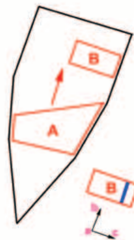
Figure 8: This schematic drawing shows the position of the two alexandrite crystals depicted in Figure 5 in the molybdenum container applied for crystal growth as indicated by the producer; the growth direction (red arrow) is almost parallel to the b-axis and perpendicular to the c-axis of the alexandrite crystal (indicated schematically below right with black arrows); the position and orientation of the slab cut parallel to the ab-plane and used for chemical analysis (five scans by electron microprobe) is indicated in blue.
