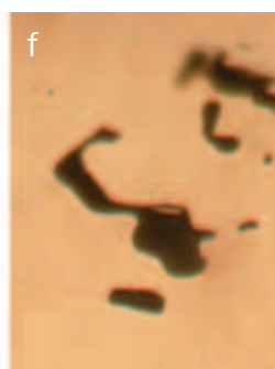
Figure 14: Irregularly-shaped flat cavities in an HOC alexandrite: (a) overview in the direction parallel to the b-axis; (b) in plane polarized light and (c) between crossed polarizers; in (c) only small reflections of the edges of the cavities are visible, but no birefringent solid phase is present; in immersion (d–f), under various angles to the illuminating light beam, the cavities appear transparent (d), semitransparent (e) or opaque (f). Field of view (a) 3.8 \times 2.8 mm; (b–f) 1.05 \times 0.8 mm. Photos a and d–f by K. Schmetzer; b and c by T. Hainschwang.
