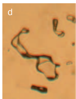
Figure 14: Irregularly-shaped flat cavities in an HOC alexandrite: (a) overview in the direction parallel to the b-axis; (b) in plane polarized light and (c) between crossed polarizers; in (c) only small reflections of the edges of the cavities are visible, but no birefringent solid phase is present; in immersion (d–f), under various angles to the illuminating light beam, the cavities appear transparent (d), semitransparent (e) or opaque (f). Field of view (a) 3.8 \times 2.8 mm; (b–f) 1.05 \times 0.8 mm. Photos a and d–f by K. Schmetzer; b and c by T. Hainschwang.
