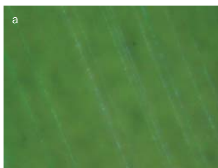
Figure 16a,b: Thin sections of Kyocera chatoyant synthetic alexandrites oriented almost perpendicular to the b pinacoid show layers parallel to the a plane with numerous tiny needles alternating with layers of transparent alexandrite. The layers are thicker in b . Reflected light, crossed polarizers, field of view 112 x 84 \mu\text{m} . Photos by H.-J. Bernhardt.
