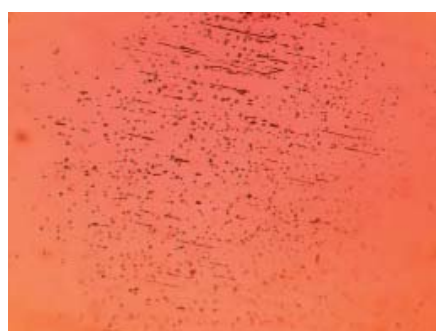
Figure 11: Mostly rounded, occasionally also somewhat elongated gas bubbles in synthetic alexandrite. Immersion, field of view 3.7 x 2.7 mm. Photo by K. Schmetzer.
