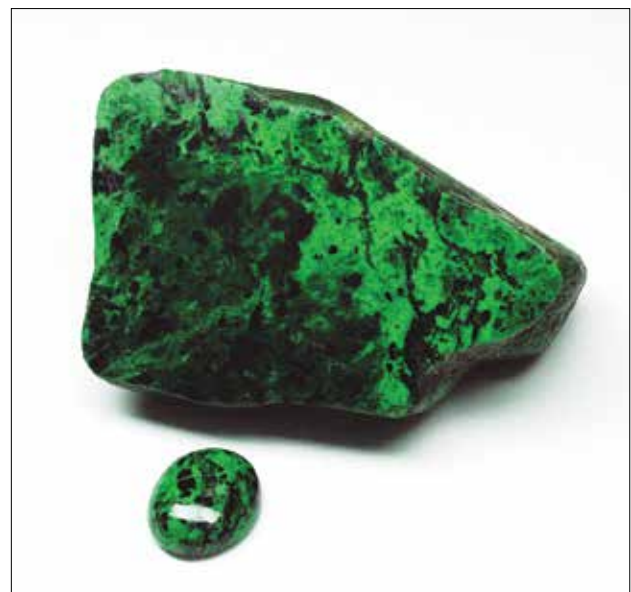
Figure 2: Kosmochlor is one of the many constituents of maw-sit-sit, a rock that also commonly contains chromian jadeite, albite, clinocllore, amphibole and chromite. The cabochon shown here weighs 12.09 ct and the polished cobble is 128.02 g (65.7 × 45.3 mm). Photo by Tay Thye Sun.
