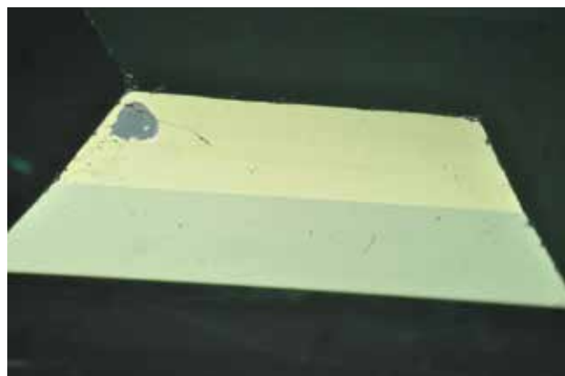
Figure 3: The chipped areas on the pavilion of the 13.45 ct emerald show the duller lustre of the underlying emerald against the bright metallic lustre of the coated facets. Also note the dark line corresponding to a surface-reaching fracture that cross-cuts the large chip. Photomicrograph by G. Choudhary; reflected light, magnified 24 \times .
