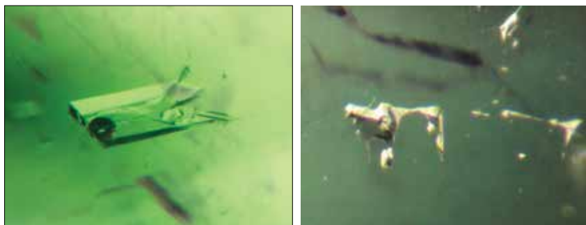
Figure 12: Primary two-phase (liquid-gas) inclusions display various jagged forms in the Vietnamese fluorite. Photomicrographs by M. Chaipaksa; magnified 70 \times .
