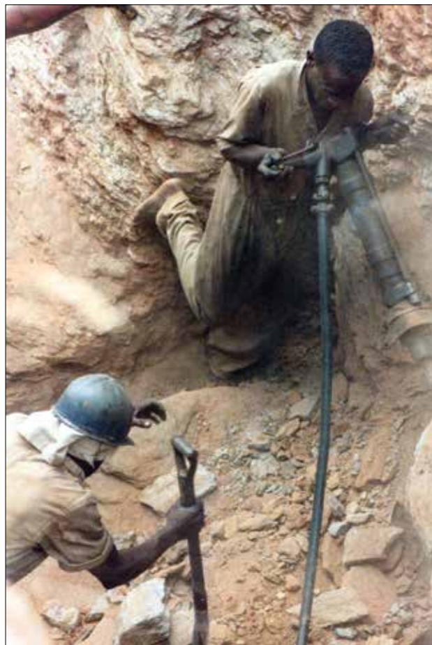
Figure 10: Here the team uses an 80 lb (36 kg) jackhammer to break up the country rock in the weathered horizon, at a depth of \sim 30 feet (9.1 m) from the surface. At greater depths, the unweathered rock is extremely hard and requires blasting with explosives. Photo by J. Walker, 1997.
