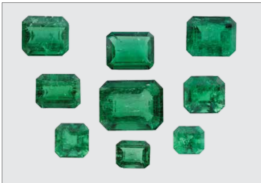
Figure 1: These nine faceted emerald samples (3.54–33.64 ct) proved to be coated with an ultrathin carbon-based film on their pavilion facets. Composite photo by G. Choudhary.
