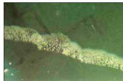
Figure 13: This partially healed fracture in the fluorite consists of a plane of fluid inclusions. Photomicrograph by M. Chaipaksa; magnified 50 \times .
