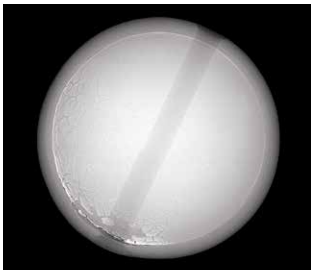
Figure 31: With microradiography, a round bead is clearly visible, identifying the sample as a beaded cultured pearl.
