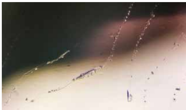
Figure 2: Elongate, centipede-like inclusions are seen in one of the Austrian moonstones. Photomicrograph by M. Chaipaksa; magnified 70×.
