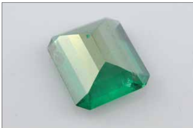
Figure 2: The pavilion facets of this 13.45 ct emerald show a golden metallic to sub-metallic lustre that indicates the presence of a coating. Also note the chip in the coating near the keel of the pavilion toward the upper left. Photo by G. Choudhary.
