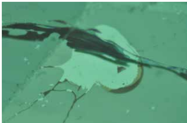
Figure 4: Under diffused transmitted light, the coating layer appears brown, particularly around the chipped areas. Note the difference in colour between the underlying emerald and the surrounding coated surface. Also, the underlying fracture contains some subtle bluish flashes suggesting the presence of resin filler. Photomicrograph by G. Choudhary; magnified 64 \times .
