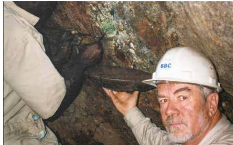
Figure 12: Campbell Bridges supervises the extraction of a tsavorite nodule from the No. 2 tunnel of the Scorpion mine. Lightweight hand tools are utilized to minimize damage to the gem material. Photo by J. Walker, 2003.
