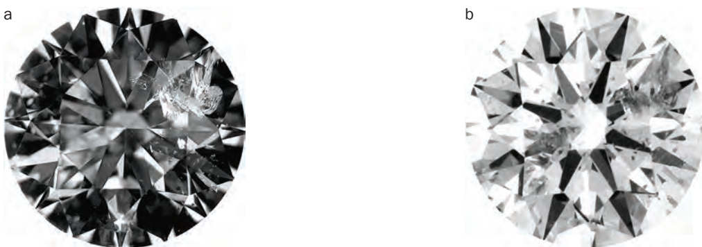
Figure 21: This 0.35 ct I_2 -graded diamond (4.55–4.54 × 2.78 mm) contains a large I_1 -size fracture that is best seen with darkfield illumination (a). Viewed with overhead lighting (b), a reflection of the fracture causes a doubling of its apparent area, which combined with the relatively small size of the diamond leads to a solid I_2 clarity grade.
