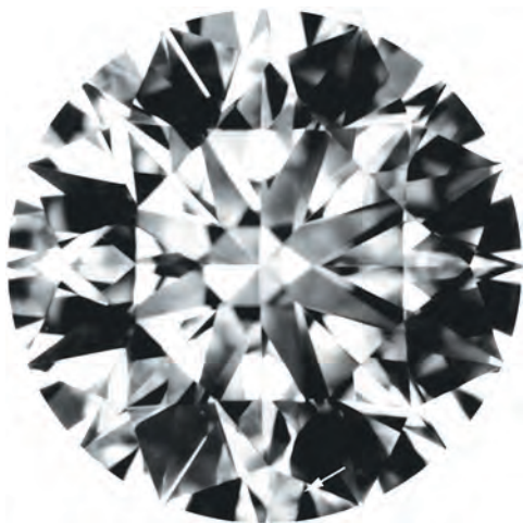
Figure 14: This 0.92 ct VVS_1 -graded diamond ( 6.22\text{--}6.23 \times 3.85 mm) contains a VVS_2 -size pinpoint. The position of this inclusion near the girdle at 6 o'clock calls for a half-grade adjustment, making the clarity grade a low VVS_1 .
