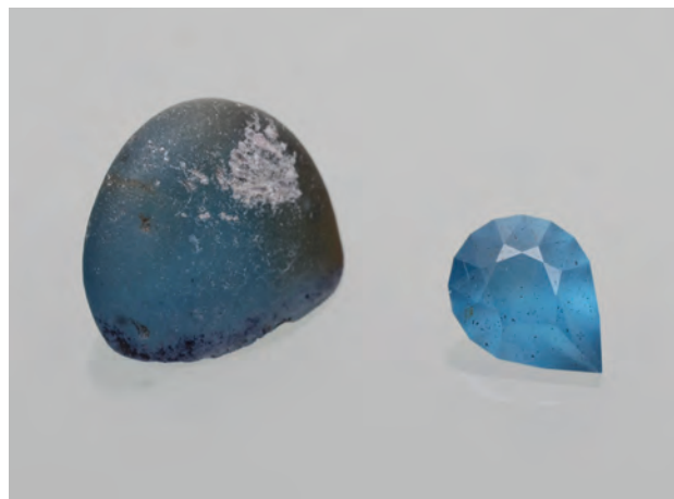
Figure 16: These translucent blue samples proved to be polycrystalline kyanite. The sawn pebble (7.48 ct) is what remains after cutting of the pear-shape gem (1.72 ct). Photo © M. S. Krzemnicki, SSEF.
