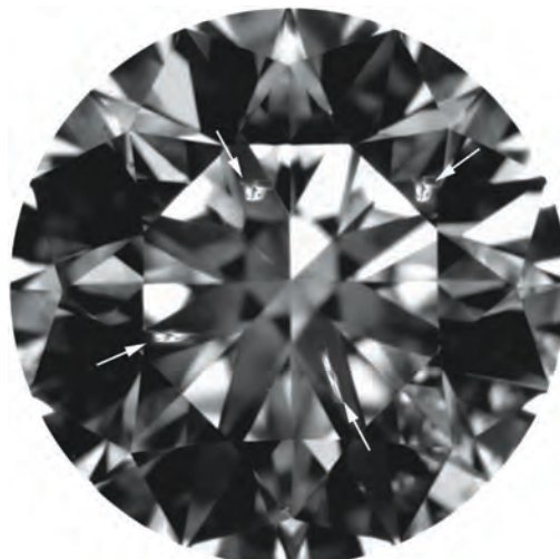
Figure 4: This 1.11 ct diamond (6.66–6.63 × 4.11 mm) contains four SI 1 -size inclusions that have different dimensions, but the same area and contrast, and thus similar noticeability. Each has an area determined to be approximately 35,000 μm 2 .
