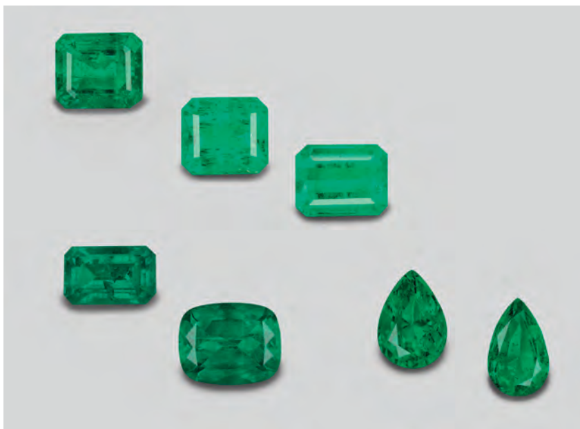
Figure 1: Some of the emeralds studied for this report are shown here. Top row, from left to right: 0.76 ct from Davdar, China; and 0.71 and 0.66 ct from Colombia. Bottom row, from left to right: 1.14 ct synthetic Taurus 'Platinum'; 2.34 ct synthetic Chatham; and 0.37 and 0.23 ct from Kafubu, Zambia. Composite photo by Bilal Mahmood, American Gemological Laboratories.
