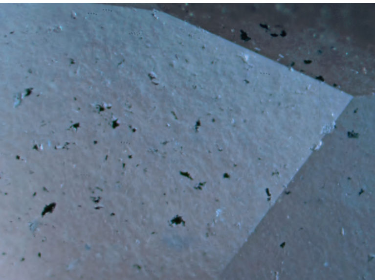
Figure 17: Viewed with the microscope, the faceted polycrystalline kyanite showed a treacle-like appearance and numerous black residues of polishing powder in small cavities on the polished surface. Photomicrograph © M. S. Krzemnicki, SSEF; magnified 60 \times .
