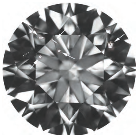
Figure 5: This 0.70 ct diamond (5.74–5.71 × 3.52 mm) contains four VS 2 -size inclusions between the 10 and 11 o'clock positions near the table edge. All of these inclusions have the same area and noticeability, despite their varying dimensions.
