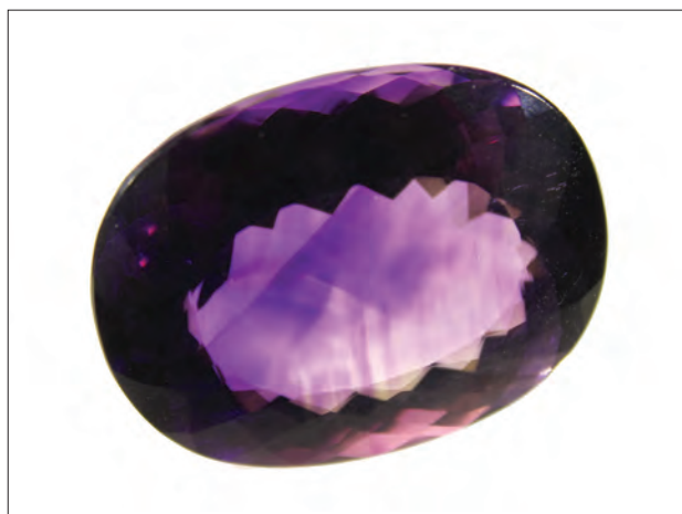
Figure 6: Straight and angular colour zoning is evident in this 113.79 ct São Paulo amethyst. Photo by B. Williams.
