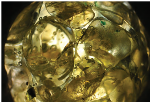
Figure 27: The bead in Figure 26 consisted of several pieces of yellowish green peridot embedded in a pale yellow polymer matrix. Note the presence of gas bubbles confined to the interstitial polymer areas. Photomicrograph by G. Choudhary; magnified 24×.
