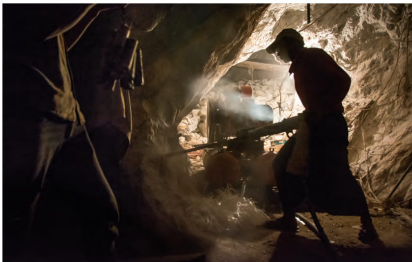
Figure 4: A miner dressed in a longyi (traditional Burmese skirt) uses a pneumatic drill to prepare the marble for blasting. His assistant in the left foreground holds several sticks of explosives. Photo by B. M. Laurs.
