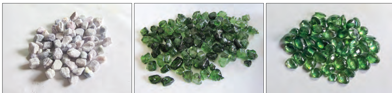
Figure 4: These images show the corundum starting material after acid cleaning (left), and rough and faceted lead-glass-filled green sapphires after the treatment (centre and right). The rough stones weigh 1–5 g and the faceted samples are 1–3 ct. Photos by S. Promwongnan and N. Susawee.
