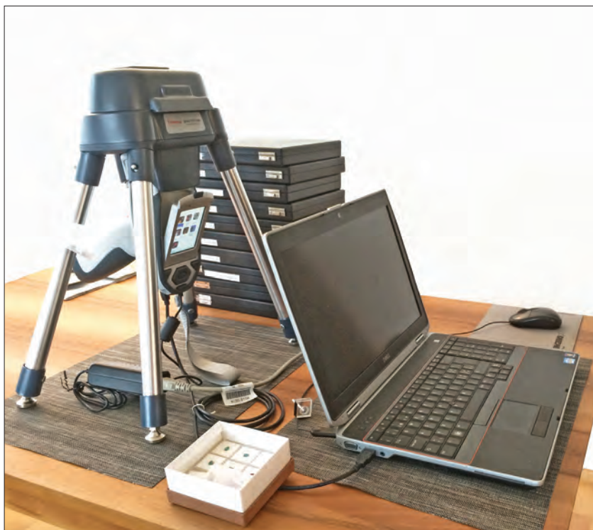
Figure 3: The EDXRF unit is seen here mounted in a stand used for analysing small samples. The sample chamber (18 × 8 cm) is large enough to accommodate a variety of unmounted samples, but may be too small for bulky jewellery items; larger stands are available. Photo by H. A. Hänni.
