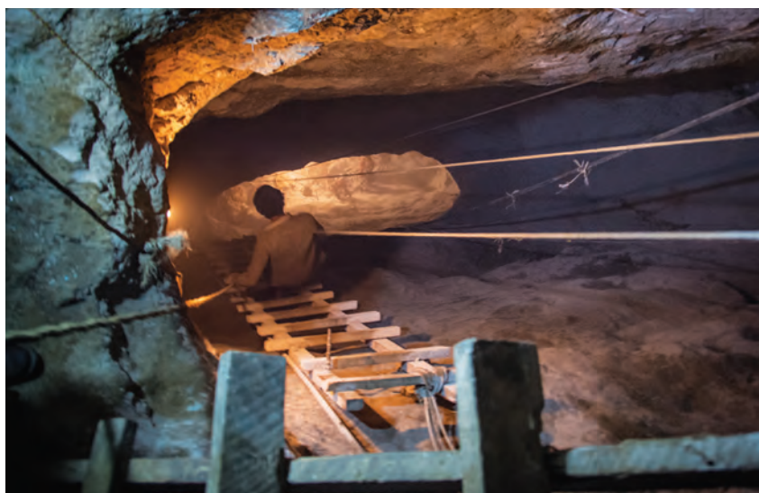
Figure 3: A miner descends a steep ladder to the working face where marble is drilled and blasted in search of rubies. The cables on the right are used to hoist the marble to a haulage tunnel, where it is then loaded into ore cars. Photo by B. M. Laurs.
