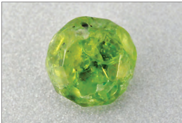
Figure 26: This 3.25 ct bead turned out to be a composite, made up of pieces of peridot embedded in a polymer matrix. Photo by G. Choudhary.
