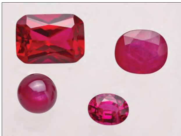
Figure 6: The corundum gems analysed for this study are (clockwise from top left): a 9.10 ct Verneuil synthetic ruby (sample 1), a 4.83 ct ruby with Pb-glass filling (sample 4), a 1.86 ct flux-grown synthetic ruby from Ramaura (sample 2), and a 4.12 ct natural untreated star ruby from Mogok (sample 3). Photo by H. A. Hänni.
