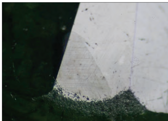
Figure 9: These views show a glass-filled cavity within a treated sapphire in darkfield (left) and reflected light (right). Photomicrographs by N. Susawee; magnified 20 \times .
