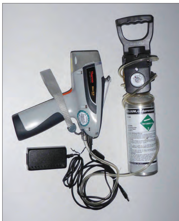
Figure 2: The portable EDXRF device (Niton XL3t GOLDD+ from Thermo Scientific) tested for this study is shown on the left, together with cables for its power and USB connections. On the right is the He purge unit that is used for light-element analysis. The image scale can be judged from the size of the AC power adapter (6 × 10 cm). Photo by F. A. Herzog.
