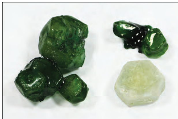
Figure 2: Shown here is an example of the low-quality pale coloured corundum that is used as the starting material for glass filling (bottom right, 3.15 g), together with two fused pieces of corundum and green glass after the treatment process (10.17 and 1.76 g). Photo by N. Atsawatanapirom.
