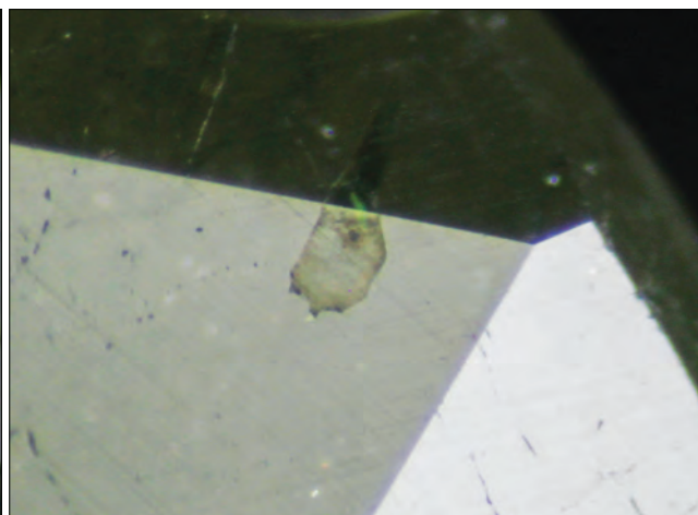
Figure 10: Reflected light reveals the lower lustre of the lead-glass filler in fissures (left, magnified 32 \times ) and in a cavity (right, magnified 16 \times ) as compared to the host sapphire. Photomicrographs by N. Atsawatanapirom.
