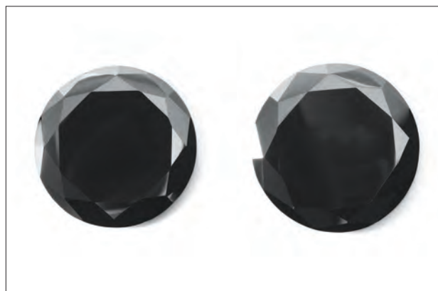
Figure 22: These large black diamond imitations (left, 29 ct and right, 34 ct) consist of very fine-grained synthetic moissanite. Photo by C. Caplan.
