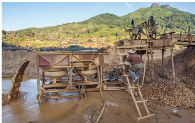
Figure 8. At the washing plant, rocks larger than 2.5 cm are screened off, and the remaining material is washed into a jig. Photo by B. M. Laurs.
