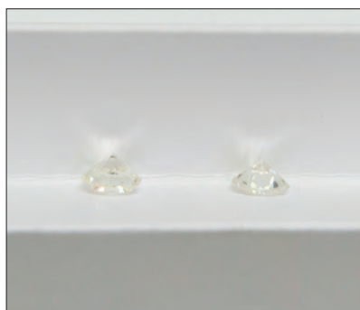
Figure 1: The conventional way to colour grade diamond simulants is as done for D-to-Z diamonds, with both the sample and master stone in the face-down position against a white or light grey background, using daylight-equivalent fluorescent light. Here, a master stone is on the left and a synthetic moissanite is on the right. Each gem is approximately 5 mm in diameter. Photo courtesy of Charles & Colvard Ltd.
