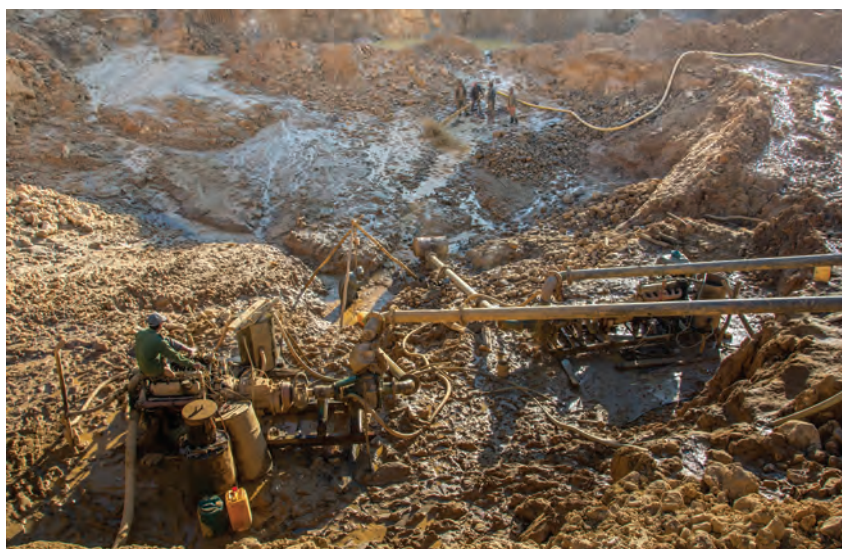
Figure 7. A water cannon is used to wash gem-bearing material into a small collecting area, or sump, from where it is pumped out of the pit to a processing plant. Photo by B. M. Laurs.
