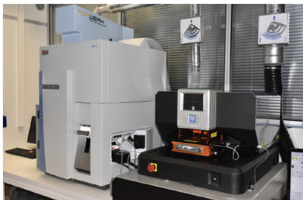
Figure 2: This LA-ICP-TOF-MS system, named GemTOF, was installed at SSEF in July 2016. The ICP-TOF-MS instrumentation is on the left and the LA unit is on the right. Photo by Vito Lanzafame, SSEF.
