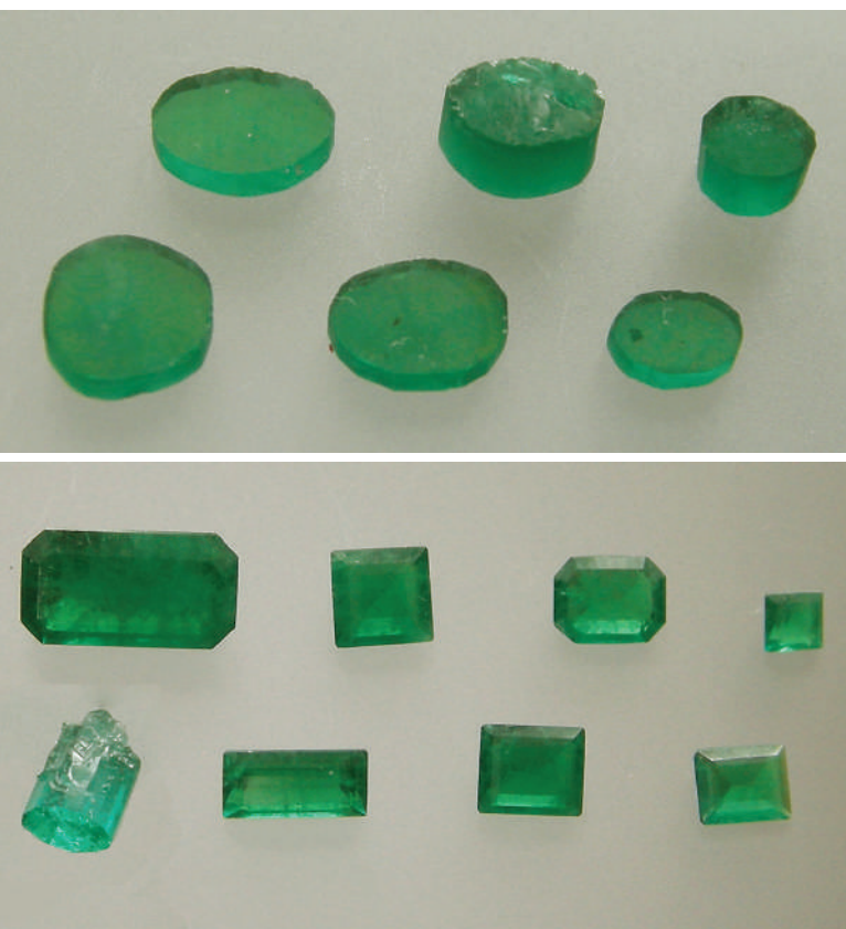
Figure 22: These photos show some of the samples of type 4 Cr- and Ni-bearing synthetic emerald studied from the collection of the Technische Universität Bergakademie Freiberg. Top: Tabular plates or short prismatic crystals—the crystal in the upper row, centre, measures 8.6 \times 5.7 \times 3.8 mm and weighs 1.62 ct. Bottom: Faceted samples; the largest at the upper left measures 13.5 \times 7.6 mm and weighs 4.04 ct; shown for comparison is a Cr-bearing synthetic emerald crystal at the lower left from the early Chatham production measuring 5.2 \times 3.6 mm and weighing 0.40 ct. The use of Ni in addition to Cr caused a somewhat more yellowish green coloration for the synthetic emeralds produced by IG Farben. Photos by K. Schmetzer.
