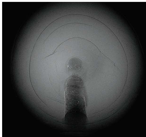
Figure 31: X-radiography of the pearl shows an unusual structure (approximately 1.3 mm long) in the centre, close to the end of the drill hole. Image by O. Segura.
