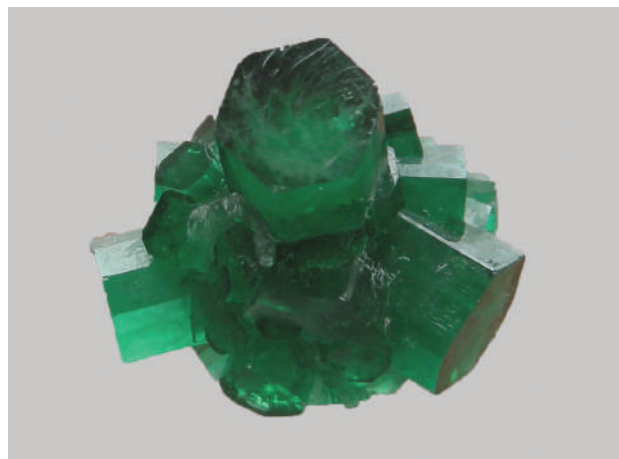
Figure 14: This cluster of type 1 synthetic emerald crystals (20.4 × 17.3 × 13.6 mm) was produced by IG Farben without the addition of a Ni-bearing compound and is from the collection of C. Weise, Munich. Photo by K. Schmetzer.
