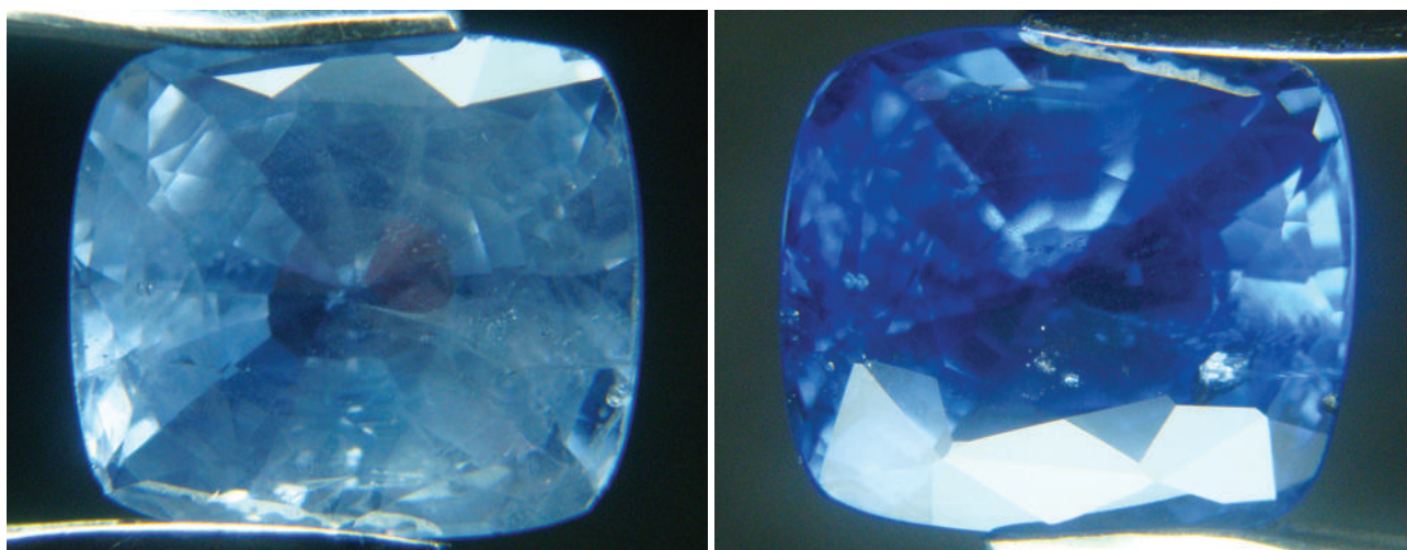
Figure 37: This 1.19 ct sapphire is shown before (left) and after (right) HPHT treatment. Photomicrographs by Youngsoo Chung; magnified 10 \times .
