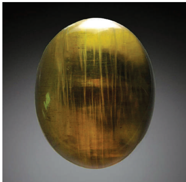
Figure 5: Elongate planar veils traverse the length of the 584.22 ct apatite, as shown here in transmitted daylight-equivalent illumination. The c-axis is oriented perpendicular to these veils. Photo by J. Rakovan.
