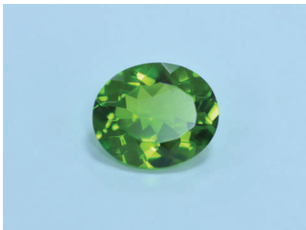
Figure 34: This faceted 6.08 ct sample was identified as a new imitation of peridot: yttrium aluminosilicate glass. Photo by W. Han.
