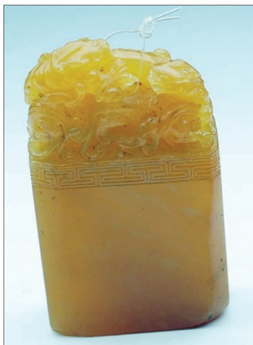
Figure 9: Left: This yellow stone carving (44.90 × 26.58 × 12.19 mm) was found to be a material known as Tianhuang in China, which may consist of the kaolinite-group minerals dickite and/or nacrite. Right: In this view, the main flat side of the carving displays whitish vein-like patterns. Photos by Tay Thye Sun.
