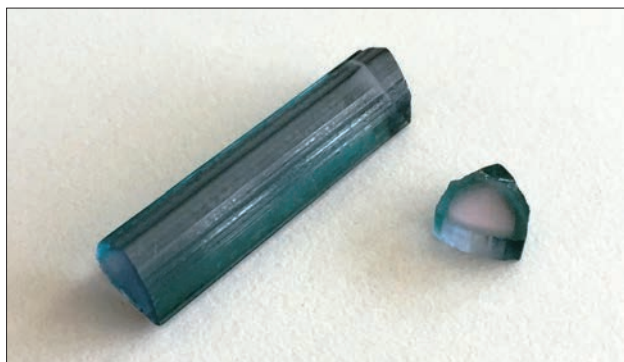
Figure 47: This sample of borosilicate glass was sliced into two pieces and examined for this report. The length of the larger piece is 30 mm. Photo by Lore Kiefert.
