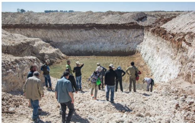
Figure 30: Field trip participants survey one of the mining trenches at the London Run deposit. The light-coloured sediments in the pit walls are diamond bearing, and they are overlain by a dark-coloured soil horizon and previously mined material. Photo by B. M. Laurs.
