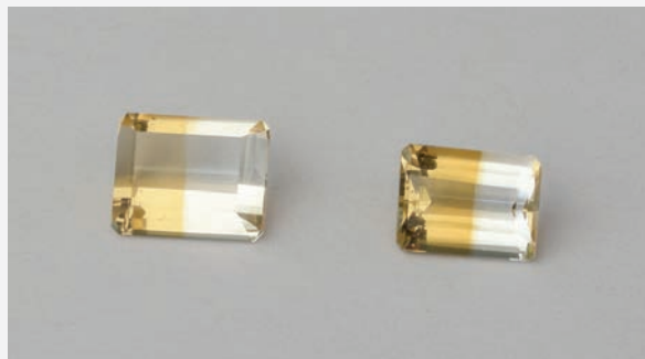
Figure A-1: Faceted colour-zoned quartz consisting of a lighter yellow, almost colourless, zone and a more intense yellow zone is referred to as 'Luna y Sol' or 'Lunasol' in the trade. These examples weigh 3.17 ct (left, 10.0 × 8.0 mm) and 2.14 ct (right). Photo by K. Schmetzer.
