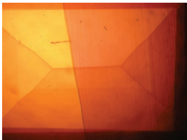
Figure 29: Growth striations are frequently seen in the violet zones of faceted synthetic ametrine. These striations are parallel or only slightly inclined to the violet/yellow boundary. Photomicrograph by K. Schmetzer; field of view 5.8 × 4.4 mm.
