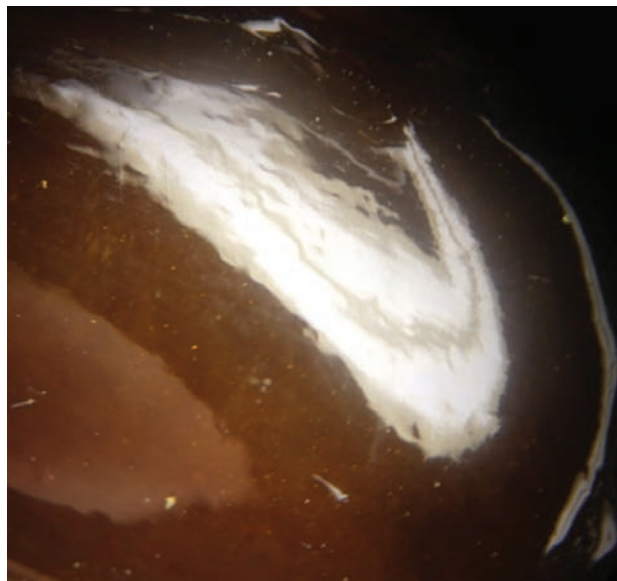
Figure 10: Ripples are seen on the surface of baked amber JF-1. Photomicrograph by Y. Wang; magnified 10 \times .
