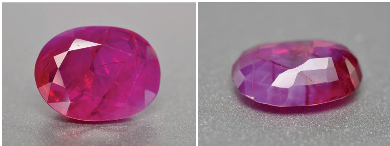
Figure 50: Left: This 6.20 ct bright purplish red oval cut with pronounced orange fractures was identified as a synthetic ruby. Note also the subtle milkiness throughout the sample. Right: The pavilion of the synthetic ruby exhibits a large cavity instead of a culet, which is a common cutting style in 'old' stones originating from Burma (Myanmar). Also visible is a strong sheen effect in some areas. With this combination of features, this synthetic could easily be mistaken for a natural ruby. Photos by G. Choudhary.
