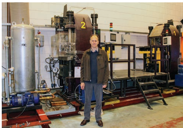
Figure 42: At the AOTC research facility in The Netherlands, two older presses, each weighing 17 tonnes, are still in use. Co-author Branko Deljanin poses for scale. Photo by J. C. Zwaan.
