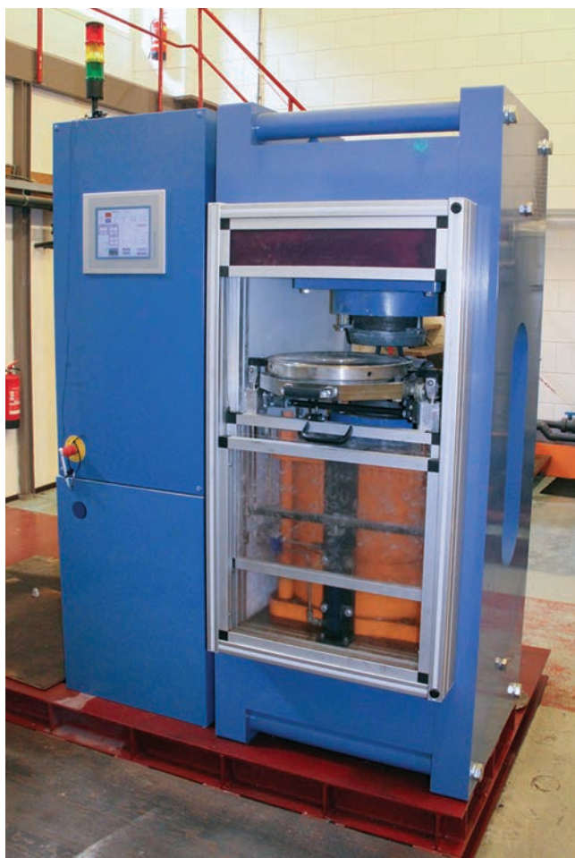
Figure 43: New Bridgman-type presses such as this one (front and back) provide significant advances in the efficiency of growing synthetic diamonds. Photos by J. C. Zwaan.
