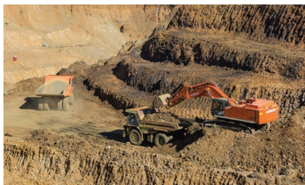
Figure 28: An excavator and dump trucks are used to mine this open pit at the Tirisano deposit. Photo by B. M. Laurs.
