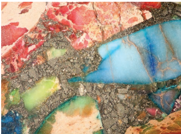
Figure 55: Microscopic observation of the surface of the sample in Figure 54 shows differently coloured areas with heterogeneous colour distribution, including some fragments that appear to be partially without colouring. The reflective metallic matrix consists of a colourless substance embedded with fragments of pyrite. Photomicrograph by F. Schmitz; magnified 30 \times .
