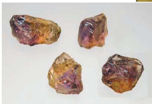
Figure 3: Quartz crystals from the Anahí mine are sawn and/or cobbled at the processing plant of the company Minerales y Metales del Oriente . Photo taken in 1997, courtesy of Udo Reimann. This process leaves irregularly shaped pieces of quartz (here, 5.7–9.3 g) that commonly exhibit a distinct colour boundary (inset photo by K. Schmetzer).
