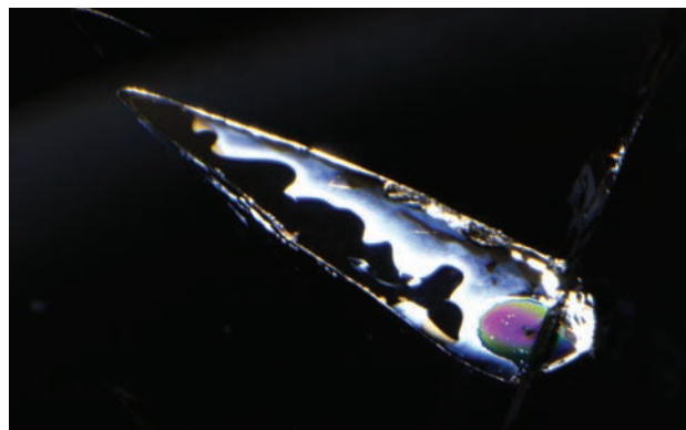
Figure 39: This biotite inclusion in quartz showed a highly reflective mirror-like interface and a circular area of thin-film interference colours. Photomicrograph by N. D. Renfro, © GIA; image width 4.7 mm.
