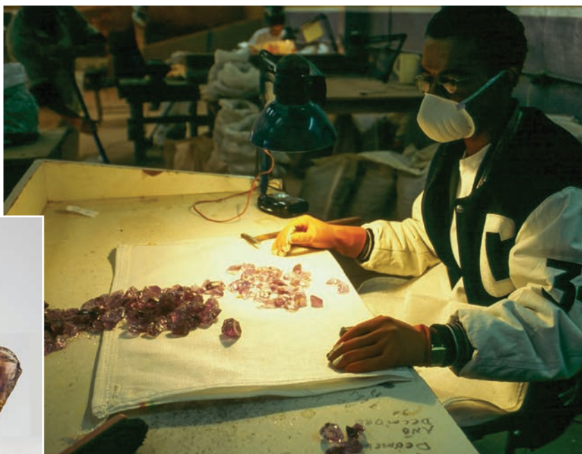
Figure 3: Quartz crystals from the Anahí mine are sawn and/or cobbled at the processing plant of the company Minerales y Metales del Oriente . Photo taken in 1997, courtesy of Udo Reimann. This process leaves irregularly shaped pieces of quartz (here, 5.7–9.3 g) that commonly exhibit a distinct colour boundary (inset photo by K. Schmetzer).
