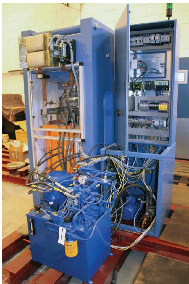
Figure 43: New Bridgman-type presses such as this one (front and back) provide significant advances in the efficiency of growing synthetic diamonds. Photos by J. C. Zwaan.
