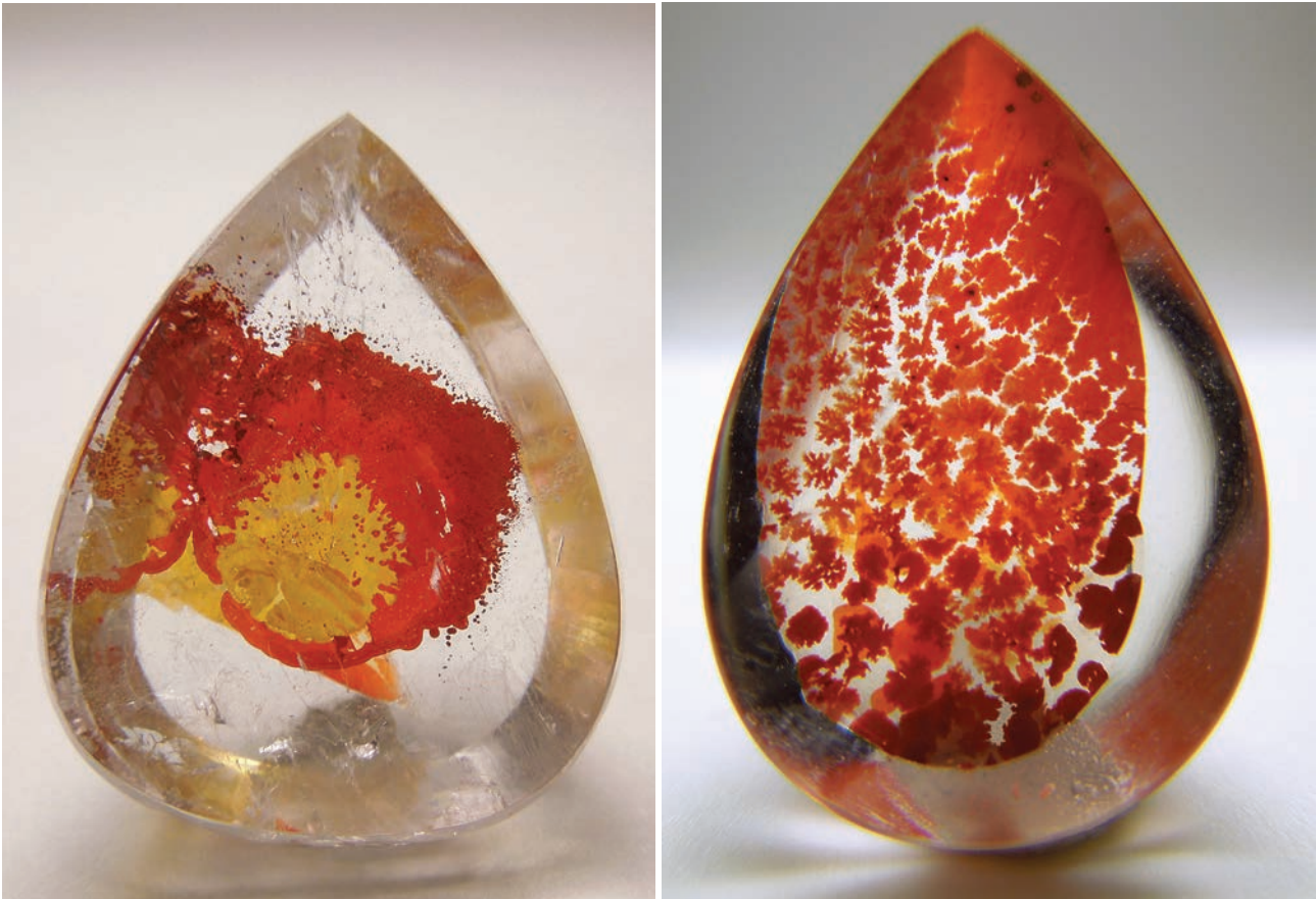
Figure 34: The red and yellow inclusion assemblage in the quartz on the left (~19 ct) probably consists of hematite and goethite, respectively. Dendritic patterns are seen in the hematite inclusions within the quartz on the right (4.68 ct). Specimens and photos courtesy of Luciana Barbosa.
