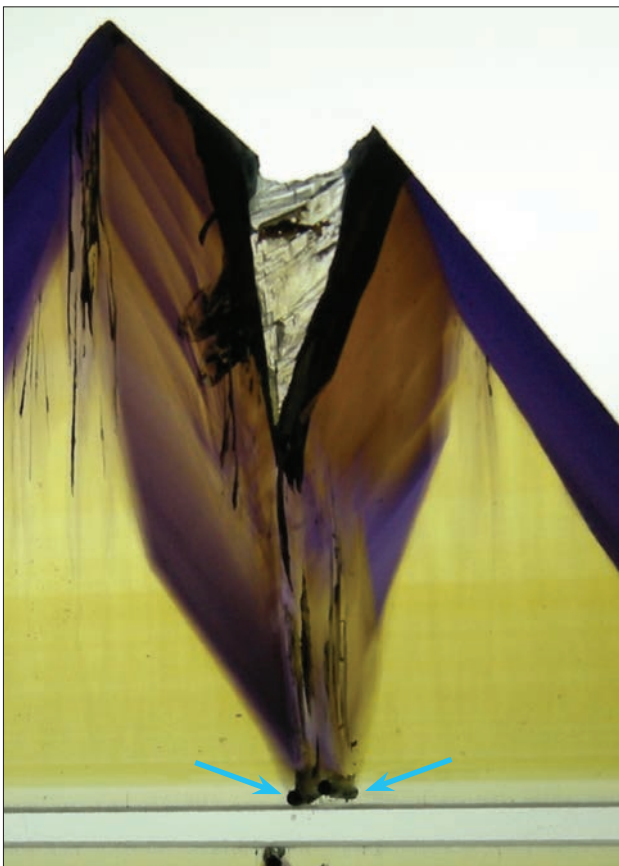
Figure 20: Growth of synthetic ametrine is also performed with Z-cut seed plates elongated parallel to the Y direction but with steel pins interrupting crystal growth. (Above, left) This drawing of a view parallel to the c-axis shows the orientation of the seed plate and the steel pins, as well as the position of the slice shown on the right. (Above, right) This slice of such a synthetic ametrine crystal was cut parallel to the Y direction (i.e. parallel to the long x prism faces); it measures 93 × 59 × 10 mm. The slice consists of two ametrine subindividuals with parallel orientation; steel pins are indicated with blue arrows. The colour distribution within basal c and rhombohedral r and z growth sectors can be seen; some boundaries between basal yellow growth sectors and adjacent violet-to-brown r growth zones are bent. Photo and drawing by K. Schmetzer.
