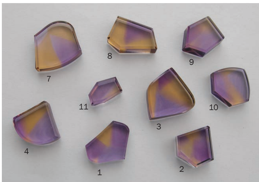
Figure 6: Slices of natural ametrine viewed parallel or almost parallel to the c -axis show variable colour distribution between violet r and yellow z growth sectors. In some of the samples, the r sectors include a range of hues from violet to purple. The samples weigh from 6.31 to 21.39 ct (sample 7, 20.3 × 19.5 × 5.4 mm). Photo by K. Schmetzer.
