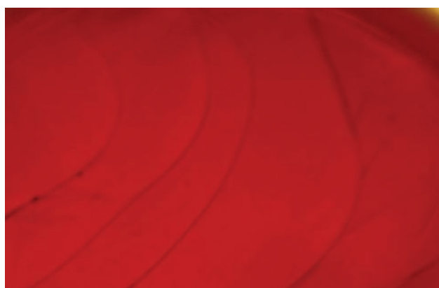
Figure 7: Red flow striations are seen within baked amber sample JF-1. Photomicrograph by Y. Wang; magnified 10×.
