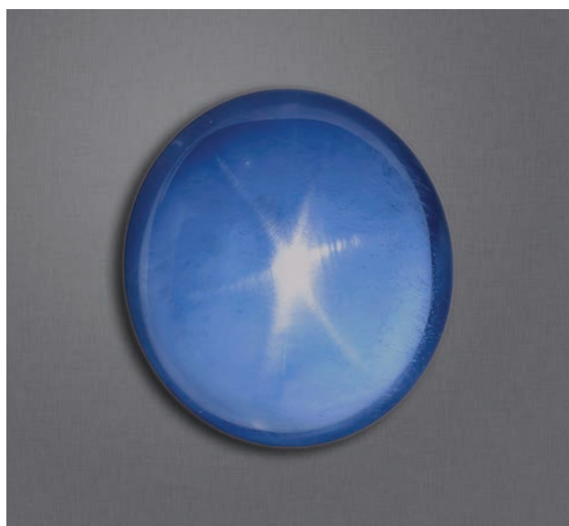
Figure 58: This 28.21 ct blue synthetic star spinel (18.6 × 17.5 × 9.3 mm) was sent to GIT's laboratory for an identification report. Photo by C. Onlaor.
