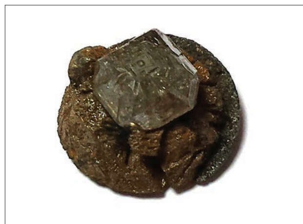
Figure 45: Typically, three crystals of synthetic diamonds (each less than 1 ct) are produced during each growth cycle, but single crystals up to 3 ct (as shown here) and occasionally up to 8 ct have been produced. Photo by J. C. Zwaan.
