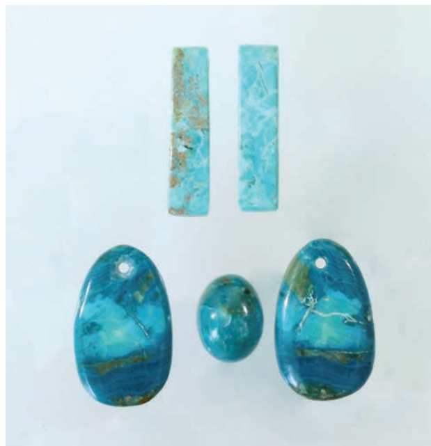
Figure 7: These polished samples consist of Apache Blue Stone that has been stabilized by polymer impregnation. The pieces on top (23.4 × 5.6 mm) were treated by the currently used stabilization method, while those on the bottom (drop shapes of 22.0 × 14.0 mm and an oval cut of 12.3 × 9.4 mm) were treated by an older polymer impregnation technique that partially darkened their colour. Photo by Dean Brennan.
