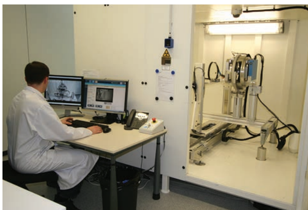
Figure 2: The X-ray phase contrast and darkfield imaging prototype EVITA, developed and installed at the CSEM research facility in Switzerland, was one of the instruments used in this study. Photo © V. Revol, CSEM Switzerland.
