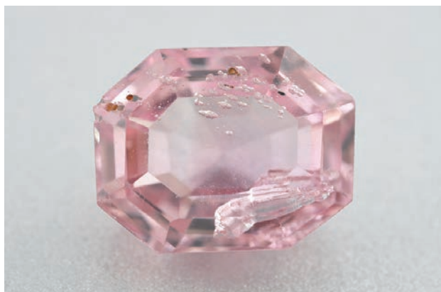
Figure 36: This 12.56 ct pink flame-fusion synthetic spinel coloured by iron is unusual for its large bent tubular inclusion (negative crystal/bubble), which is visible to the unaided eye in the lower right here. Also note the group of parallel ‘bomb-shaped’ gas bubbles in the upper portion of the gem, which are oriented in a different direction than the large inclusion. Photo by G. Choudhary.
