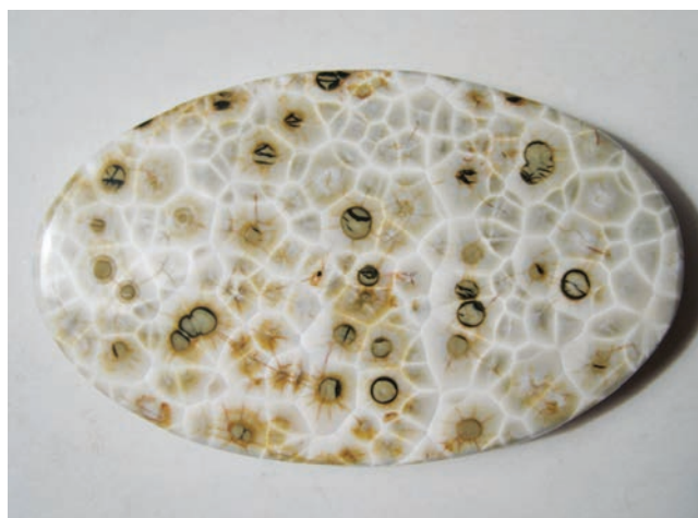
Figure 14: The cellular pattern in this natrolite cabochon is accentuated after it has been soaked in water for 10 seconds. In addition, its weight has increased from 229.21 to 231.85 ct. Photos by M. Campos Venuti.
