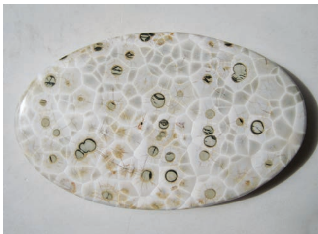
Figure 14: The cellular pattern in this natrolite cabochon is accentuated after it has been soaked in water for 10 seconds. In addition, its weight has increased from 229.21 to 231.85 ct. Photos by M. Campos Venuti.
