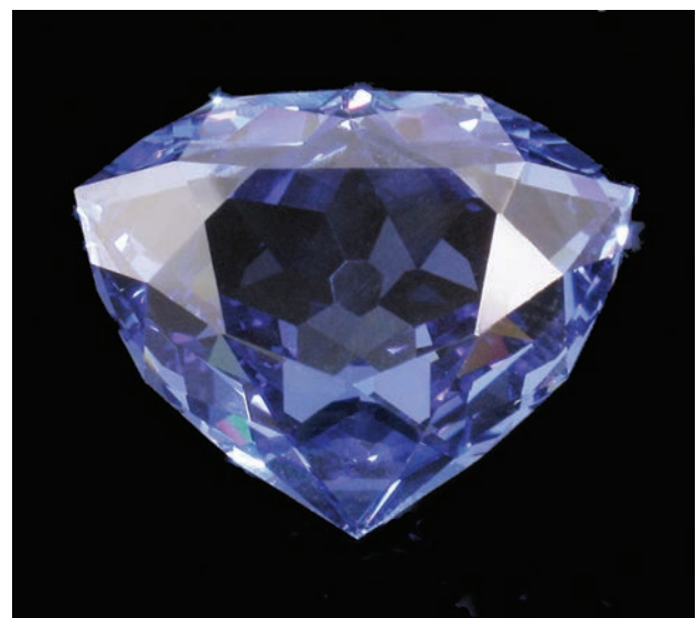
Figure 3: This CZ replica of the French Blue diamond was faceted by Scott Sucher (The Stonecutter, Tijeras, New Mexico, USA), and represents the stone as it was cut by Piton. Photo by Scott Sucher.
