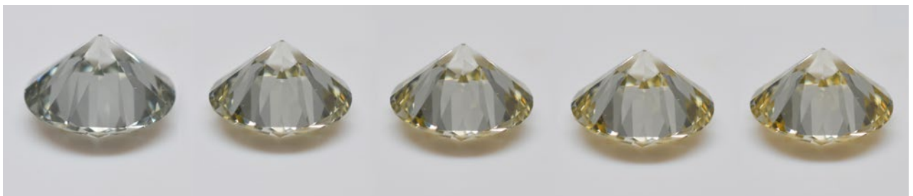
Figure 2: Viewed here table-down, the 25.85 ct chameleon diamond displays a progressive change in colour when heated from ambient conditions (left) to 160°C (right). Photos by A. Delaunay.
