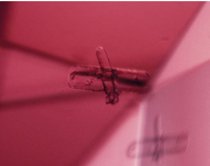
Figure 30: Colourless hexagonal prisms with the appearance of apatite also formed inclusions in the Mozambique spinels. Photomicrograph by Idan Shaulov; magnified 60x.
