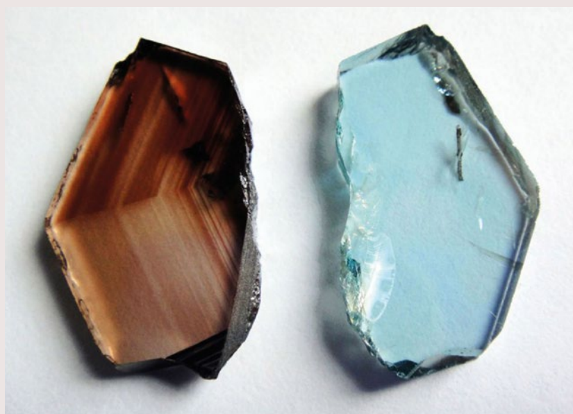
Figure 6: These two slices were cut from a gem-quality zircon crystal from Phnum Trom (largest dimension 17 mm). The samples were prepared as doubly polished plates (2.7 mm thick), and the half on the right was subjected to heat treatment whereas the one on the left remained in its initial state. The untreated specimen shows strong zoning, which disappeared after heat treatment. Photo by Astrid Wittwer.
