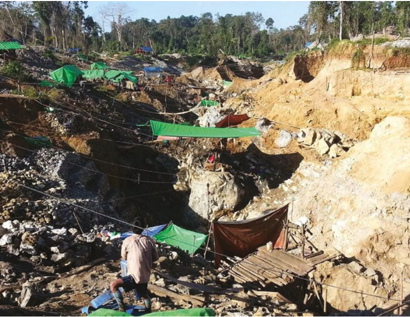
Figure 35: In the Khamti area, amber is mined from open pits (left) and from hand-dug shafts (right). Photo by Ben Sim.
