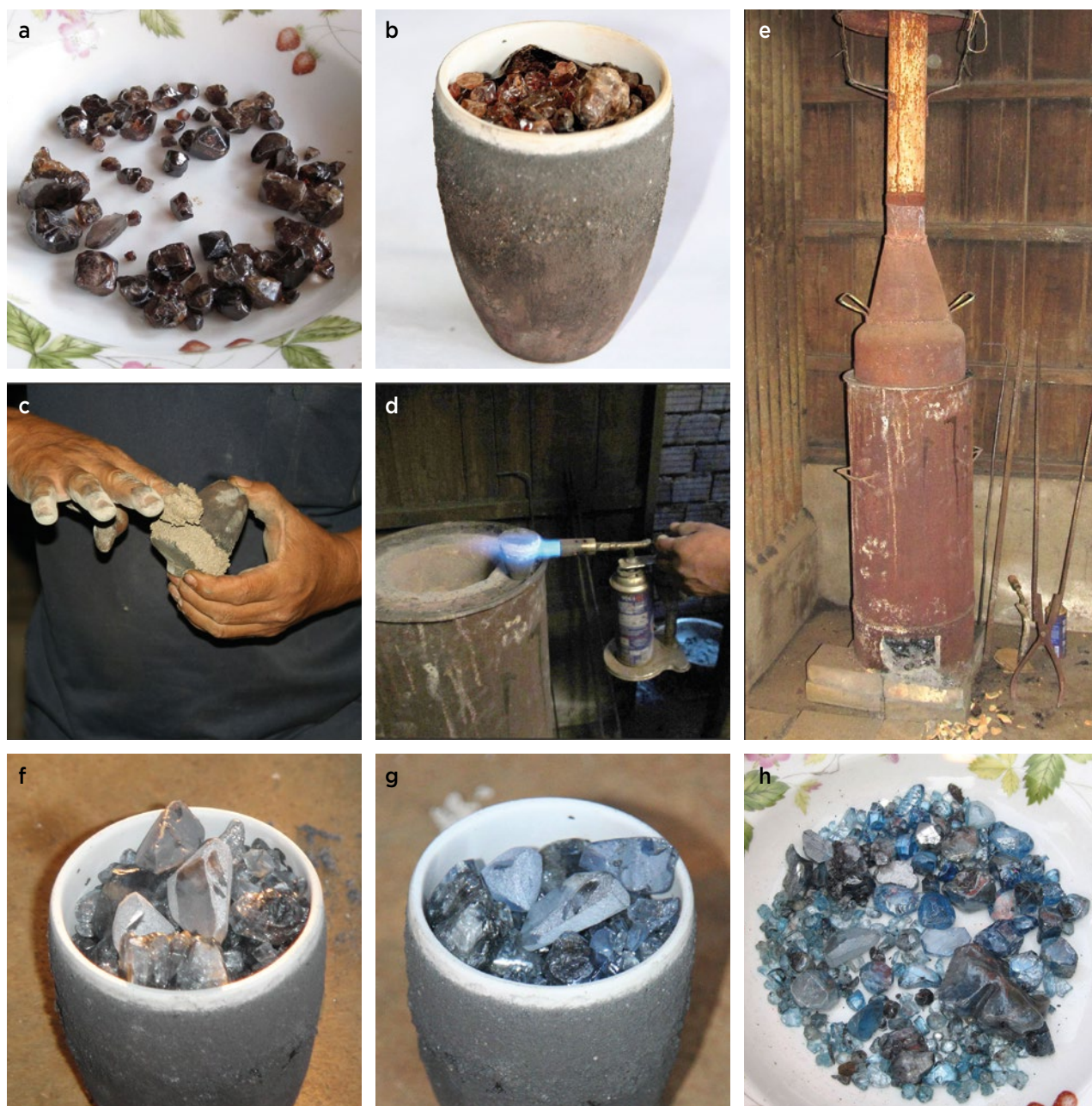
Figure 5: For the heat treatment of Ratanakiri zircon in a reducing environment, (a) the brown starting material is put into (b) an alumina crucible, and the lid is sealed with a refractory clayey material (c, d). Heat treatment at \sim 900\text{--}1,000^\circ\text{C} for 2–3 h is done in fairly simple ovens (e), with plenty of charcoal to ensure reducing conditions. After opening the crucible lid, the still-hot zircon material appears rather colourless (f), but becomes increasingly blue upon cooling (g). A good fraction of the heated zircon (h) shows the typical vivid blue colour. Photos by L. Nasdala (a, d, e, h), Ralf Grunert (b, c, g) and Astrid Wittwer (f).
