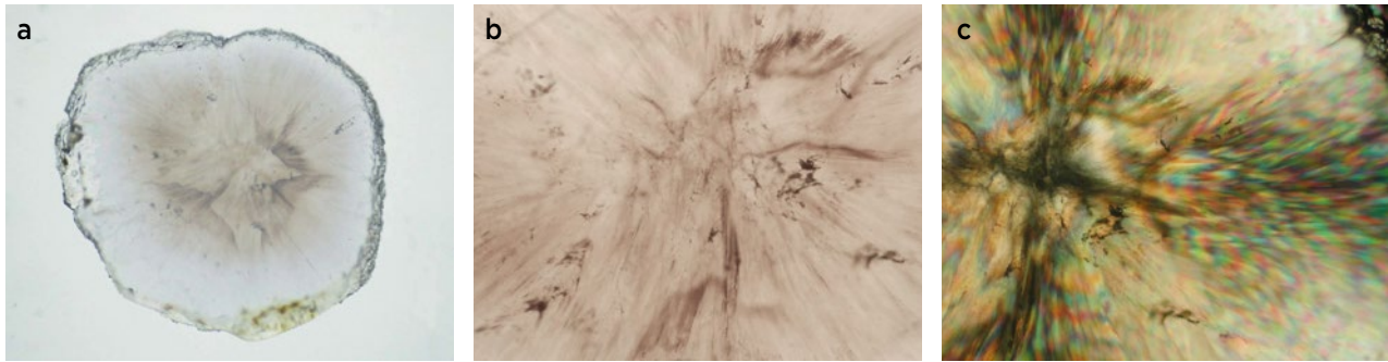
Figure 22: A thin slice (0.56 mm thick) of a 4.1-mm orb of Manakarra amethyst displays radial cracks and grain boundaries that are most visible toward its interior ( a, b ). In cross-polarised light, the radiating growth habit of the quartz is obvious ( c ). The individual quartz domains are generally about 20 \mu\text{m} wide. Photomicrographs by G. R. Rossman; image widths 1.97 mm (b and c).
