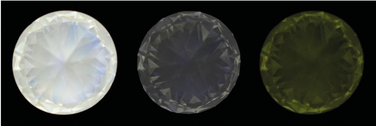
Figure 3: The 25.85 ct diamond luminesces intense chalky white to long-wave UV radiation (left) and weaker white to short-wave UV (centre). The unusual yellow phosphorescence (right) is characteristic of chameleon diamonds. Photos by A. Delaunay.
