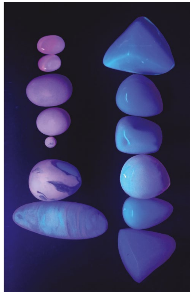
Figure 36: These 0.72–55.67 ct samples of Khamti amber (left) display variable fluorescence (right), consisting mostly of pink in the left column and blue-to-purple in the right column. The fluorescence is shown here under long-wave UV radiation. Photos by S.I Liu.
