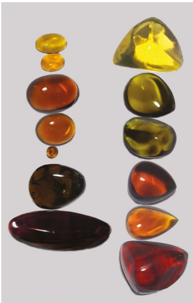
Figure 36: These 0.72–55.67 ct samples of Khamti amber (left) display variable fluorescence (right), consisting mostly of pink in the left column and blue-to-purple in the right column. The fluorescence is shown here under long-wave UV radiation. Photos by S.I Liu.
