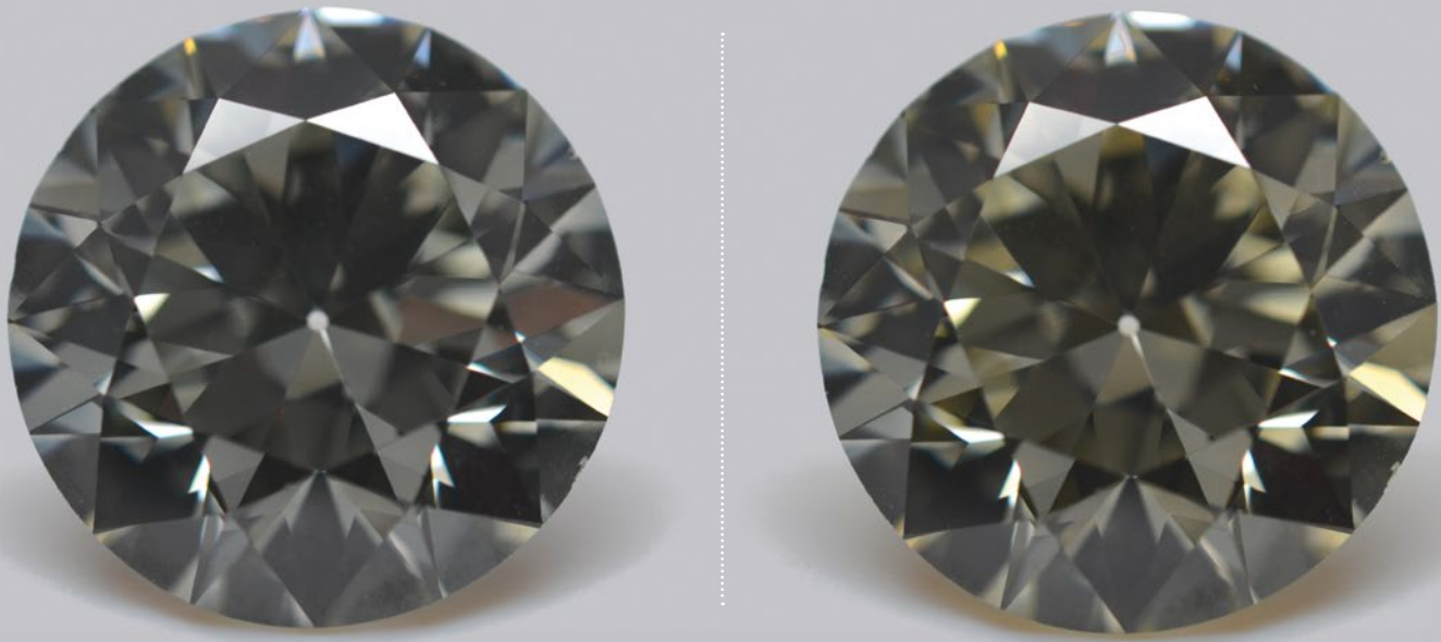
Figure 1: The 25.85 ct chameleon diamond studied by the authors is shown with its slightly greyish green 'stable' colour at room temperature (left) and its greyish yellow 'heated' colour (right). Photos by A. Delaunay.
