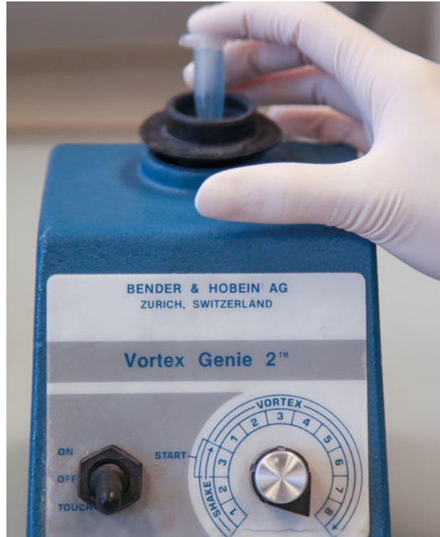
Figure 3: Vigorous vortexing of the nacre sample material in EDTA solution is necessary to detach the DNA molecules from the CaCO 3 framework. Photo by L. Cartier, SSEF.
