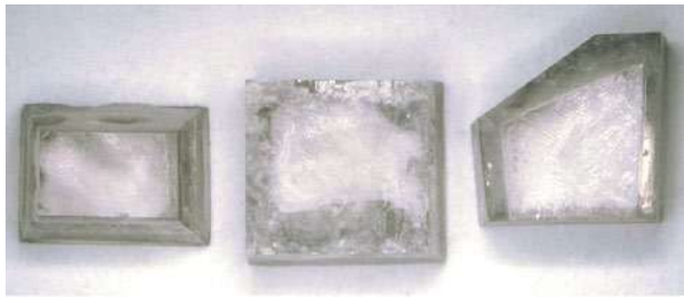
Figure 9: Three hybrid samples of CVD synthetic diamond overgrown on natural diamond were created for this study. The samples range from 3.4 to 3.6 mm wide and have CVD overgrowths of 0.92–1.09 mm thickness. Photo by X. Wu.
