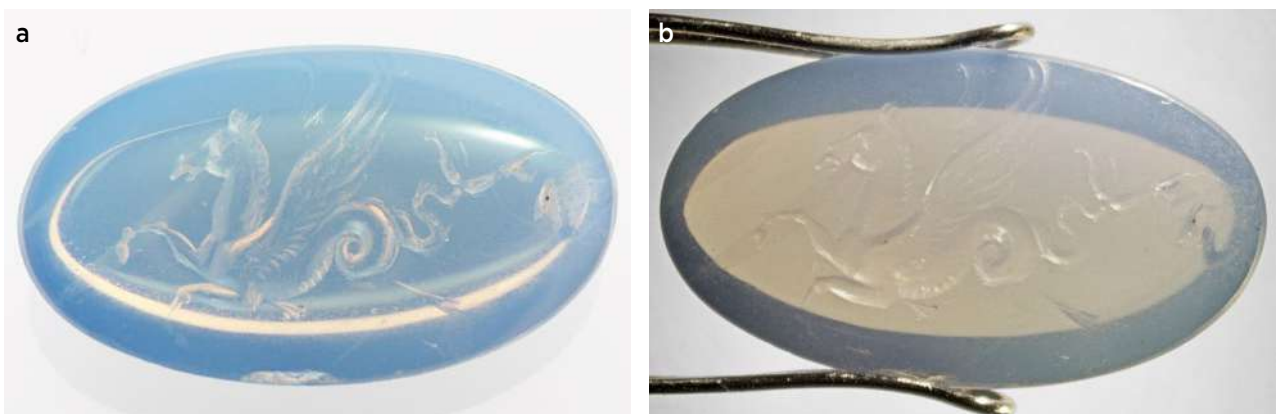
Figure 8: A comparison of the Roman intaglio in (a) reflected light and (b) transmitted light reveals the different colour appearances of the sapphire (bluish grey and greyish brown, respectively). Photos by M. S. Krzemnicki, SSEF.
