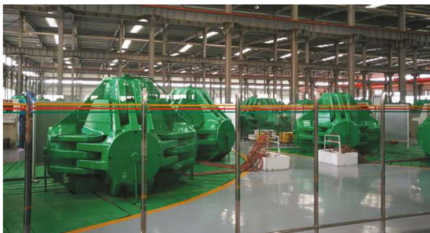
Figure 5: The factory of Zhengzhou Sino-Crystal Diamond in China’s Henan Province is a major producer of HPHT synthetic diamonds. This facility is scheduled to produce 7 Mct of gem-quality HPHT synthetic diamonds in 2020. Photo by T. Lu.
