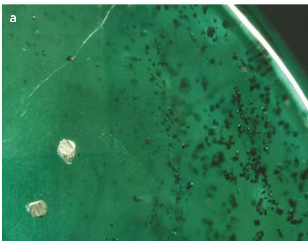
Figure 12: (a) Pyrite crystals and abundant chromite grains are prominent in this emerald, consistent with those from Santa Terezinha de Goiás in Brazil. (b) The chromite inclusions occur as both isolated grains and clusters in the emerald. Photomicrographs by R. Zellagui in darkfield illumination; magnified 9× (a) and 7× (b).
