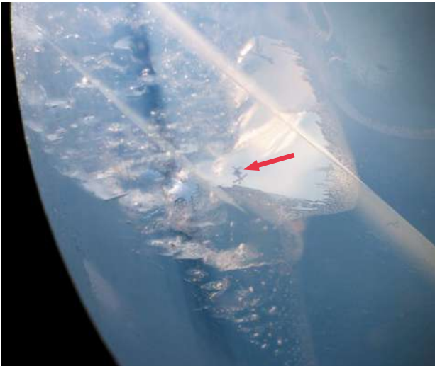
Figure 10: Magnification reveals twin planes and a healing fissure with dotted fluid inclusions in the Roman sapphire intaglio. The larger fluid inclusions show structured expansion discs. The main expansion disc contains tiny, radially arranged needles (see arrow) interpreted as Al-hydroxide precipitates. Photomicrograph by M. S. Krzemnicki, SSEF; image width 3 mm.
