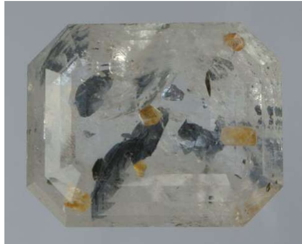
Figure 30: Inclusions of near-colourless to brownish yellow powellite occur together with dark grey molybdenite in this quartz from the Confianza mine. The stone weighs 62.33 ct and is 27 mm long. Photo by J. Hyršl.
