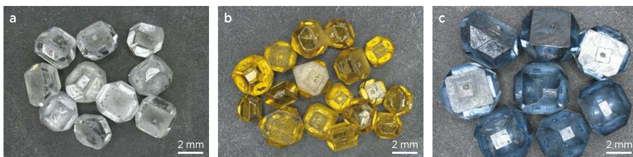
Figure 4: These crystals (0.40–0.80 ct) produced by Jinan ZhongWu New Materials are typical of Chinese HPHT synthetic diamonds that are (a) colourless, (b) yellow and (c) blue. Photo by T. Lu.
