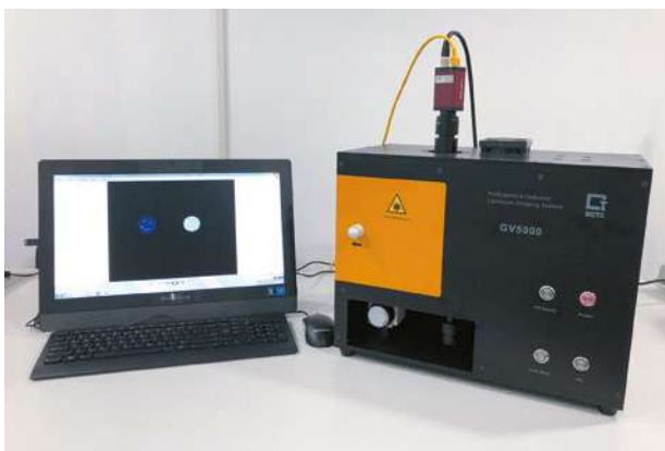
Figure 12: The GV5000 diamond-identification instrument was developed at NGTC. It uses fluorescence and phosphorescence imaging and spectral collection, decay-time measurements, and growth-pattern observations to distinguish HPHT and CVD synthetic diamonds from natural ones. Photo by H. Dai.
