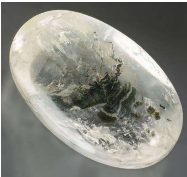
Figure 27: The dark green inclusions in this polished quartz (11.45 ct) were analysed for this report, and proved to be gormanite. Photo by Robison McMurtry, © GIA.
