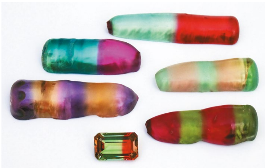
Figure 21: A 24.45 ct faceted synthetic corundum and five Verneuil half-boules (21.7–33.1 g) are representative of material now being produced by Thai Tech Sapphire Co. Ltd. Photo by L. Nasdala.
