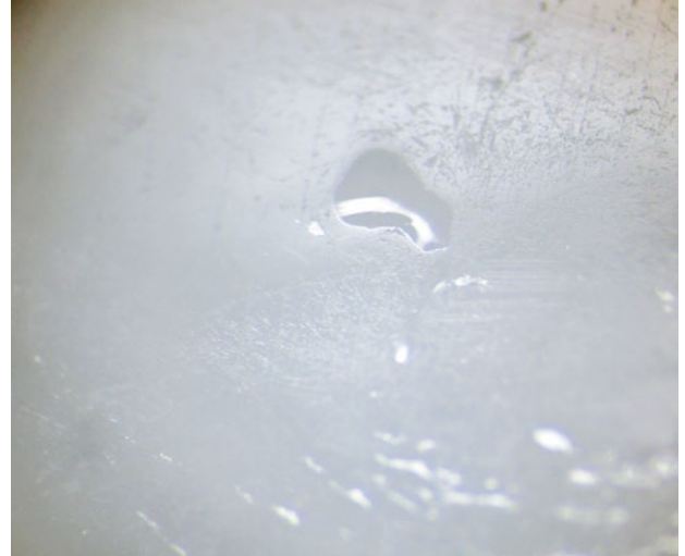
Figure 34: Depressions on the surface of the filled sapphire exhibit a glassy appearance. Photomicrograph by Dean Brennan, Stone Group Laboratories; magnified 30 \times .
