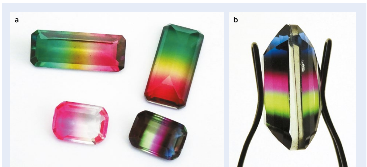
Figure 23: (a) Four faceted glass doublets (6.4–14.9 ct) represent another multicoloured material that has recently appeared on the Thai gem market. (b) Even without immersion it can be seen that the pavilion and crown of this 6.7 ct doublet are colourless; the apparent colouration is caused by the central resin layer. The small colourless spot in the upper right of this sample (only visible from the side) is caused by insufficient contact between the pavilion and the resin layer. Photos by L. Nasdala.
