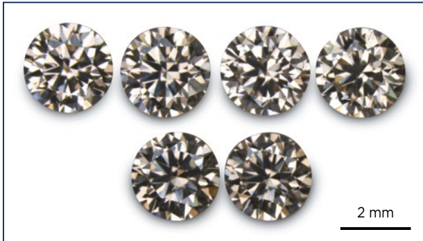
Figure 17: These six 2.5-mm-diameter CVD synthetic diamonds were found in a parcel of more than 1,000 light brown diamonds. Photo by T. Hainschwang.
