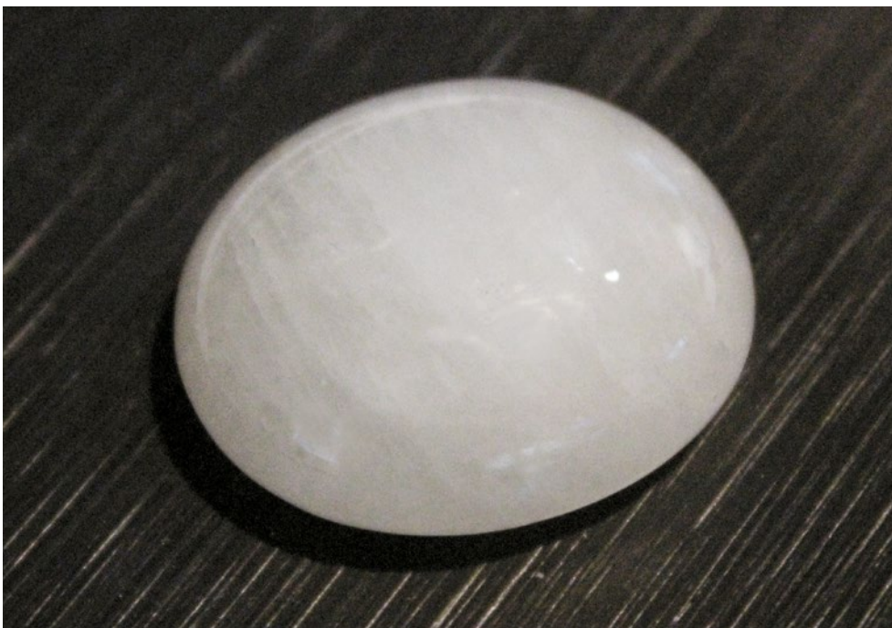
Figure 31: This 62.59 ct white sapphire proved to be filled with lead glass. Photo by B. Williams.
