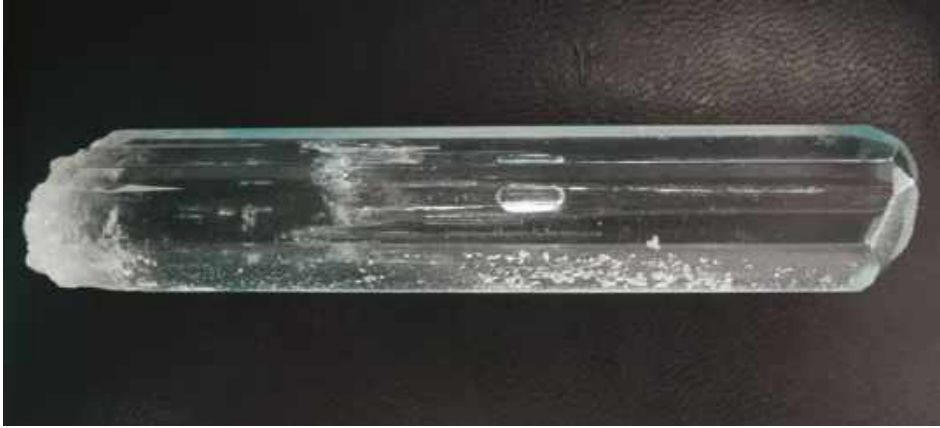
Figure 4: This aquamarine crystal contains an elongate growth channel oriented parallel to the c -axis that has a movable gas bubble (here, positioned about halfway along its length). The crystal measures approximately 89 × 17 mm, and the growth channel is about 56 mm long and 3 mm wide. Photo by B. M. Laurs.
