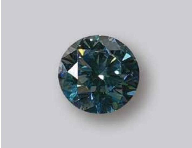
Figure 1: The two type IIa blue CVD synthetic diamonds (1.76 ct loose and 2.63 ct mounted) examined for this study owe their colour to irradiation treatment. Photos by Z. Song.
