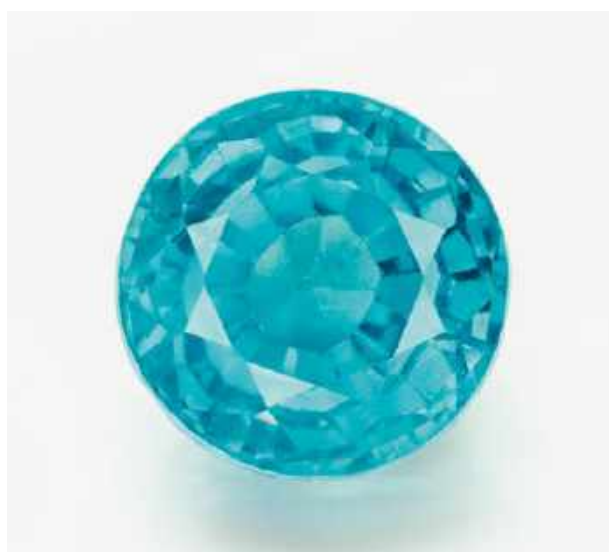
Figure 36: This 3.73 ct melt-grown synthetic sapphire has an unusual colour, which more closely resembles that of Paraíba-type tourmaline, apatite or zircon than a variety of natural corundum. Photo by Alex Mercado and Bilal Mahmood, AGL.
