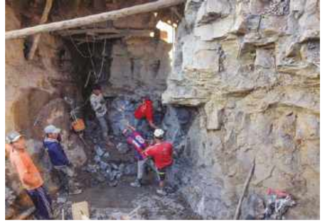
Figure 7: A pulley system (see ropes and orange bucket) is being used to remove amber-bearing limestone from this adit at Lachun Maw. The mining crew then breaks open the pieces of limestone in search of amber. Photo by Thet Tin Nyunt.
