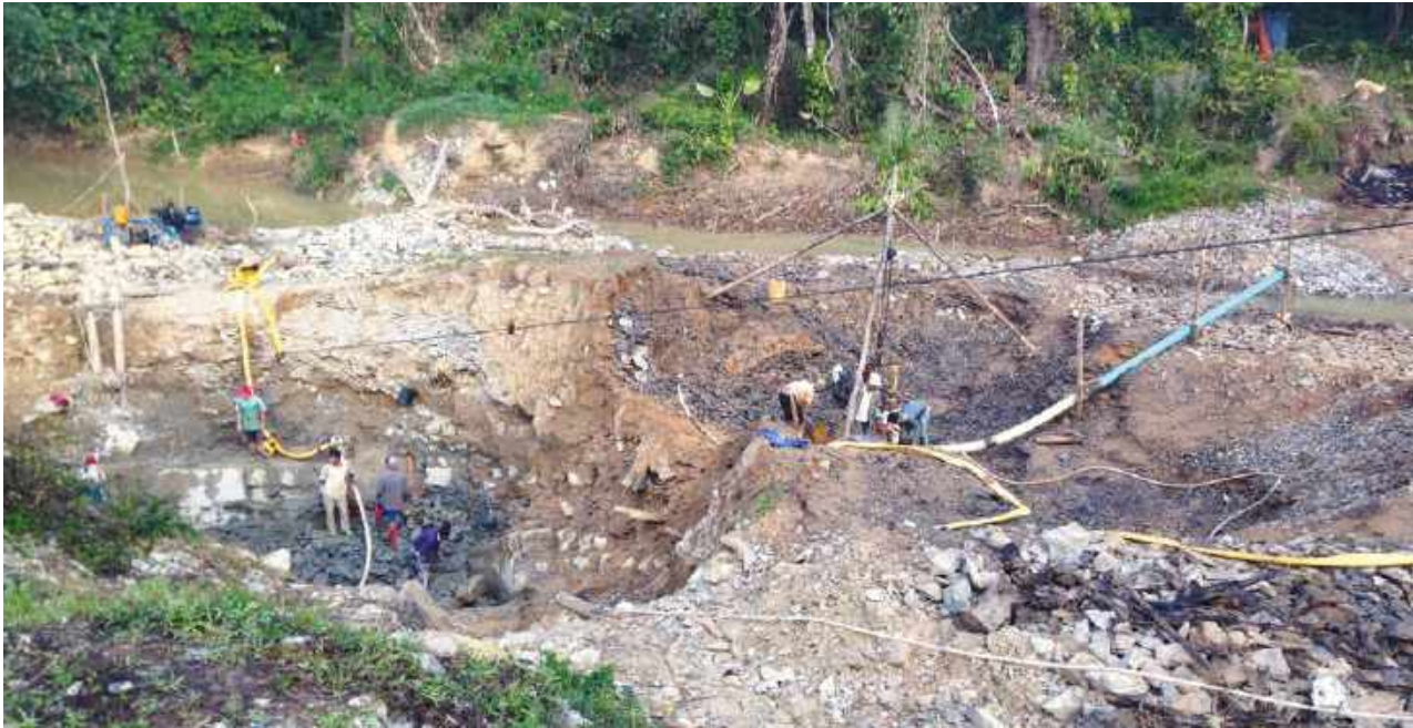
Figure 9: Open-pit mining for amber sometimes takes place, as shown here at Kyat Maw. The miners must use pumps to keep the pits from flooding with water. Amber from this mine tends to be dark brown, brown and yellow. Photos by Thet Tin Nyunt.
