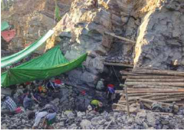
Figure 6: This view of Lachun Maw shows the entrance of an adit that explores the amber-bearing limestone at a shallow angle along bedding planes. Photo by Thet Tin Nyunt.
