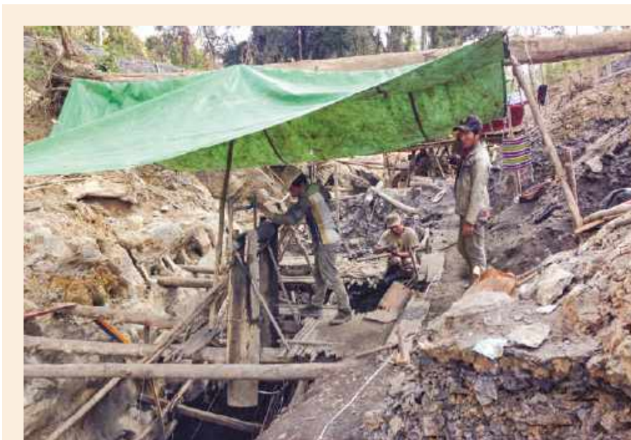
Figure 8: Vertical shafts are also used to reach the amber-bearing limestone, as shown here at Kyat Maw. This shaft is more than 5 m deep. Photo by Thet Tin Nyunt.
