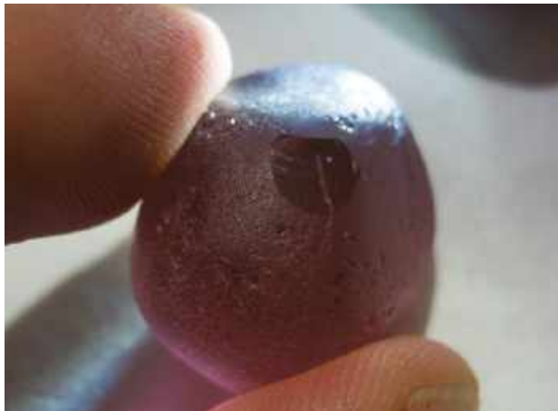
Figure 35: Weighing 26.18 g, this gem ‘pebble’ was offered as a garnet in Arusha, Tanzania, and proved to consist of manufactured glass. Note the tiny gas bubble visible on the upper right side of the polished window. Photo by B. M. Laurs.
