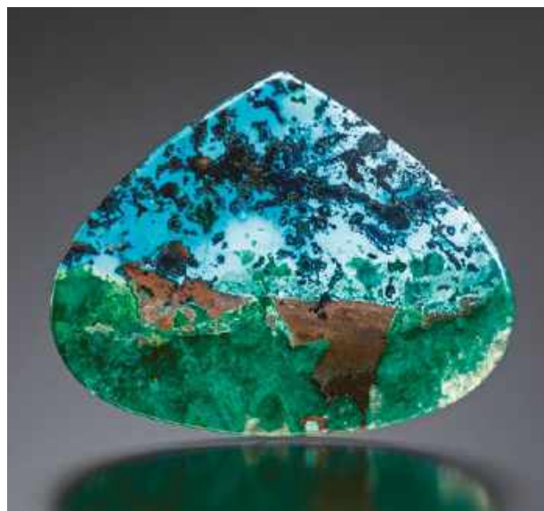
Figure 34: This colourful doublet (58.2 × 45.1 × 4.7 mm) consists of an assemblage of diopside (green), chrysocolla (light to medium blue) and shattuckite (dark blue), which has been affixed to a durable backing material. Photo by Jeff Scovil.
