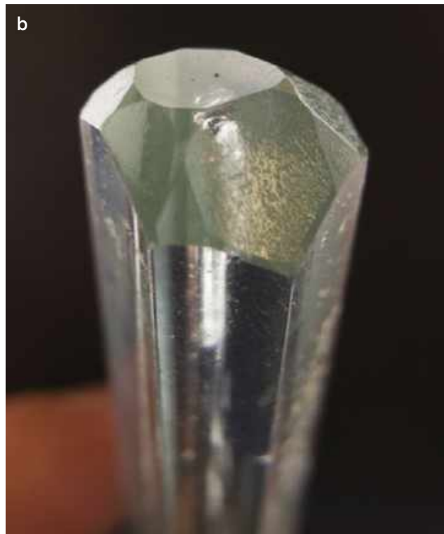
Figure 5: (a) The growth channel hosting the bubble ends within about 2 mm of the aquamarine crystal’s termination. (b) In reflected light, a tiny dimple is visible as a dark spot on the flat termination of the crystal, and is located adjacent to where the growth channel ends. Photos by B. M. Laurs.
