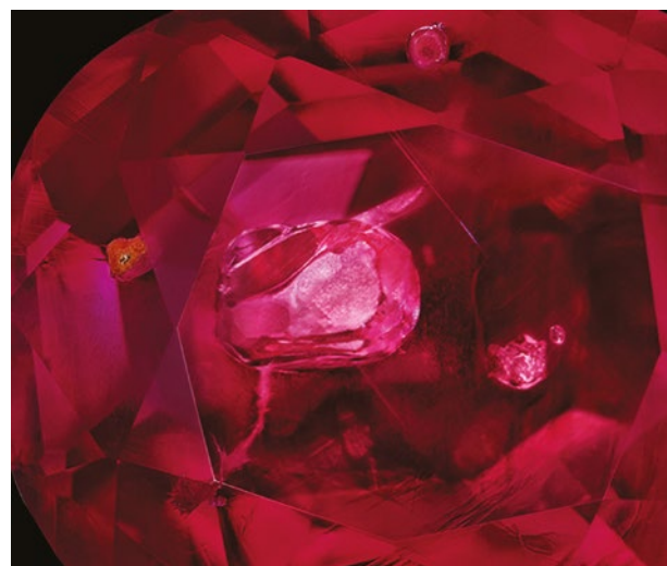
Figure 6: Shown here is a particularly large near-colourless apatite crystal located just under the table facet of the 1.39 ct Burmese ruby. Photomicrograph by C. P. Smith; magnified 28 \times .
