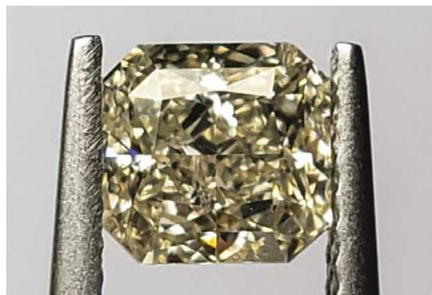
Figure 11: This 1.29 ct pale yellow type IIa diamond owes its colour to H4 centres. Photo by W. Zhu.
