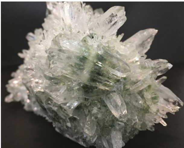
Figure 20: This group of crystals (160 mm long) on one side of the synthetic quartz cluster displays conspicuous colour banding perpendicular to the direction of crystal growth. Photo by H. Dai.
