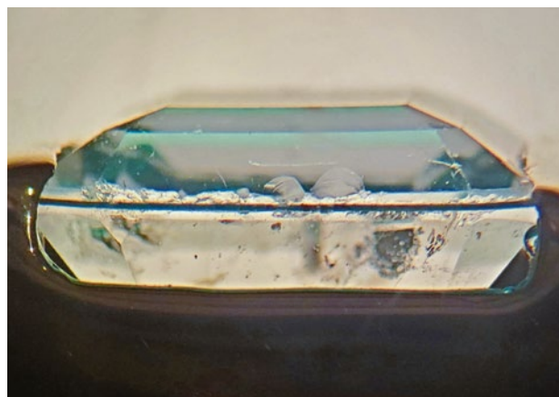
Figure 17: A side view of the girdle of the triplet clearly reveals a coloured intermediate layer. Photo by B. Williams, using darkfield illumination and immersed in water.
