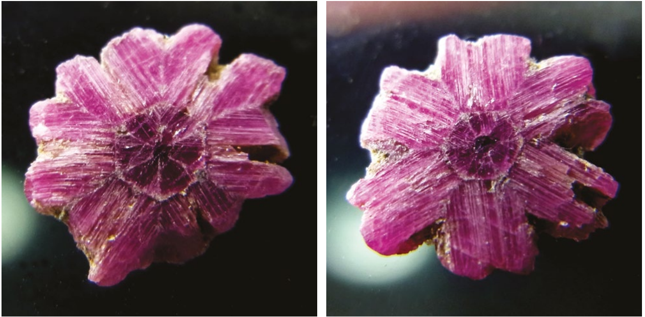
Figure 1: Two flower-shaped trapiche rubies (each slice is about 5–7 mm diameter and 1.0–1.5 mm thick) from Mong Hsu were analysed for this study: samples FS02 (left) and FS03 (right). Photos reproduced from Liu (2015).
