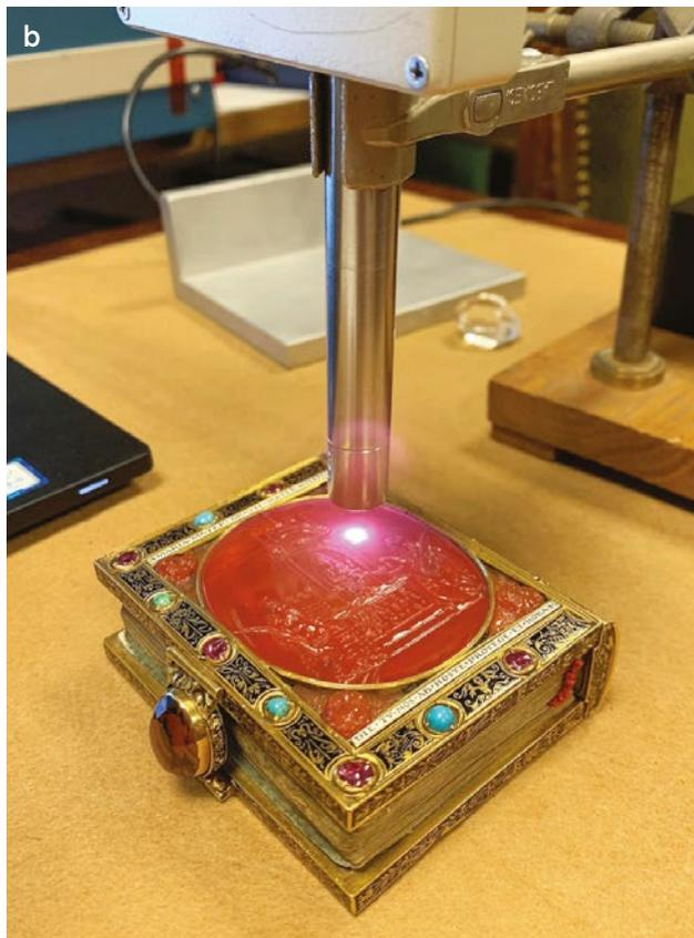
**Figure 6:** Portable instruments used for the gemmological examination of the Book of Hours included (a) a refractometer and (b) a Raman spectrometer with a 785 nm red laser. Photos by G. Panczer.
