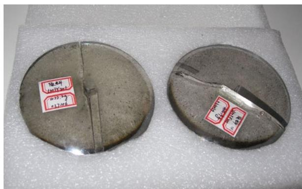
**Figure 22:** These two bulk-crystal plates of silicon carbide were photographed at SICC Materials Co. Ltd in Jinan, China. They are representative of some of the damaged silicon carbide material used to facet synthetic moissanite gems. The plate on the left weighs 422.2 g and the one on the right is 405.9 g. Photo by Jianjun Li.
