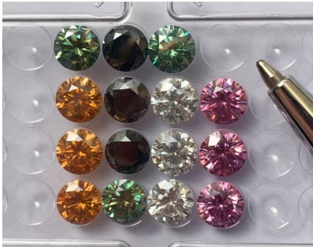
**Figure 23:** Round brilliants cut from synthetic moissanite such as these with a diameter of about 6.5 mm are roughly the size of a 1 ct diamond. The black and green colours are as grown, while near-colourless gems are produced by annealing brown material, and pink and brownish orange colours are due to surface coatings. Photo by Jianjun Li.
