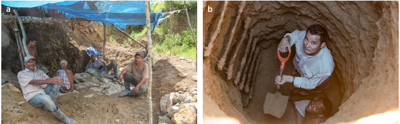
Figure 4: Most amber mining in the Dominican Republic takes place in underground workings. (a) Local miners rest near a typical shaft that is more than 10 m deep. (b) One of the authors (GS) joins a local miner at the bottom of a shaft. Photos by Guanghai Shi (a) and Yongqiao Wu (b).
