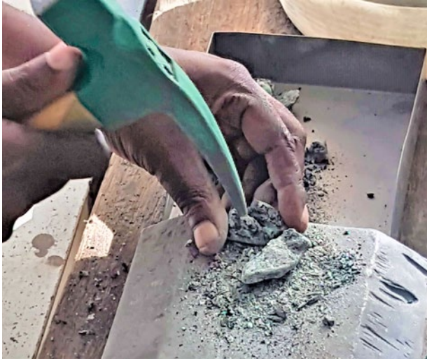
Figure 7: Conventional hand cobbing is accomplished using a hammer in order to recover emeralds from micaceous schist. Photo by V. Rudashevsky and O. Alikin.
