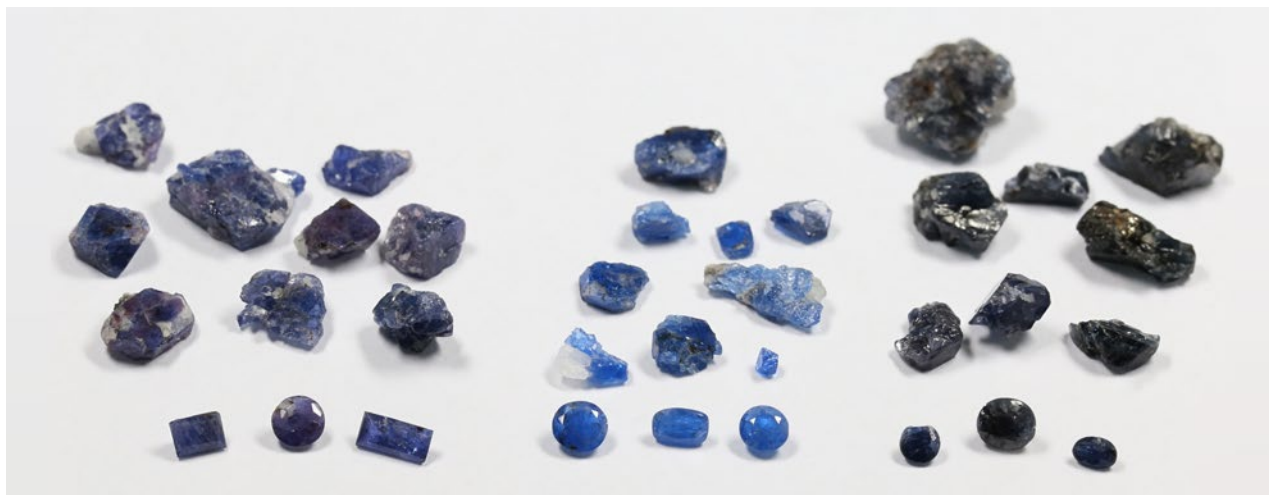
Figure 4: The spinel study samples were separated into the three colour groups: violet-blue (left), bright blue (centre) and dark blue (right). The faceted stones weigh 0.19–0.79 ct. Photo by K. Schollenbruch.
