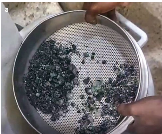
Figure 8: Disaggregated material that passed through the 16 mm sieve during EPD processing is then wet-screened using a 2.8 mm sieve (a) to remove waste silt (b). Photos by V. Rudashevsky and O. Alikin.
