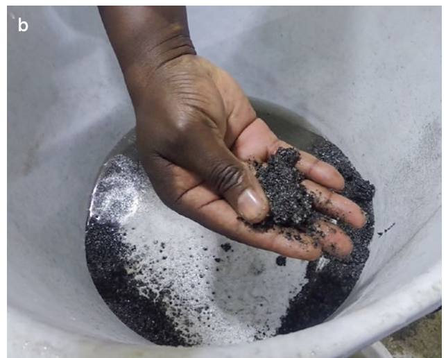
Figure 8: Disaggregated material that passed through the 16 mm sieve during EPD processing is then wet-screened using a 2.8 mm sieve (a) to remove waste silt (b). Photos by V. Rudashevsky and O. Alikin.
