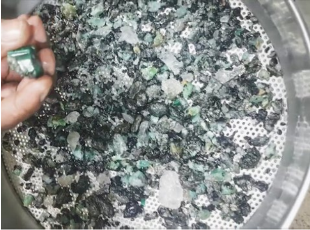
Figure 9: Emeralds are hand-picked from the disaggregated material after EPD processing, including some relatively large crystals. Photo by V. Rudashevsky and O. Alikin.
