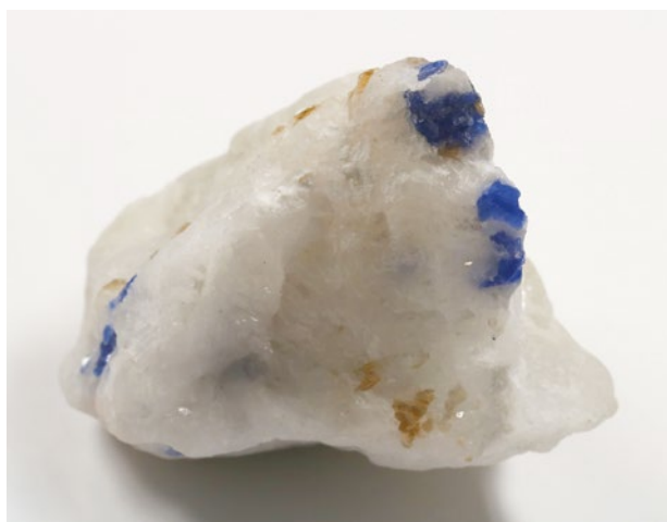
Figure 5: This matrix specimen (approximately 6.3 cm wide) consists mainly of coarse calcite marble that contains several bright blue spinel fragments. Smaller brown phlogopite crystals are also seen in this view. Photo by K. Schollenbruch.
