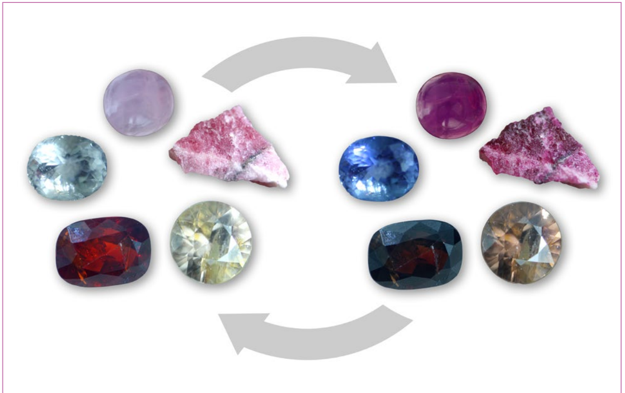
Figure 1: Some remarkable photochromic gems are shown in this composite image before (left) and after (right) exposure to UV radiation. Clockwise from top: sodalite (hackmanite; 0.48 ct), tugtupite (1.10 g), near-colourless zircon (0.43 ct), red zircon (21.3 ct) and marialite (0.91 ct). Photos by Thomas Hainschwang and Féodor Blumentritt.
