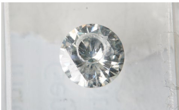
Figure 27: A hole was drilled through sealed plastic packaging to allow access for the tip of a diamond tester to the table of this round brilliant (6.53 mm in diameter overall). However, electrical conductivity cannot be measured without metal contact, so distinction between diamond and synthetic moissanite is not possible using only a diamond tester while a sample is enclosed in such packaging. Although this sample was accompanied by a report indicating it is diamond, further testing showed it to be synthetic moissanite. Photo by U. Henn.
