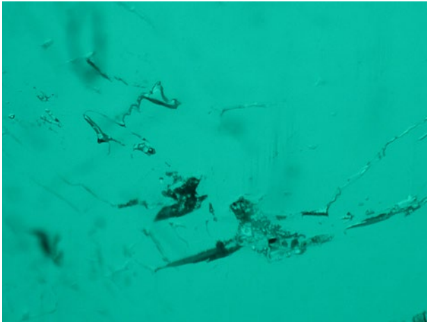
Figure 13: Spiky multiphase fluid inclusions are seen in an emerald from Musakashi, Zambia. Photomicrograph by M. S. Krzemnicki, © SSEF; magnified 50 \times .
