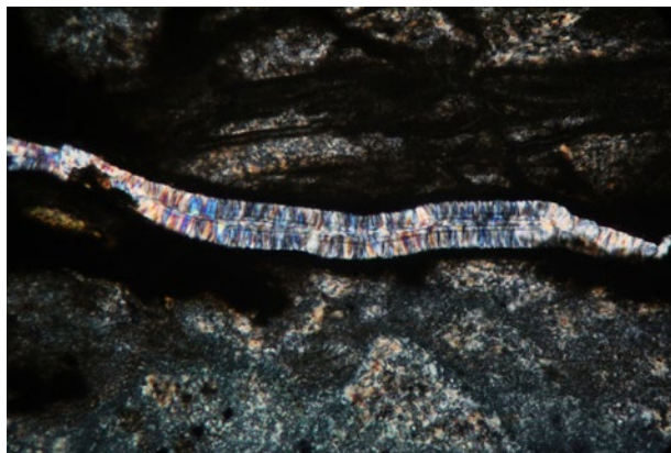
Figure 10: Viewed in cross-polarised light, this image of a thin section of Baluchistan chrysoprase shows a veinlet of crystalline quartz, as well as radial aggregates of quartz (at the bottom of the photo). Photomicrograph by P. Hadipanah; magnified 40×.
