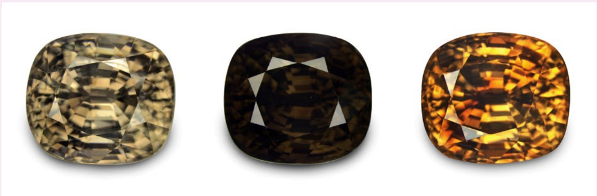
Figure 12: This 62 ct light brown photochromic zircon of unknown locality (left) shows an impressive change, becoming dark brown after exposure to long-wave UV radiation (centre). It returned to lighter brown with exposure to visible light. Interestingly, after heating at about 400°C it became bright yellow-orange (right), but that colour was not stable. Photos courtesy of Thomas Hainschwang.
