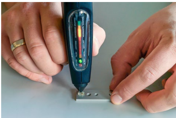
Figure 26: Use of a diamond tester that measures both thermal and electrical conductivity yields the best results for separating synthetic moissanite from diamond, but testing for electrical conductivity requires that the sample be placed in contact with metal. Photo by U. Henn.
