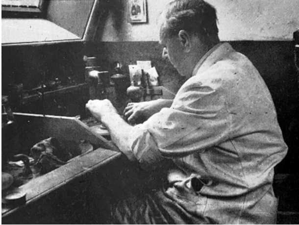
Figure 10: George Bull-Diamond, manager of Chas. Mathews (Lapidaries) Ltd from the 1940s to the 1980s, is shown cutting a stone on a jamb-peg bench in this illustration from Webster's Gems (1975, p. 434). Reproduced with permission.
