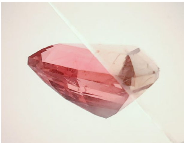
Figure 11: Strong pleochroism from pink to pale pinkish orange is shown by euclase sample 2, which weighs 2.99 ct. Photo by C. Williams.
