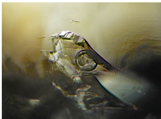
Figure 22: Negative crystals in Madagascar demantoid are mostly empty, but occasionally contain water (liquid and vapour), as seen in this example. Image width 0.9 mm.
