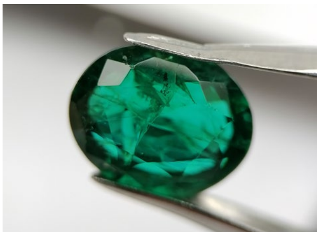
Figure 31: This 4.05 ct faceted green specimen submitted to EGL South Africa's laboratory turned out to be a glass simulant of emerald. Photo by K. Khourie.
