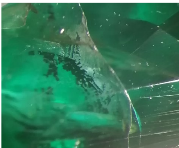
Figure 32: White residues within a surface-reaching fissure in the glass simulant indicate the presence of an oil or resin filling, which suggests a conscious attempt at fraud. Photomicrograph by K. Khourie; magnified 70×.
