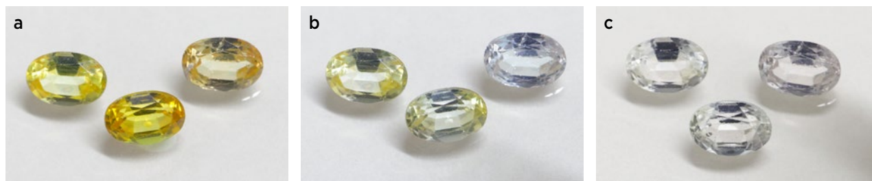
Figure 11: Three initially near-colourless sapphires (2.46–2.60 ct) gain (a) an orangey yellow colour after exposure to X-rays, (b) which fades dramatically after illumination for a few minutes by intense visible light from a 100 W halogen fibre-optic lamp. (c) All colour completely disappears after slightly heating the samples above the flame of a cigarette lighter. These three sapphires did not change colour following exposure to UV radiation. Photos by F. Blumentritt.
