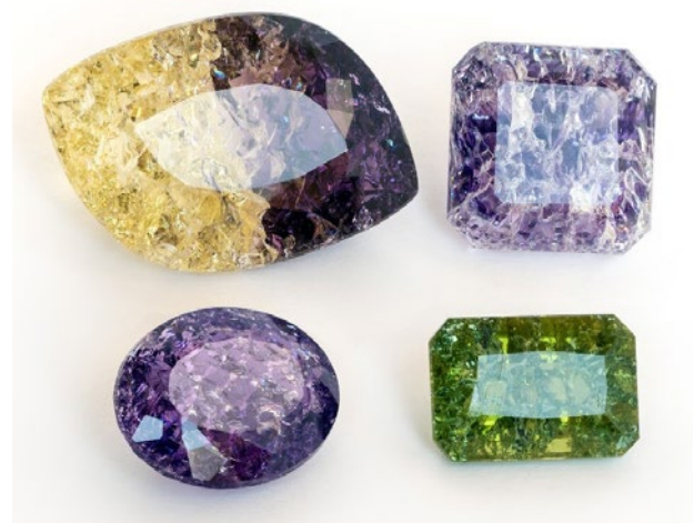
Figure 40: These four faceted samples (9.6–32.6 ct) of quench-fractured monochrome or bicoloured synthetic quartz illustrate some of the colour variations available. Composite photo by M. Wildner.
