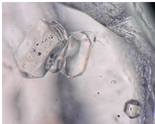
Figure 10: Transparent colourless, well-formed, hexagonal-prismatic, doubly terminated apatite crystals of variable size are oriented in different directions and show low relief in the host Tajik spinel. Magnified 200 \times .
