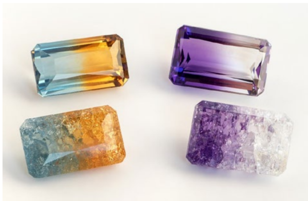
Figure 37: These two pairs of bicoloured synthetic quartz (14.8–23.5 ct) demonstrate the appearance of this material before (top row) and after (bottom row) intentional fracturing. Composite photo by M. Wildner.
