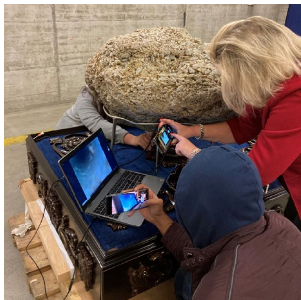
Figure 23: Endoscopic examination of a hole drilled into the aggregate reveals that the sapphire crystals extend all the way to the centre of the specimen. Photo by L. Kiefert.
