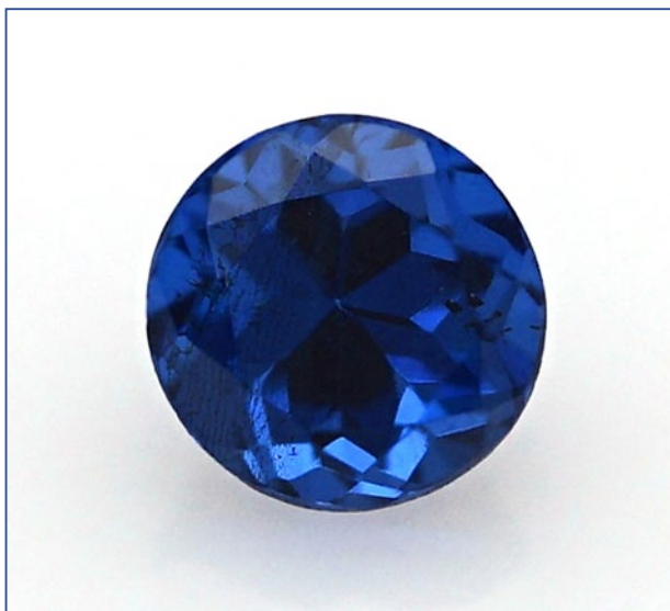
Figure 2: This 0.47 ct flux-grown synthetic spinel is coloured by cobalt. Photo by T. Stephan.
