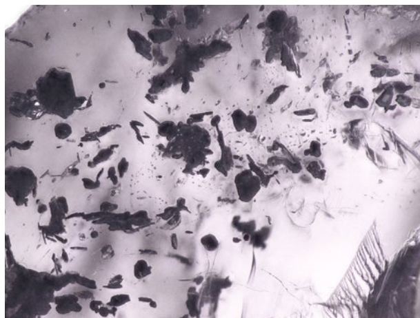
Figure 7: Graphite (which derives from the metamorphism of organic substances in the spinel host rock) is a frequent inclusion in Tajik spinel. It is present both as opaque black, mostly plate-like crystals (as shown here) and as a filling material in primary and (pseudo-)secondary cavities and fluid inclusions. Magnified 150×.
