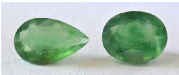
Figure 14: These green opals (1.26 ct pear and 1.76 ct oval), reportedly from Peru, were studied for this report and proved to be coloured mainly by Cr 3+ . Photo by K. Feral.
