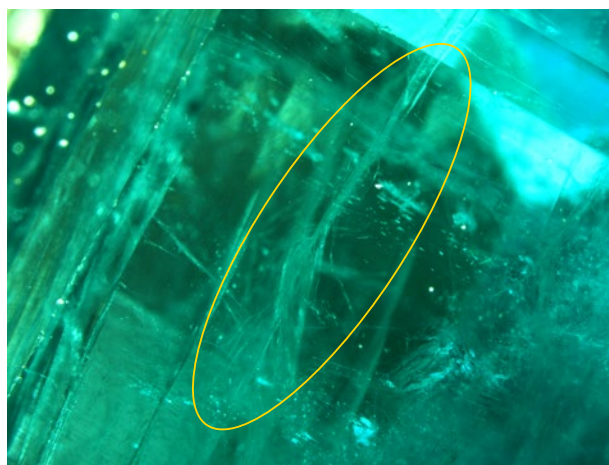
Figure 2: One of the fissures in the emerald in Figure 1 is seen here in darkfield illumination with the gemmological microscope. Photomicrograph by Christopher P. Smith; magnified 30×.
