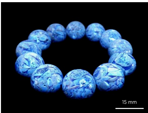
Figure 13: Long-wave UV fluorescence of the beads is unevenly blue, and they appear to consist of blocky pieces cemented together with a bonding material. Photo by Yu-Shan Chou.
