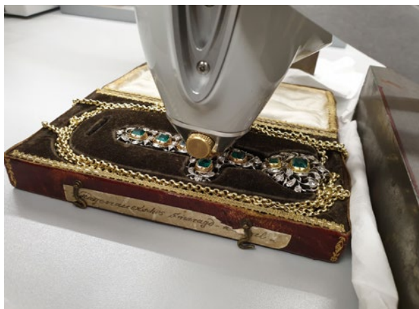
Figure 9: In 2020, the emerald pectoral cross (shown here) and ring were also analysed with a portable X-ray fluorescence unit. Photo by H. A. Gilg.
