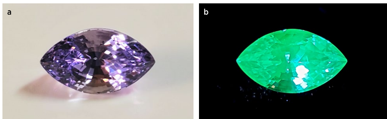
Figure 6: (a) This 'lilac' spinel from Sri Lanka weighs 3.73 ct and measures 12.64 × 7.22 × 6.52 mm. (b) Viewed under long-wave (369 nm LED) UV radiation, the spinel emits an unusual strong bluish green luminescence. Photos by C. Williams.
