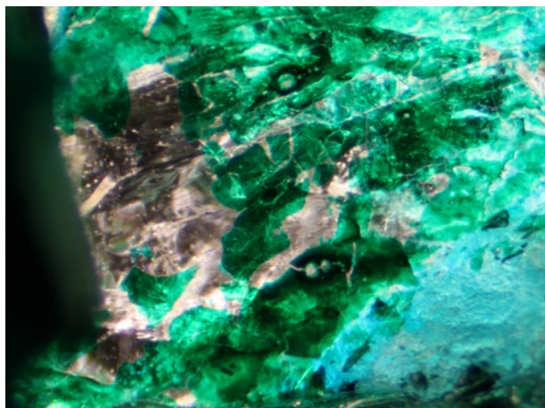
Figure 23: Viewed with a microscope, the internal surface of the cavity in Figure 22 shows an amorphous material with gas bubbles, which proved to be glass. The green colour of the glass was restricted to its surface. Also visible are areas of greenish blue glue (seen mostly on the lower right). Photo-micrograph in transmitted light by J. Štubňa; magnified 7.5×.
