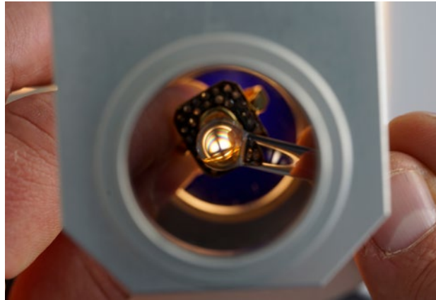
Figure 27: The conoscope reveals the centre stone in the ring to be optically uniaxial, consistent with the authors’ identification of it as synthetic moissanite. Photo by T. Stephan.
