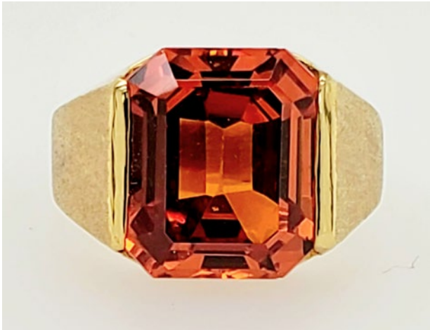
Figure 15: This orange gem (approximately 14 × 12 mm) set in a custom-made mounting was identified as a BaZrO 3 -type ceramic material. Photo by B. Williams.
