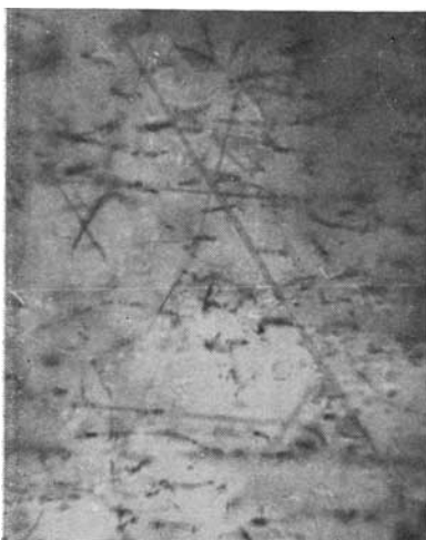
FIG. 5. Fine channels in blue Apatite cat's-eye.
