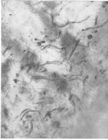
Small twisted veil-like feathers and general turbidity in a synthetic emerald made by Prof. Nacken.
